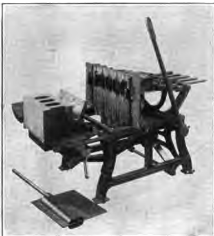
Fig. 71. Hobbs Face-Down, Wet-Process Concrete Block Machine Courtesy of Hobbs Concrete Machinery Company, Detroit, Michigan
