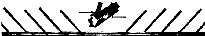
Fig. 9. Kahn Trussed Bar for Reinforcement of Concrete Courtesy of The Kahn System
