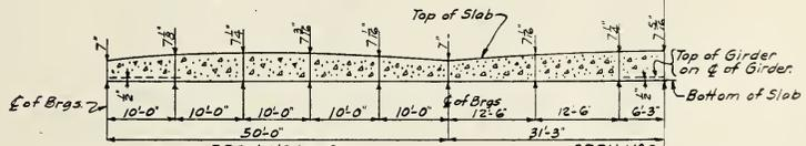
**SLAB THICKENING DIAGRAM FOR DEAD LOAD DEFLECTION**
