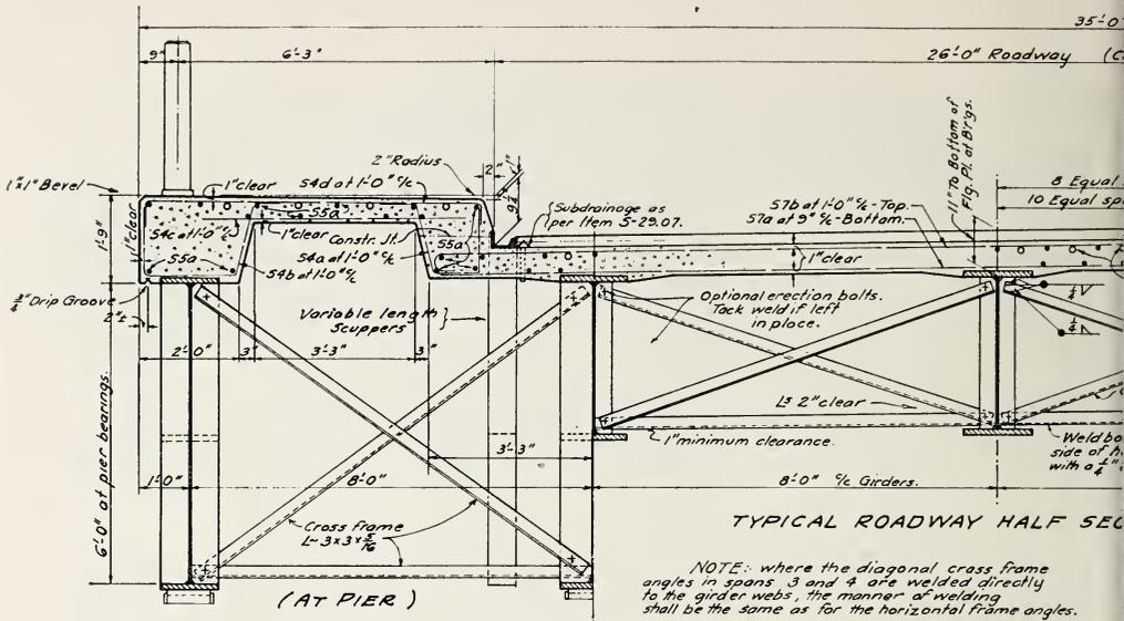
NOTE: where the diagonal cross frame angles in spans 3 and 4 are welded directly to the girder webs, the manner of welding shall be the same as for the horizontal frame angles.
