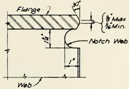
Note: Ends of girders to be welded shall be prepared in the shop and each splice checked by assembling the two beam sections to be spliced and the pieces matchmarked
