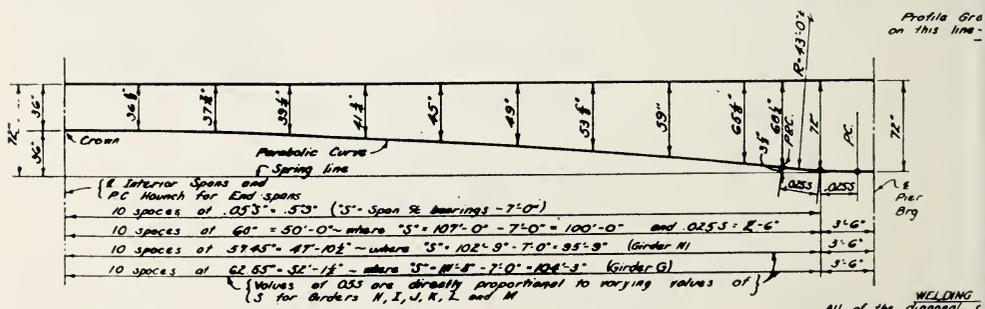
TEMPLATE FOR PARABOLIC HAUNCH FOR WEB PLATES
