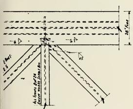
PLAN OF LATERAL BRACING (TYP.)
