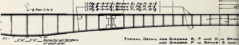
TYPICAL DETAIL FOR GIRDERS B, F AND D IN SPANS 3 AND 5
