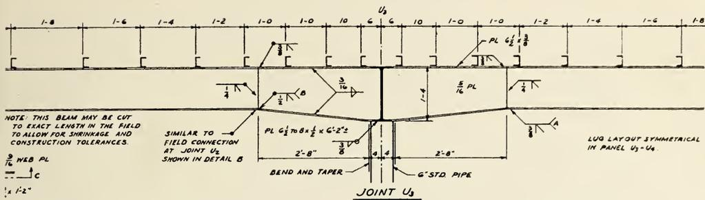
NOTE: THIS BEAM MAY BE CUT TO EXACT LENGTH IN THE FIELD TO ALLOW FOR SHRINKAGE AND CONSTRUCTION TOLERANCES.
