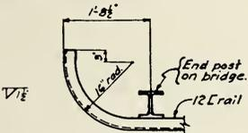
**PLAN VIEW OF RAILING AT BRIDGE ENDS**
