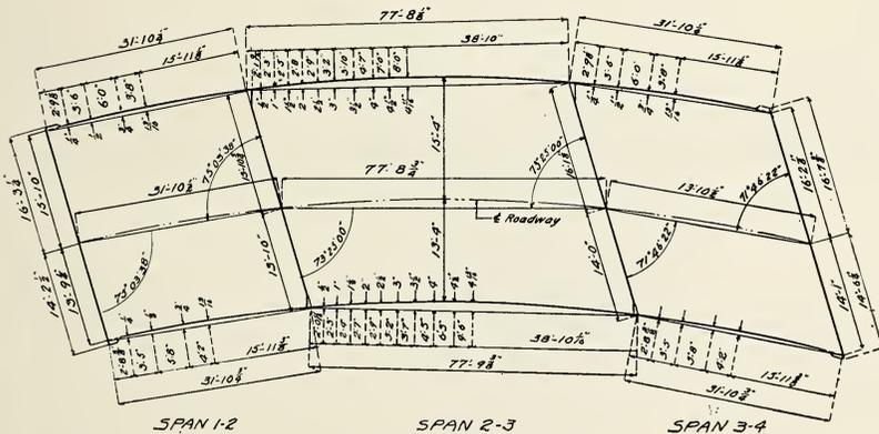
PLAN AND DIMENSIONS OF FLOOR SLAB
