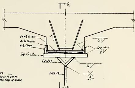
NOTE: 4 #4 BARS APPLIED & WELDED ONLY AFTER CONCRETE PRESTRESSED.
