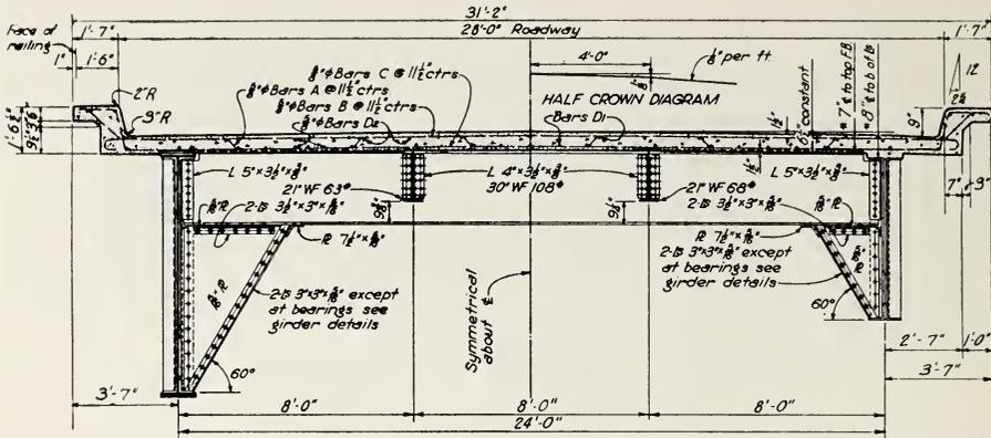
HALF SECTION THROUGH INTERIOR SPAN
