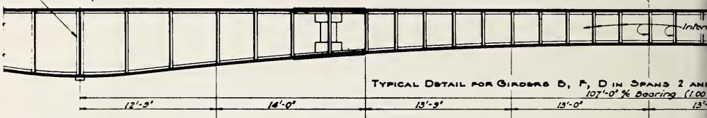
TYPICAL DETAIL FOR GIRDERS B, F, D IN SPANS 2 AND 4
