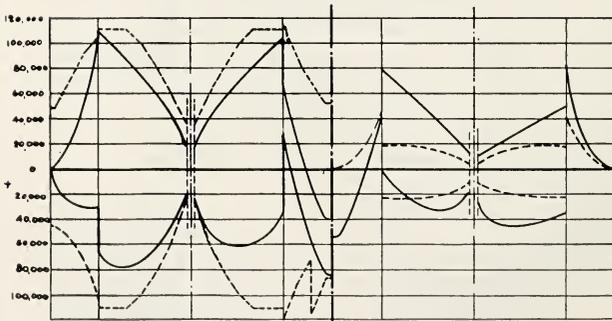
max M GIRDER    max Kern Point M of Arch    max M Girder - Kern Point Moments of Arch-Girder Moments
