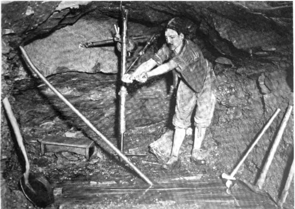
Fig. 9.—A Stoneman at Work with a Hand-drilling Machine in the face of a Stone Drift.
