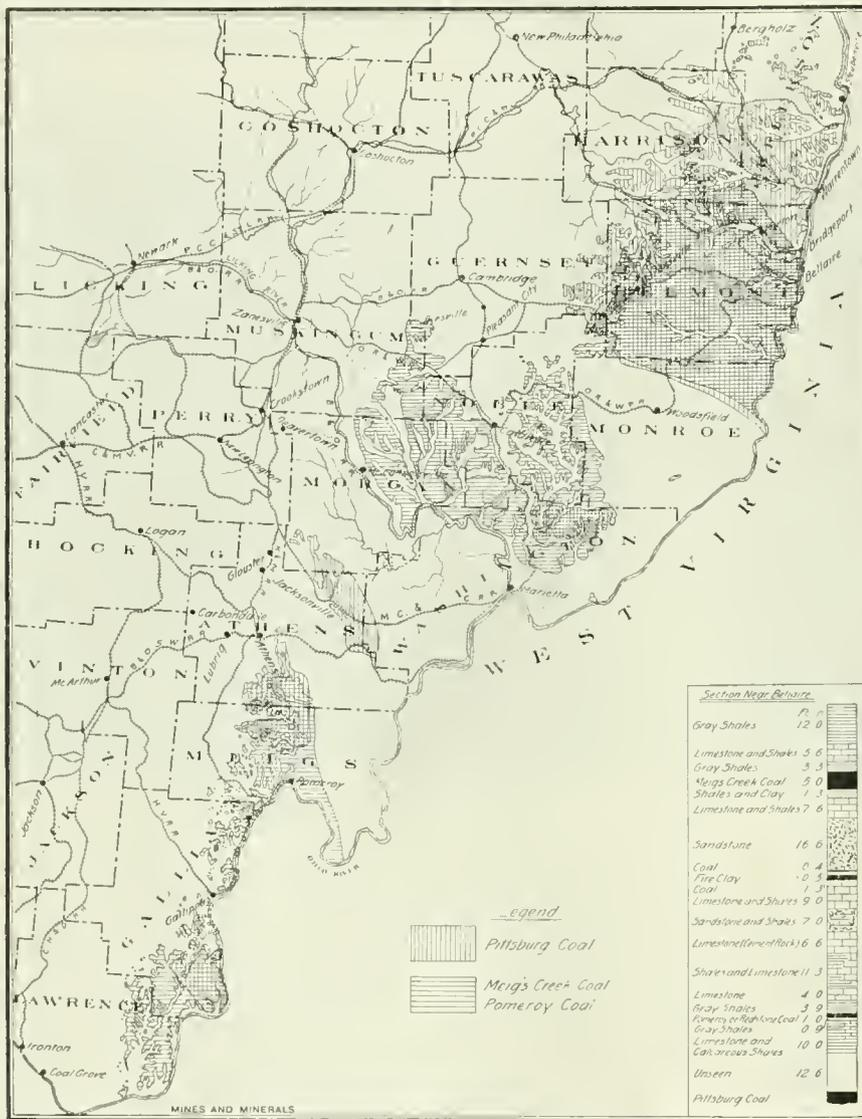
FIG. 1. MAP SHOWING COAL FIELDS OF OHIO
