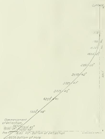
FIG. 2. PLAN SHOWING DEFLECTED BORE HOLE
