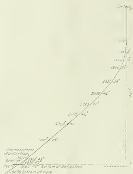
FIG. 2. PLAN SHOWING DEFLECTED BORE HOLE
