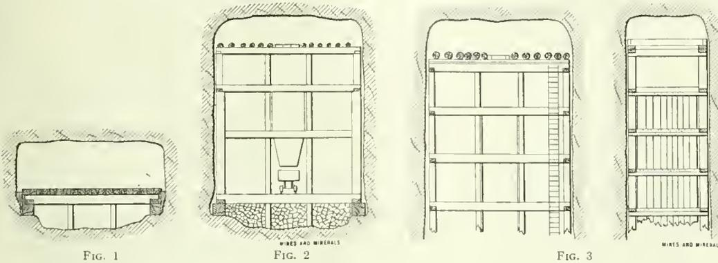
When the shaft was raised from the 7th level at the Armenia mine of Corrigan, McKinney & Co., the following method was used.
