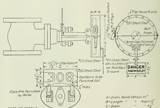
FIG. 8. LOCKING DEVICE FOR VALVES
