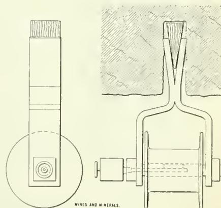
in position, the wooden wedge is drawn down about 2 inches, the shank fitted over it and the whole driven up as far as possible. As the wedge drives the shanks apart and into the roof, permanency is secured. In some cases additional wedges are placed outside the shank between it and the sides of the hole, and further security might be obtained if the device was cemented into place. However, at both the above mines, cementing is not employed and no falls of the sheave have been reported.
