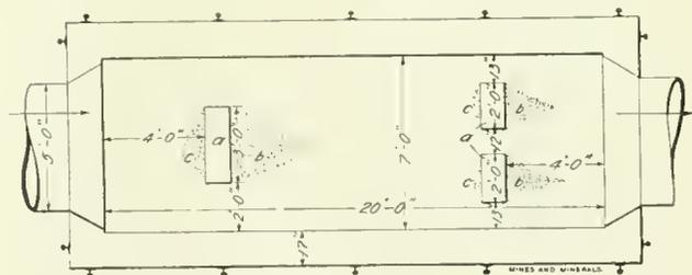
FIG. 2. PLAN OF SETTLING CHAMBER
