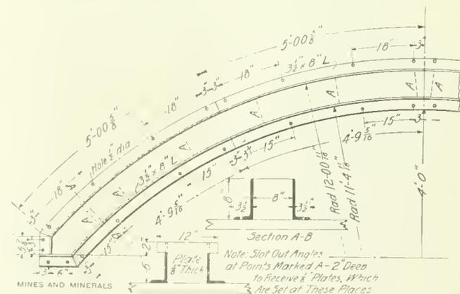
FIG. 14. STEEL FORM FOR MAKING CONCRETE BLOCK ARCH
