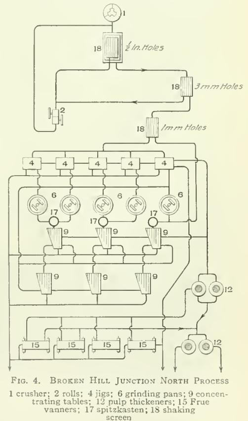
FIG. 4. BROKEN HILL JUNCTION NORTH PROCESS
