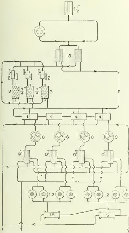
FIG. 3. BROKEN HILL SOUTH MINE PROCESS
