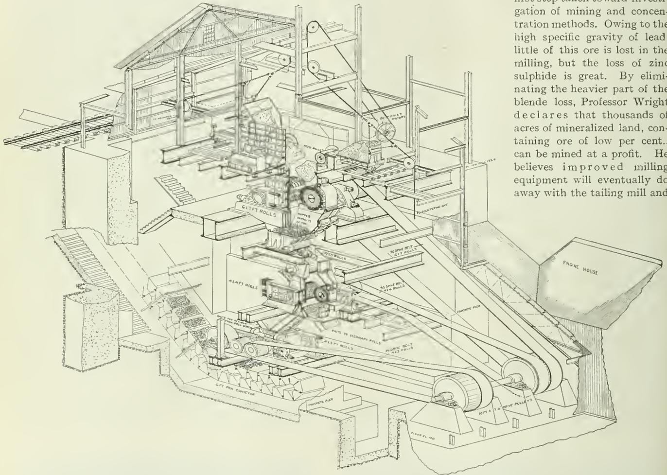
FIG. 3. TOMKINS COVE CRUSHING AND SIZING PLANT
