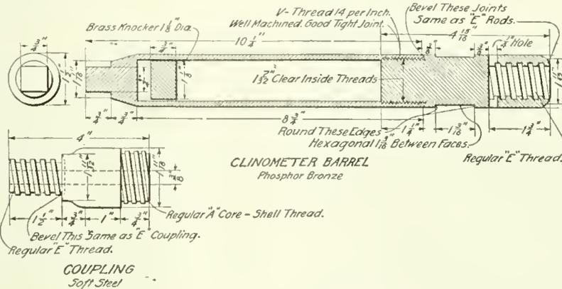
FIG. 1. DRILL HOLE CLINOMETER
