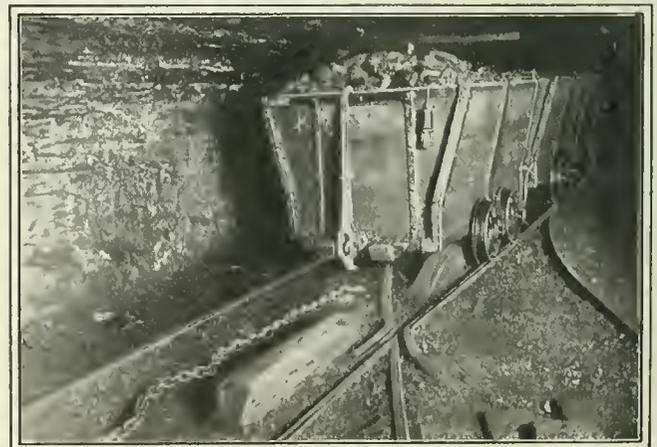
FIG. 5. NEW ARRANGEMENT FOR RELEASING TAIL-ROPE
