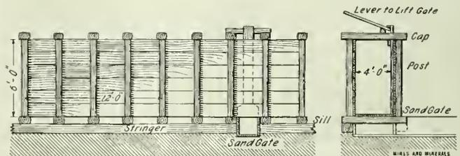
FIG. 4. FLUME WITH SAND GATE
