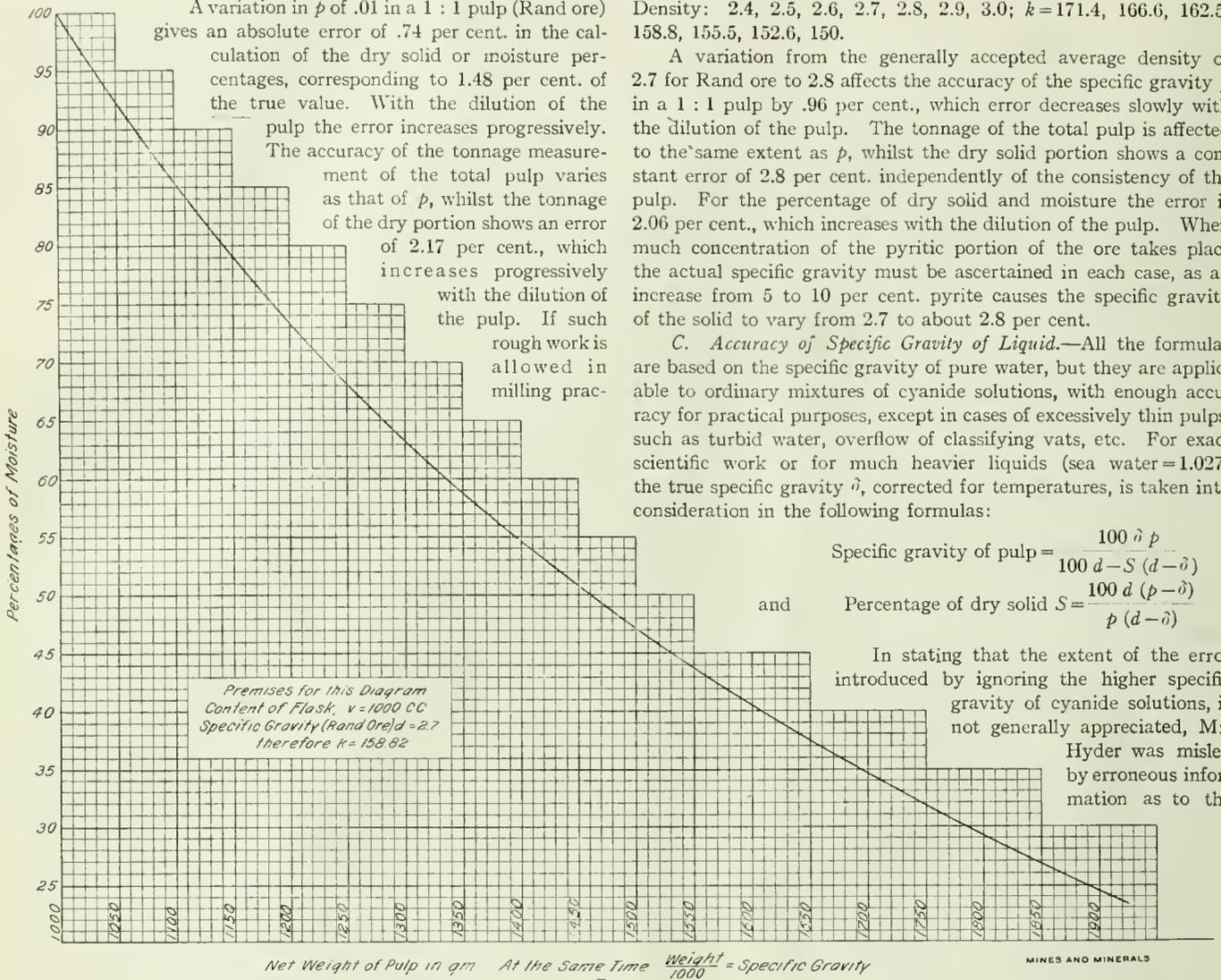
$$\text{Specific gravity of pulp} = \frac{100 \delta p}{100 d - S (d - \delta)}$$
