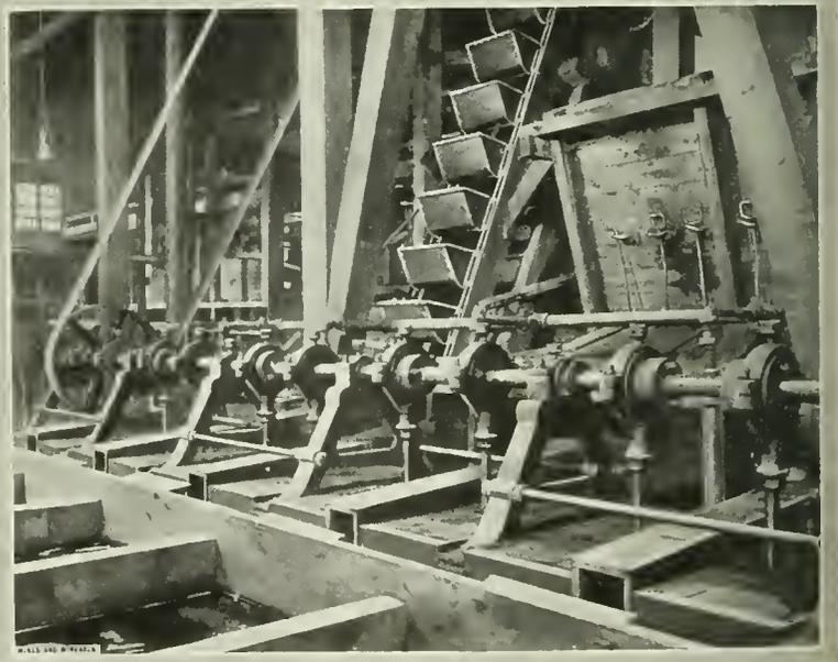
FIG. 2. LUHRIG REWASHING JIGS AND WASHED COAL ELEVATOR
