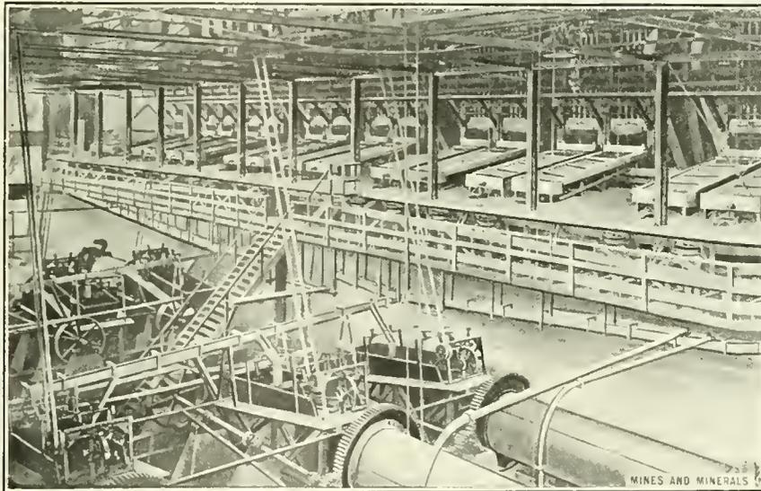
FIG. 1. BATTERY AND TUBE-MILL FLOOR OF CONCENTRATING MILL
