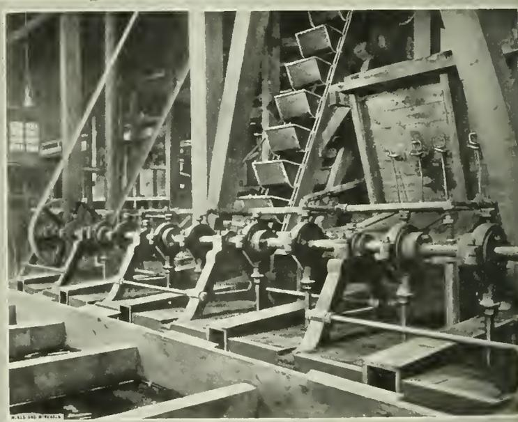
FIG. 2. LUHRIG REWASHING JIGS AND WASHED COAL ELEVATOR
