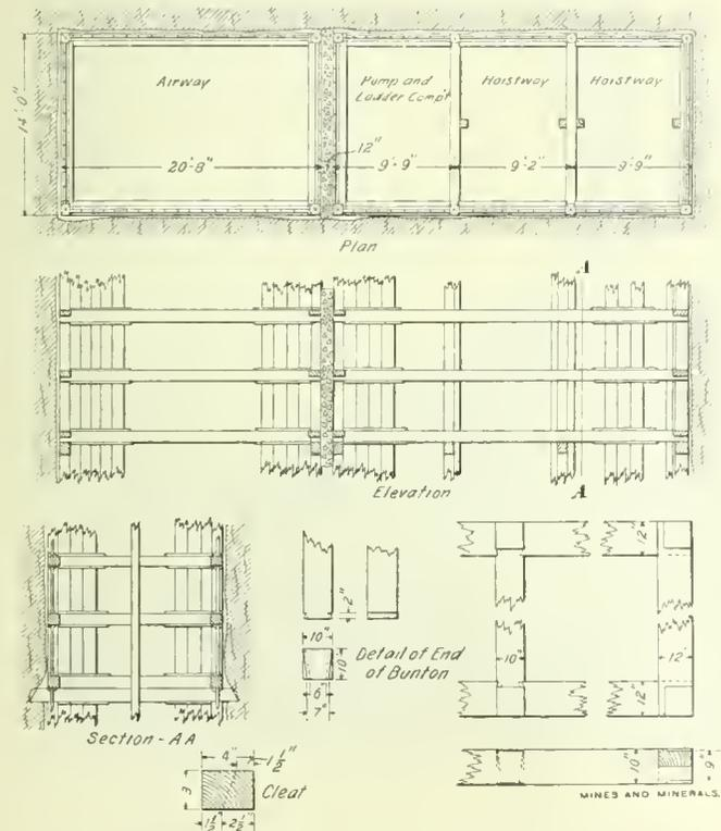
FIG. 3. PLAN AND DETAILS OF TIMBERING, LOOMIS SHAFT
