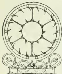
FIG. 3. END SECTION ROTARY DRIER, SHOWING CONCENTRIC SHELLS
