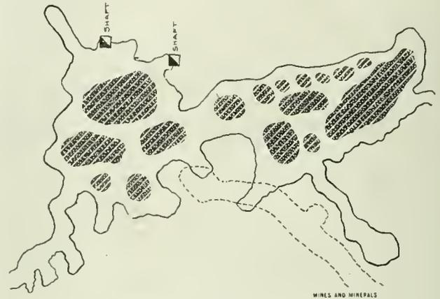
FIG. 2. METHODS OF DRIFTING IN DISSEMINATED ORE
