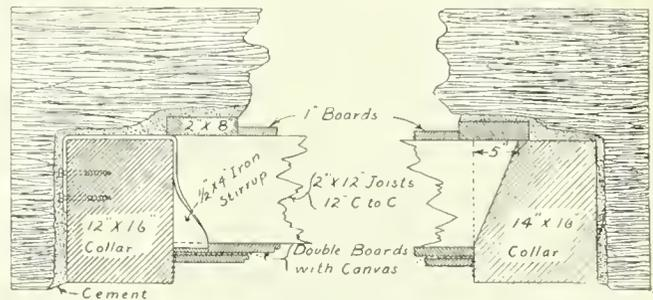
FIG. 2. DETAILS OF OVERCAST
