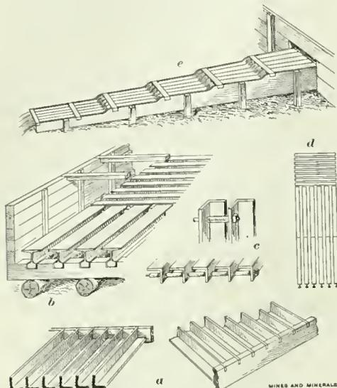
FIG. 3. RIFFLES AT KINGSBURY PLACER
