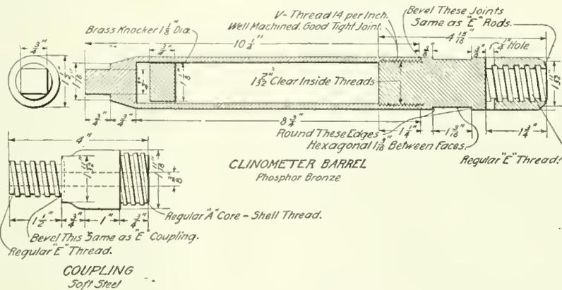
FIG. 1. DRILL HOLE CLINOMETER
