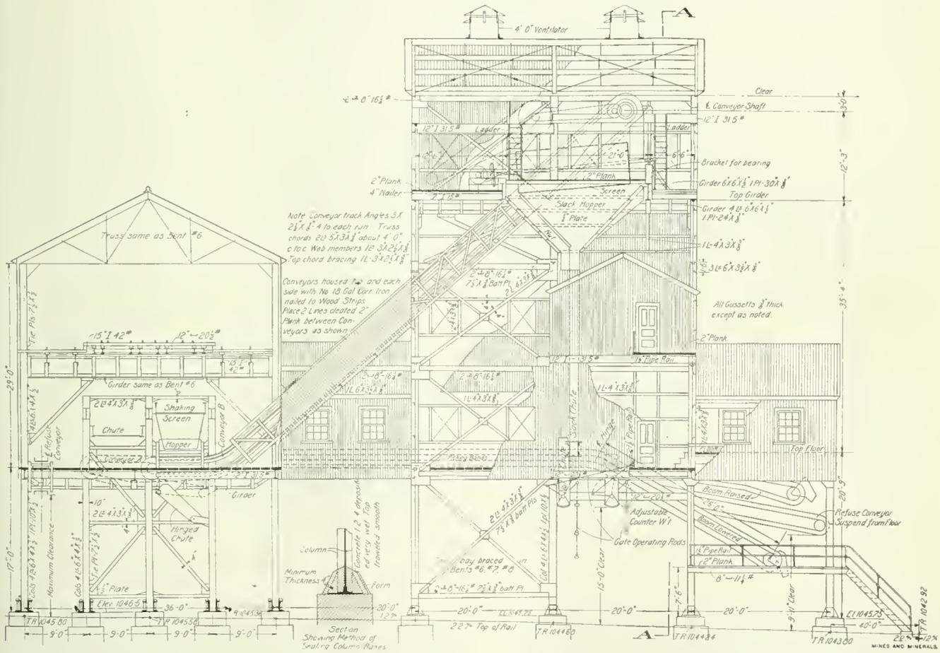
FIG. 6. SIDE ELEVATION OF HOISTING SHAFT TIPPLE
