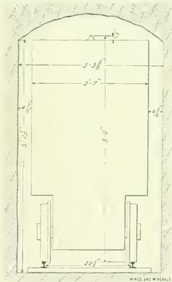
FIG. 1. CROSS-SECTION OF ADIT AND LOCOMOTIVE
