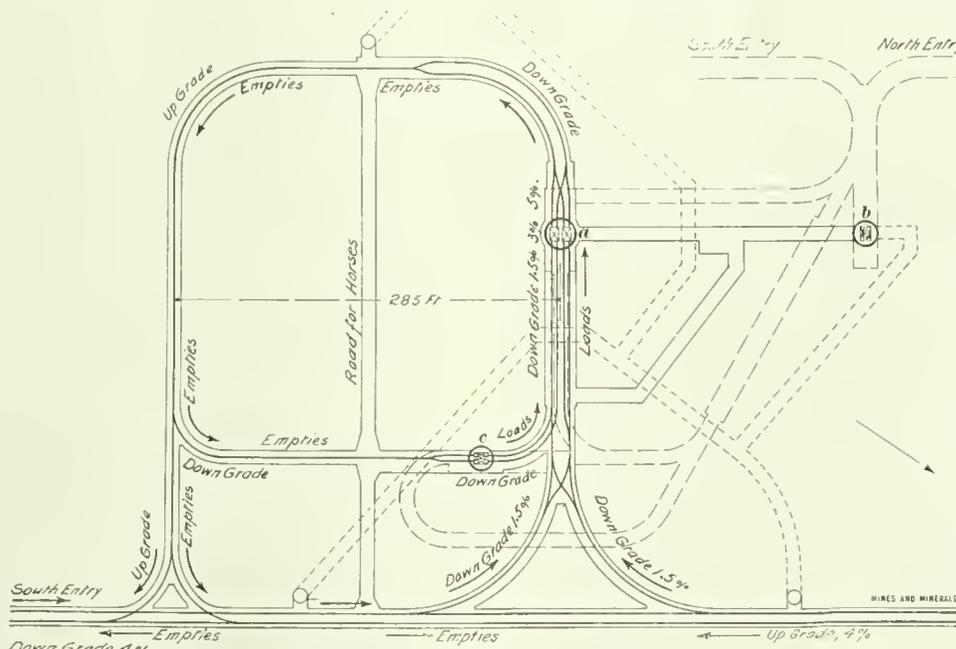
FIG. 1. PLAN OF SHAFT BOTTOM AT ARENBERG MINE
