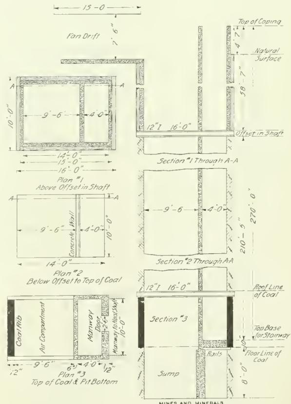
FIG. 8. PLANS AND LONGITUDINAL SECTIONS OF AIR SHAFT
