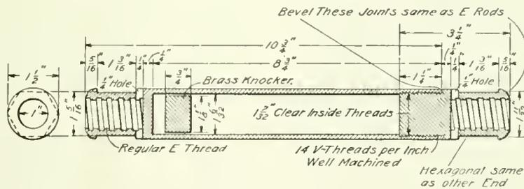
FIG. 2. PHOSPHOR BRONZE DRILL HOLE CLINOMETER
