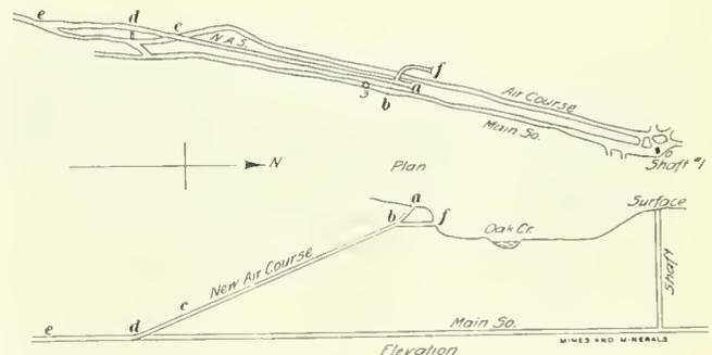
FIG. 1. PLAN AND ELEVATION OF AIR SLOPE
