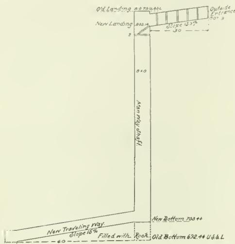
FIG. 1. SKETCH OF MANWAY SHAFT AT IMPERIAL MINE
