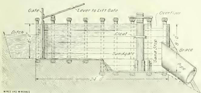
FIG. 5. PENSTOCK CONNECTING PIPE LINE WITH DITCH
