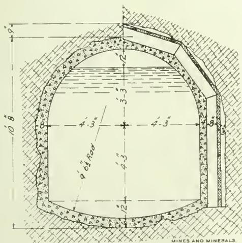
FIG. 1. SECTION OF TUNNEL No. 17, JAWBONE DIVISION
