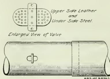
FIG. 6. PIPE LINE WITH AIR VALVE
