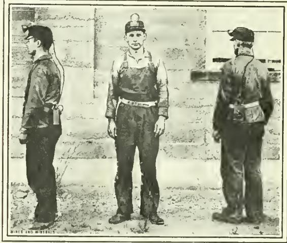
FIG. 2. ELECTRIC LAMP OUTFIT AS WORN
