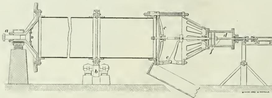
FIG. 1. SECTION, BURT REVOLVING FILTER
