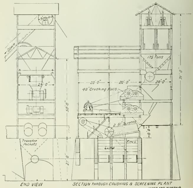
FIG. 8. END VIEW AND SECTION, ORE PREPARING PLANT
