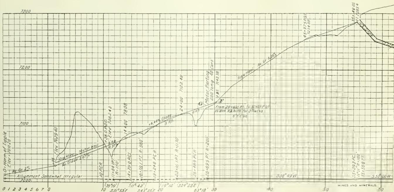
FIG. 5. SECTION SHOWING HAULAGE GRADES
