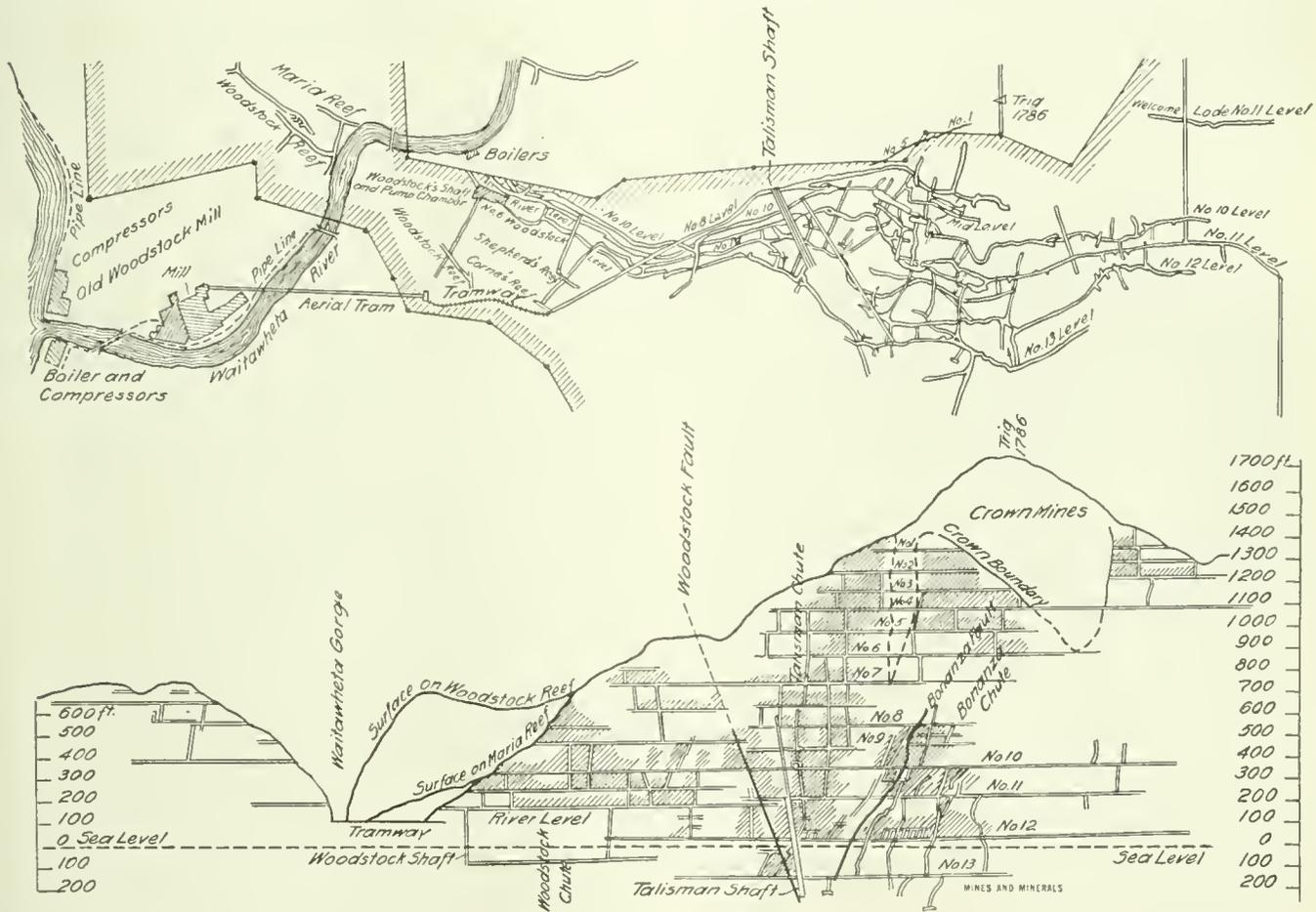
FIG. 1. PLAN AND VERTICAL PROJECTION OF PART OF TALISMAN MINE
