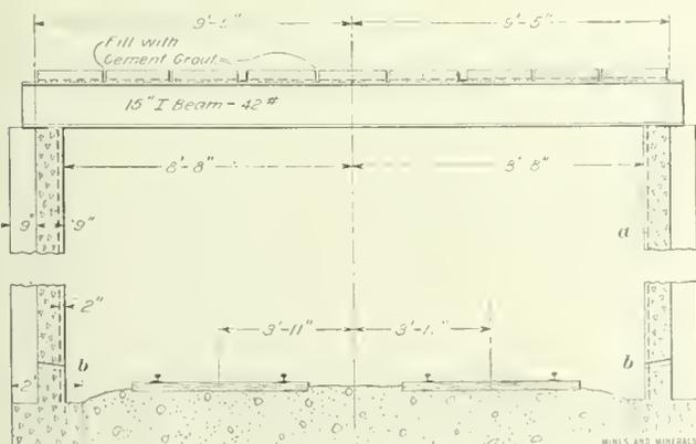
FIG. 13. SECTION OF HEADING, SHOWING CONCRETE SLAB WORK
