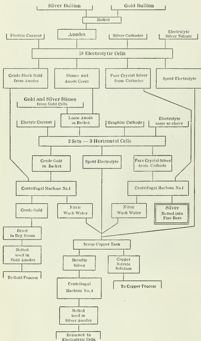
FIG. 4. DIAGRAM OF SILVER PROCESS
