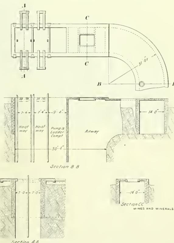
FIG. 5. PLAN AND SECTION OF AIRWAY, LOOMIS SHAFT
