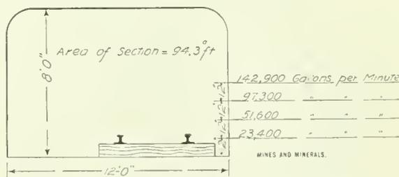
FIG. 1. CROSS-SECTION OF DRAINAGE TUNNEL
