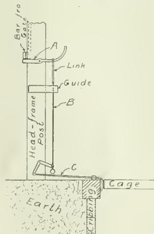
FIG. 1. LOCKING DEVICE FOR SAFETY GATE
