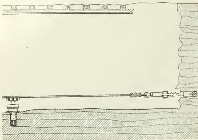
FIG. 3. APPROVED METHOD OF DEAD ENDING TROLLEY WIRE
