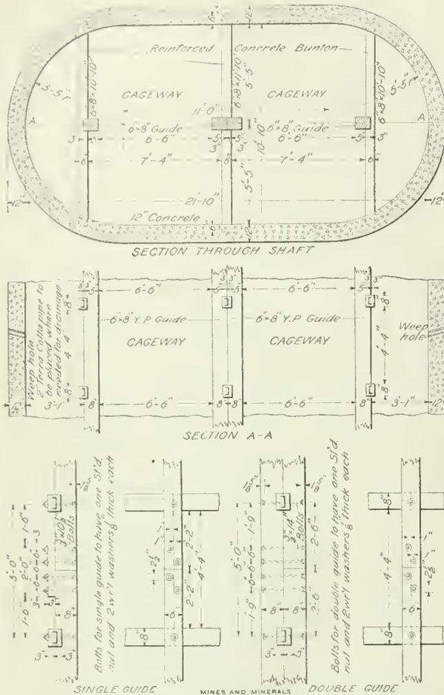
FIG. 2. SECTION, ELEVATION AND DETAILS OF SHAFT LINING
