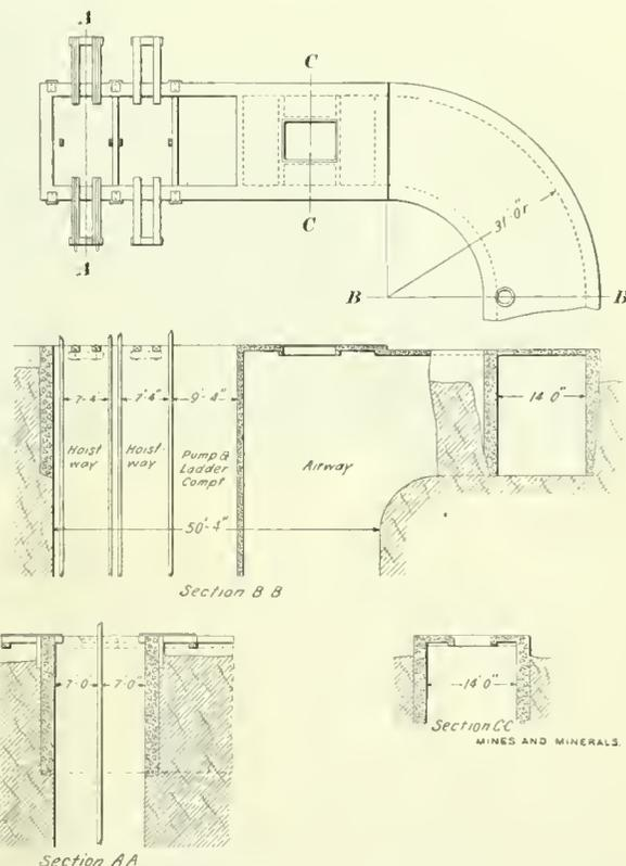
FIG. 5. PLAN AND SECTION OF AIRWAY, LOOMIS SHAFT
