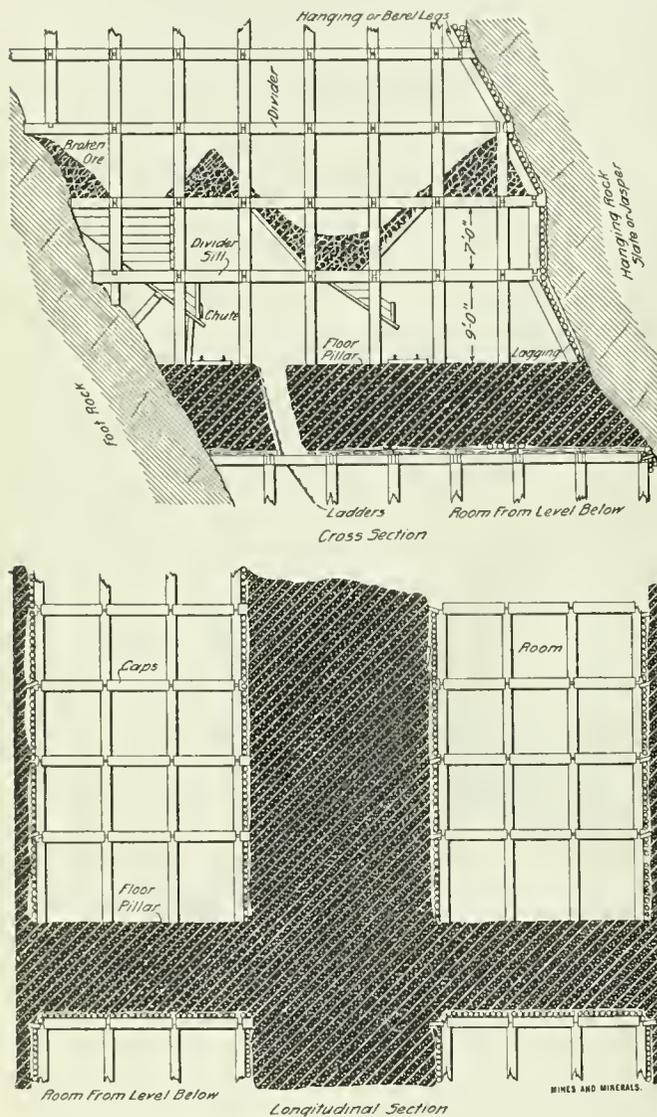
FIG. 3. VERTICAL SECTIONS SHOWING SQUARE SET TIMBERING AND SCHEME OF MINING
