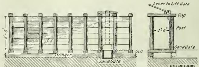
FIG. 4. FLUME WITH SAND GATE
