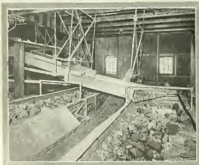
FIG. 8. SHAKING SCREEN DISCHARGING ON TO PICKING BAND
