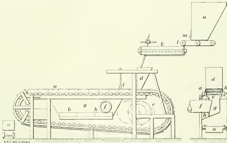
FIG. 1. LONGITUDINAL AND CROSS SECTION OF SINTERING MACHINE
