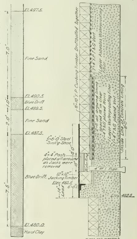
FIG. 11. PLACING OF WATERPROOF LINING
