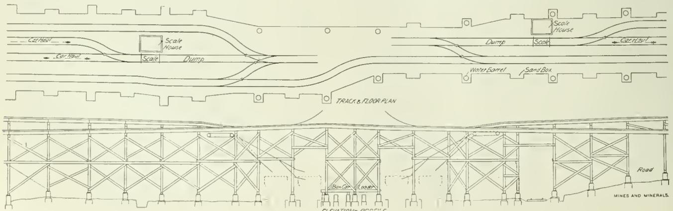
FIG. 2. PLAN AND ELEVATION OF TIPPIL AT DELAGUA MINE
