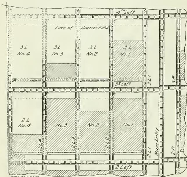
FIG. 1. LONGWALL MINING WORKED ADVANCING
