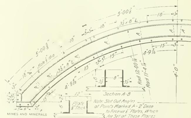
FIG. 14. STEEL FORM FOR MAKING CONCRETE BLOCK ARCH
