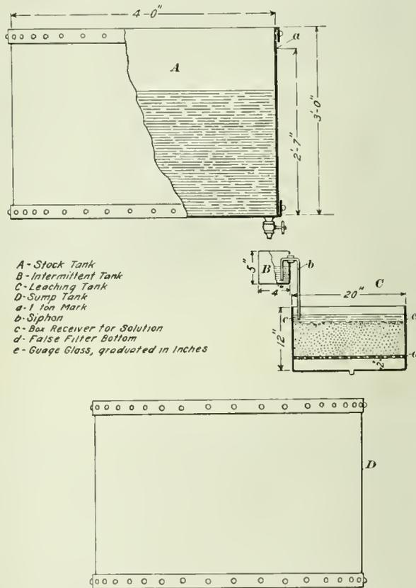
FIG. 2. TANKS FOR CYANIDE TESTS
