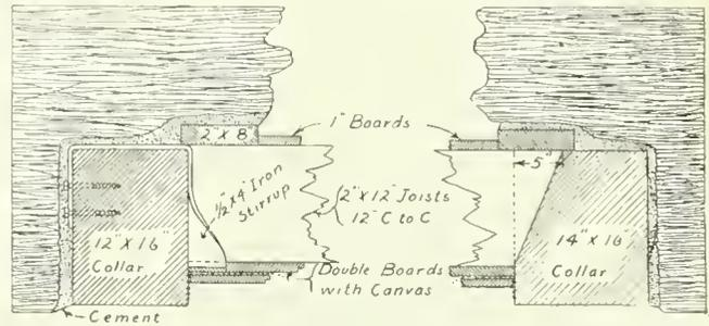
FIG. 2. DETAILS OF OVERCAST
