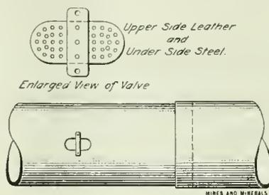
FIG. 6. PIPE LINE WITH AIR VALVE
