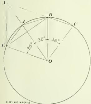
But as the angles  $ACO + COB + BOA = 144$  degrees, then the angle  $OAC = 36$  degrees also; therefore, the triangle *ABJ* is isosceles and the line *AJ* equals the chord *JB*.
