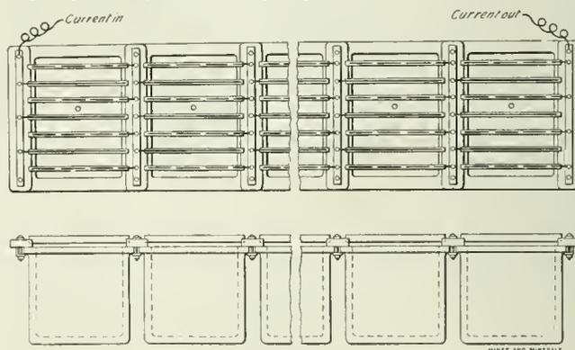
FIG. 9. PATH OF CURRENT THROUGH GOLD CELLS
