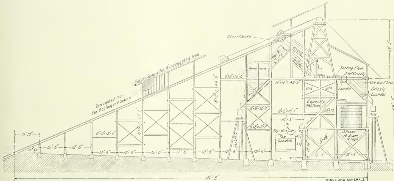
FIG. 1. HEAD-FRAME AND ORE BIN
