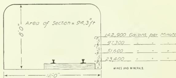
FIG. 1. CROSS-SECTION OF DRAINAGE TUNNEL
