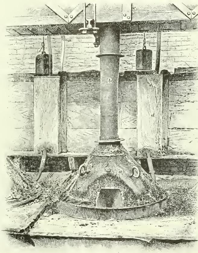
FIG. 2. UPPER PART OF PARTING KETTLE
