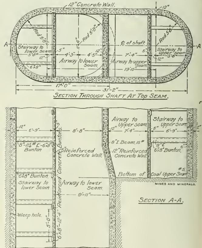
FIG. 3. SECTION AND ELEVATION OF SHAFT LINING
