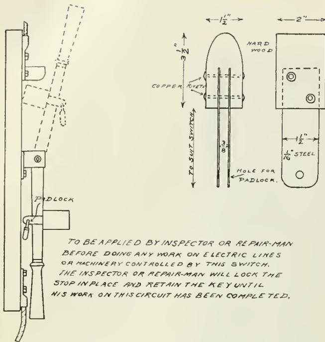
FIG. 6. LOCK FOR ELECTRIC SWITCH
