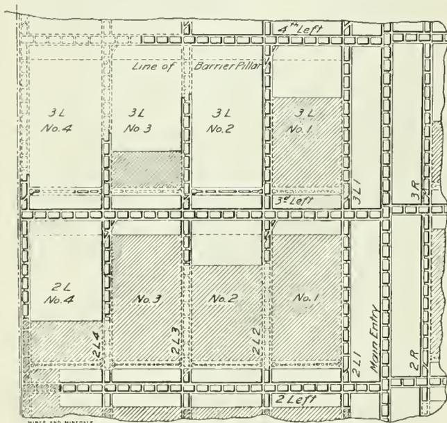
FIG. 1. LONGWALL MINING WORKED ADVANCING
