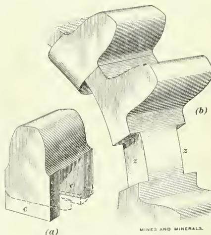
place of the broken tooth, is smoothed on the face of the wheel and two slots *z* cut in it. After being heated the prongs, *c* of the new tooth are placed in the slots, *z*, in the rim of the wheel and hammered up against the inner side thereof. Upon cooling they are absolutely tight and firm. In the figure the ends of the prongs are shown in dotted lines as partly bent under in their final position. These teeth have proven durable.
