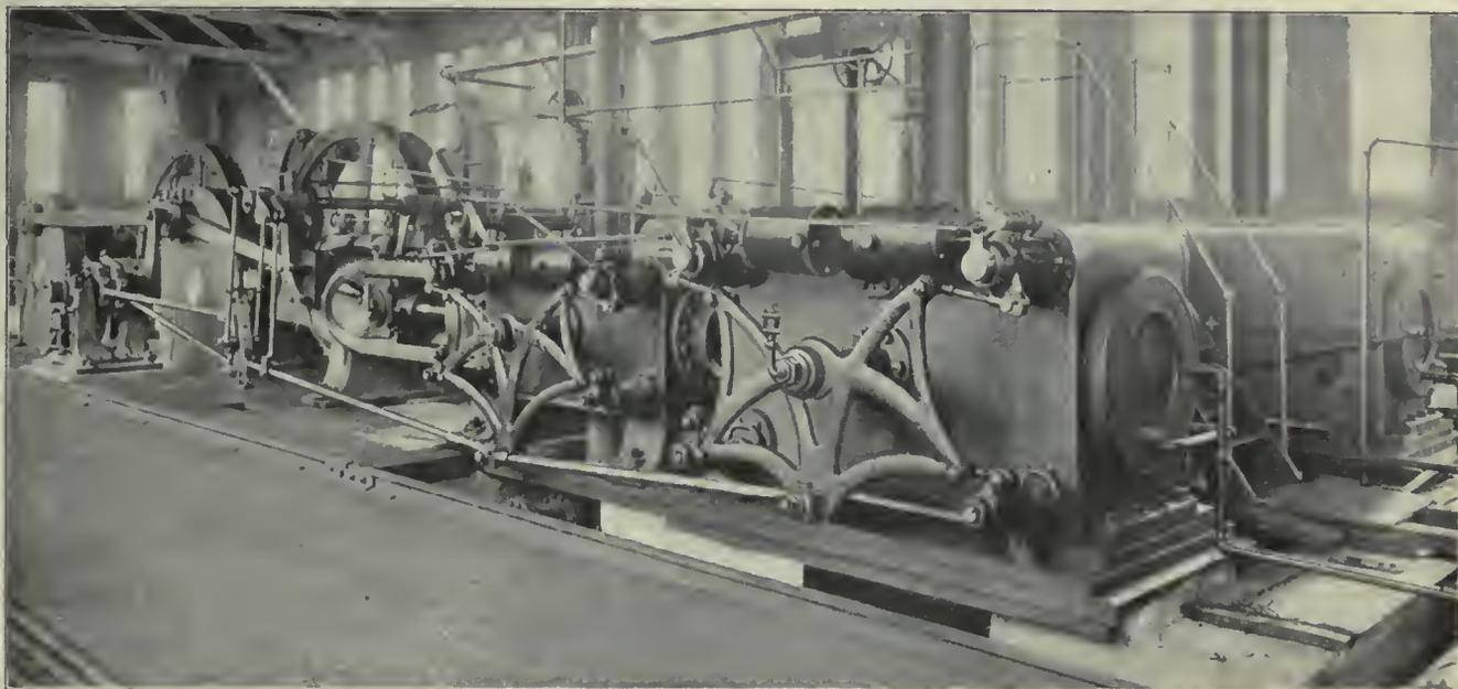
FIG. 35. WHITING HOISTING ENGINE AT RAND MINE, LTD.
