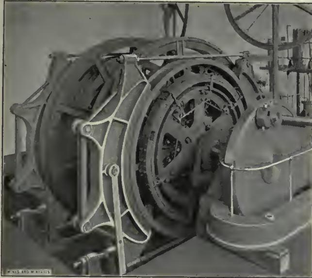
FIG. 29. HOIST WITH TWO LOOSE REELS AND FRICTION CLUTCH
