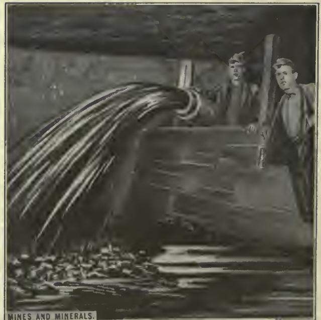
FIG. 6. FLUSHING CULM
