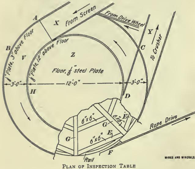
necessary to provide for a careful inspection of the coal as coming from the mine, that too much rock might not be sent out, thus overloading the washers and affecting the ash content of the coke. By reason of the screens, chutes, crushers, etc., being already installed, and by reason of the limited space available, the inspection table at this plant presents many points of interest.
