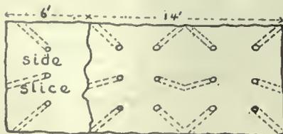
FIG. 3. PLAN OF DRILL HOLES IN ROOM MINING
