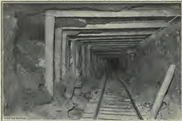
FIG. 7. STEEL MINE TIMBERS, BARTON MINE, No. 3 ENTRY, Y. & O. COAL CO., BARTON, OHIO
