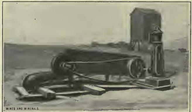
FIG. 1. BLOWING AIR DOWN A DRILL HOLE
