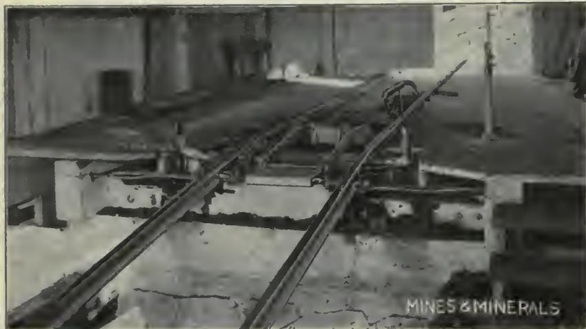
FIG. 2. CAR-DUMPING ARRANGEMENT
