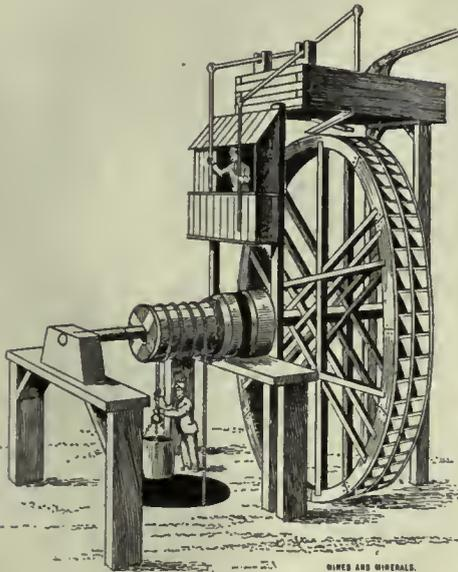
FIG. 11. DOUBLE WATERWHEEL HOIST
