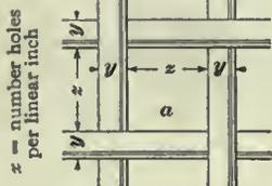
TABLE C. WIRE SCREENING. RELATIONS BETWEEN DIAMETER OF APERTURE, DIAMETER OF WIRE, SCREEN AREA AND NUMBER OF HOLES PER LINEAR INCH IN ANY SCREEN HAVING THE SAME NUMBER OF HOLES EACH WAY AND MANUFACTURED WITH ONE GAUGE OF WIRE ONLY
