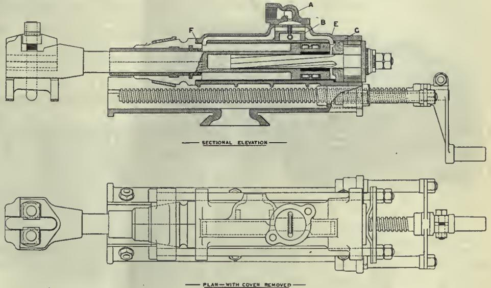
FIG. 4. THE HOLMAN 2 1/2-IN. STOPPING AIR-VALVE DRILL
