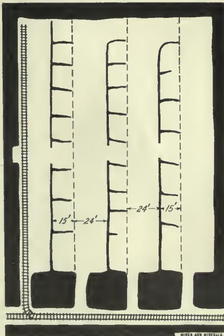
FIG. 9. SHOWING COAL LEFT IN ROOM PILLARS
