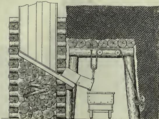
FIG. 4. LOADING CHUTE AT BOTTOM OF RISER
