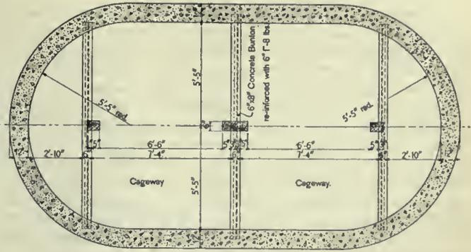
Elliptical Hoisting Shaft
