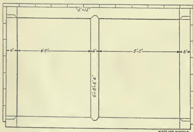
FIG. 2. SHAFT TIMBERING
