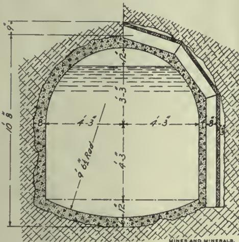
FIG. 7. SECTION OF TUNNEL No. 17, JAWBONE DIVISION
