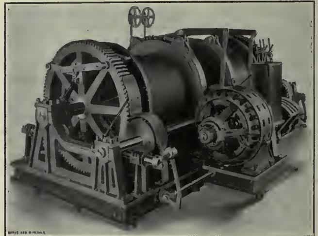
FIG. 53. DOUBLE DRUM, ELECTRIC HOIST, MESSINA, ALA.
