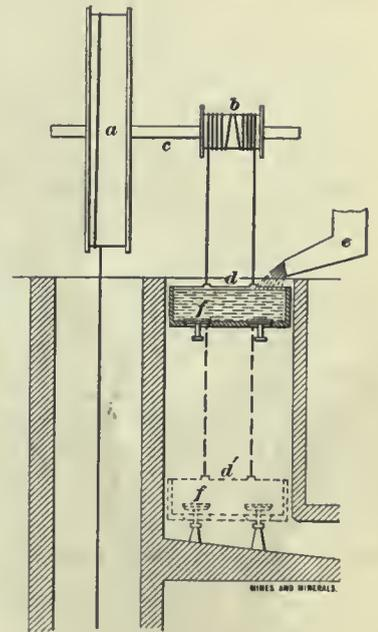
FIG. 13. WATER TANK HOIST
