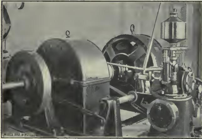
FIG. 1. PELTON GENERATING UNIT, UTAH METALS CO. TUNNEL
