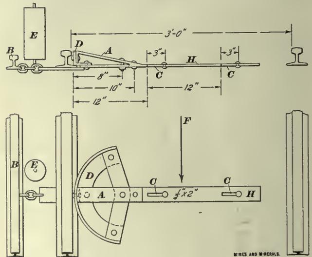
it may enter the sheaves. To do away with this extra labor an effective and cheaply constructed device is in use at the Radiant mine of the Victor-American Fuel Co., near Florence, Colo., and for a description of it we are indebted to J. Q. McNatt, mining engineer, of the latter city.
