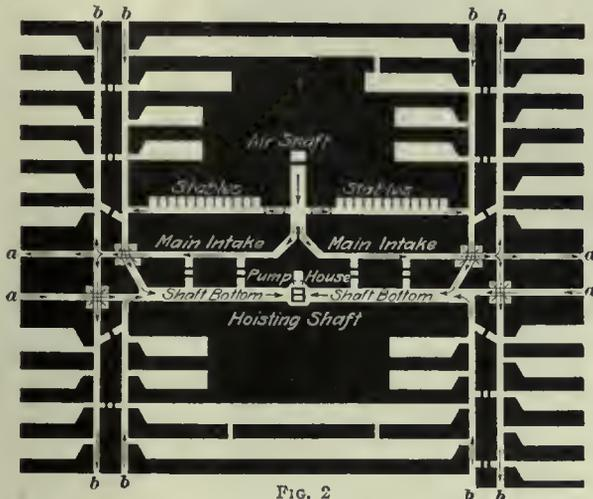
distributed so as to meet the needs in different parts of the workings; trouble with gas or the circulation of air in one section does not affect other sections of the mine; and finally, it is possible, then, to concentrate the entire circulation upon any single section of the mine, temporarily, by closing down other unaffected sections till the trouble is overcome.
