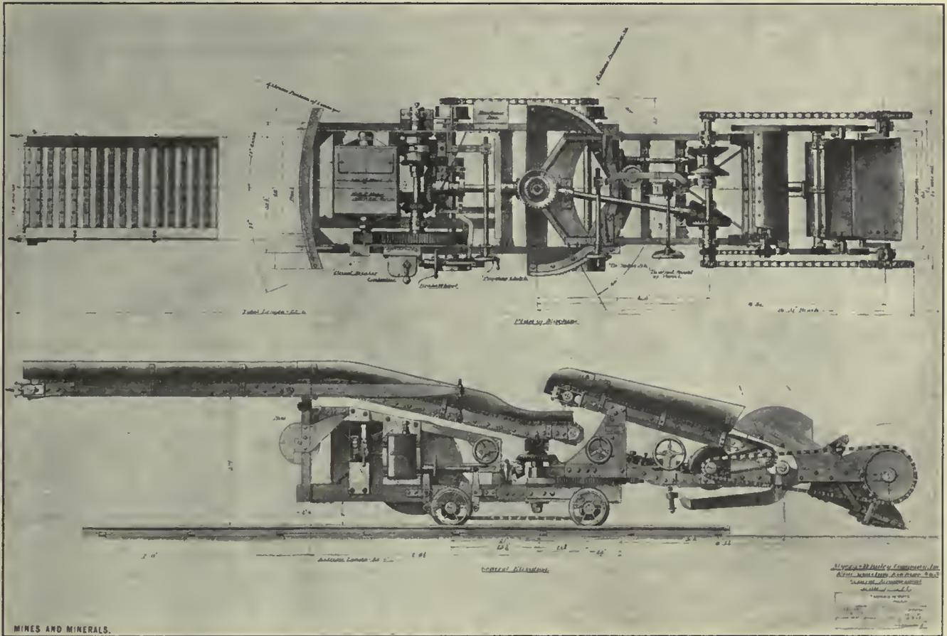
FIG. 3. PLAN AND ELEVATION OF COAL-LOADING MACHINE
