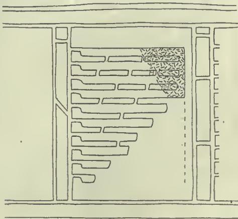
FIG. 2. PILLAR DRAWING, FACES AT ANGLE TO SIDE
