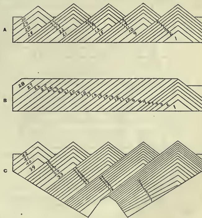
FIG. 2. DIAGRAMS REPRESENTING THE DISTRIBUTION OF COAL AS DUMPED FROM MINE CARS INTO RAILROAD CARS
