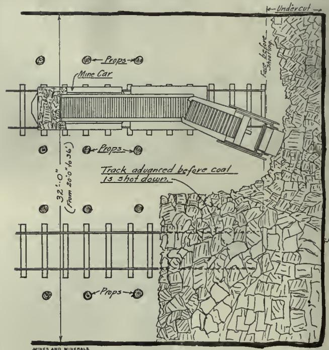
FIG. 5. WORKING FACE IN ROOM, HOLDEN MINE
