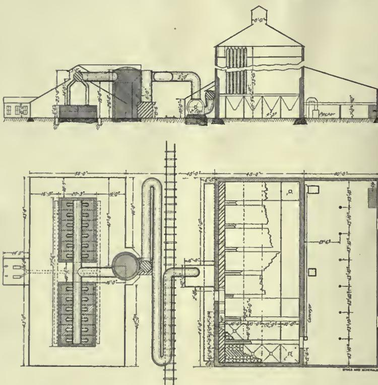
FIG. 1. PLAN AND ELEVATION OF ZINC-LEAD PIGMENT PLANT
