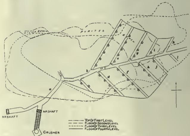
FIG. 3. PLAN OF HELEN IRON MINE
