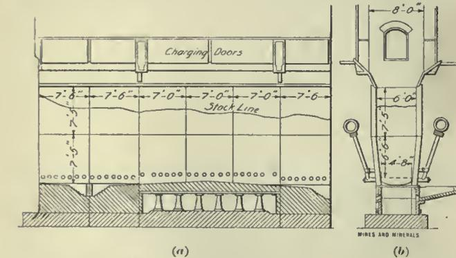
FIG. 1. WATER-JACKETED COPPER BLAST FURNACE, ANACONDA, MONT., 1909
