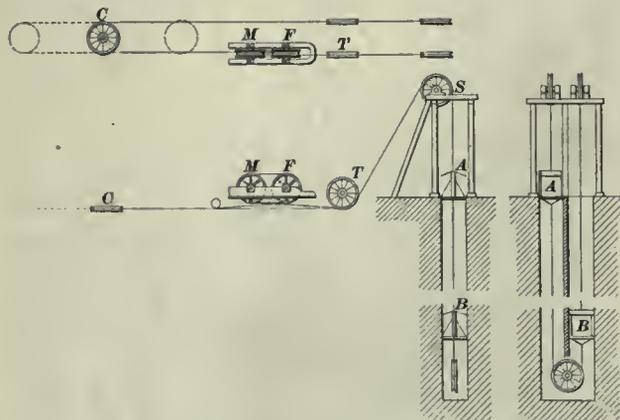
FIG. 36. PLAN AND ELEVATION OF WHITING SYSTEM
