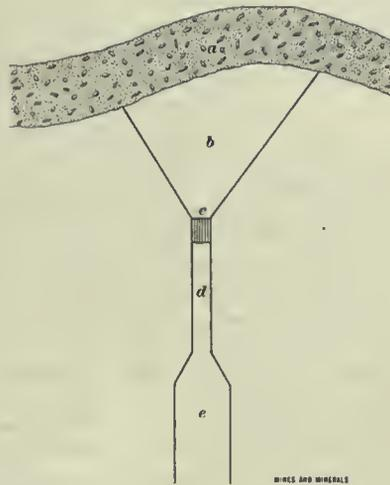
FIG. 5. a, Face; b, Head-Slucice; c, Grizzly; d, Feed Slucice; e, Slucice
