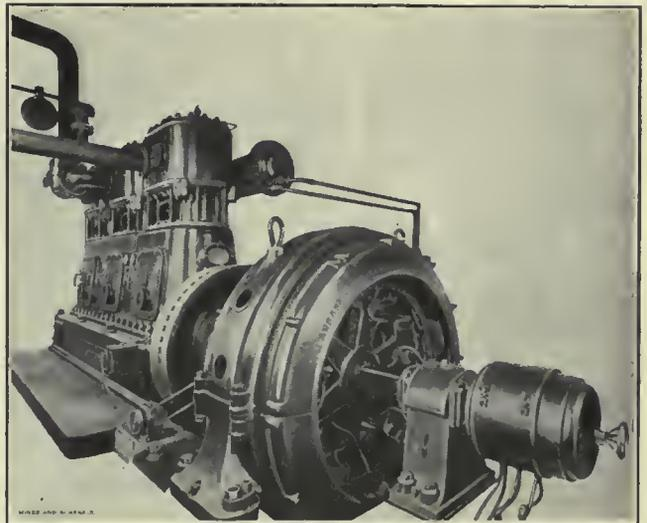
FIG. 1. ELECTRIC MOTOR DRIVING AIR COMPRESSOR
