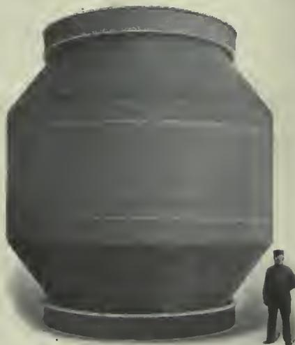
FIG. 39. DRUM OF HOIST, OSCEOLA MINE
