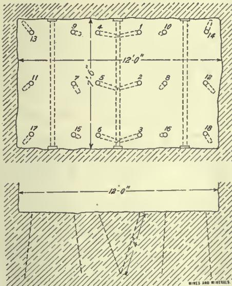
FIG. 3. BLASTING IN SHAFT SINKING
