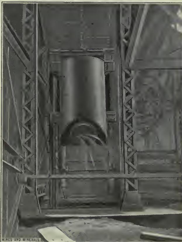
FIG. 1. REAR VIEW OF WATER BAILER
