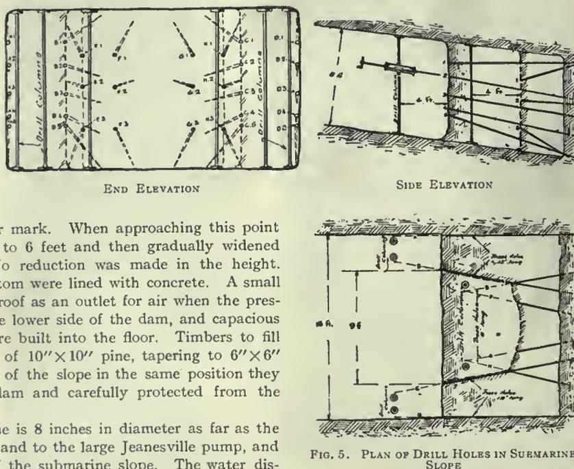
FIG. 5. PLAN OF DRILL HOLES IN SUBMARINE SLOPE
