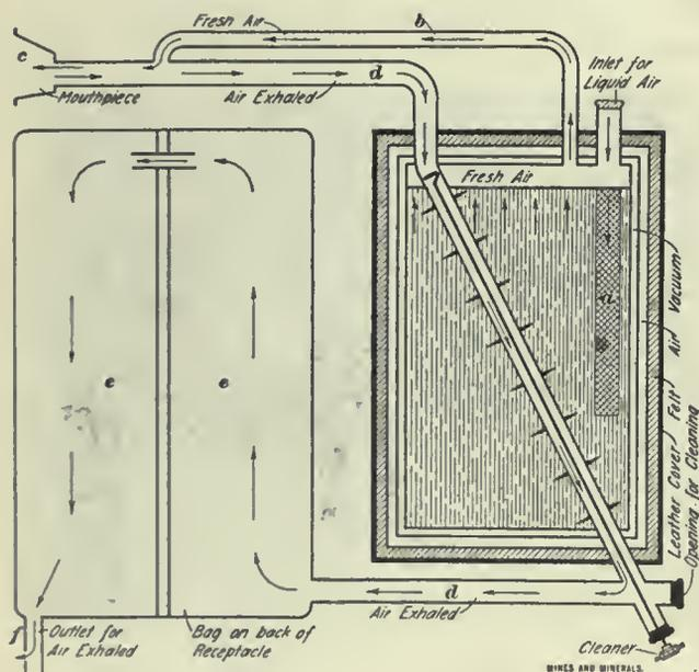
FIG. 2. DIAGRAM SHOWING CIRCULATION OF AIR IN AEROLITH
