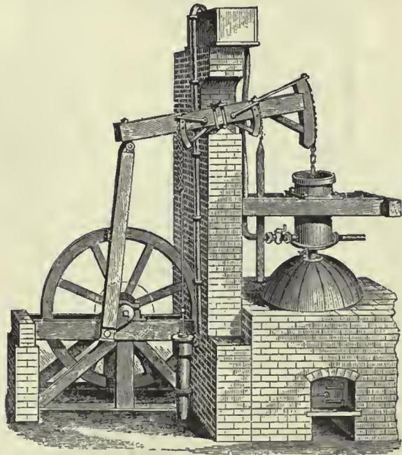
FIG. 14. NEWCOMEN ENGINE, WITH CRANK AND FLYWHEEL, 1780
