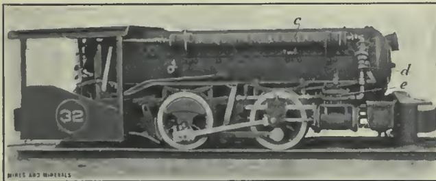
FIG. 3. RIGHT-HAND SIDE OF TWO-STAGE AIR LOCOMOTIVE
