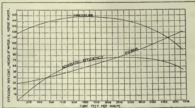
FIG. 5. PRESSURE, EFFICIENCY, AND POWER CURVES OF TURBOBLOWER
