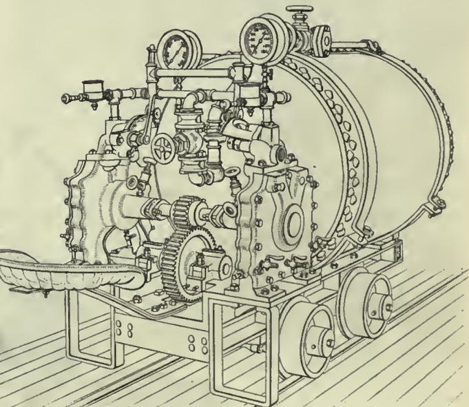
FIG. 54. COMPRESSED AIR LOCOMOTIVE USED IN TUNNEL
