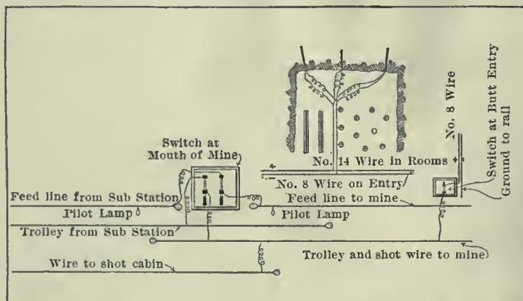
FIG. 2. DIAGRAM OF SHOT-FIRING SYSTEM IN DAWSON MINE
