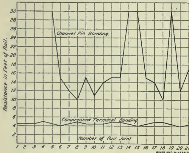
RESULT OF TESTS OF DIFFERENT KINDS OF RAIL BONDING
