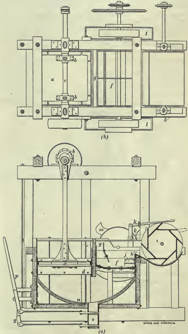
FIG. 1. PLAN AND ELEVATION OF HAZLETON JIG
