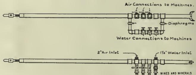
FIG. 2. COMBINATION MANIFOLD FOR AIR AND WATER
