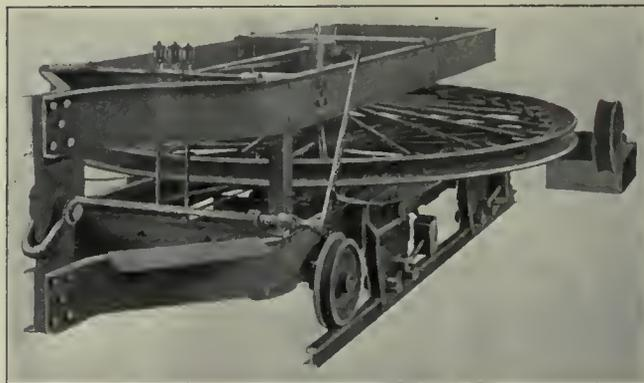
FIG. 37. TENSION CAR, WHITING SYSTEM
