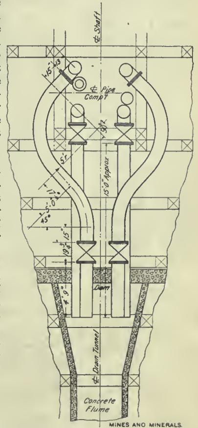
FIG. 3. PLAN OF CONNECTION OF COLUMNS TO DRAIN TUNNEL
