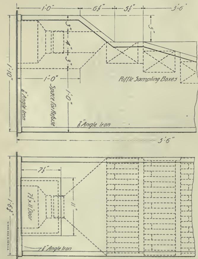
FIG. 3. PLAN AND ELEVATION OF RIFFLE SAMPLERS
