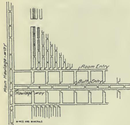
FIG. 3. SYSTEM OF WORKING
