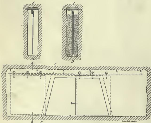
FIG. 1. PLANS AND SECTIONS OF MINE DOOR
