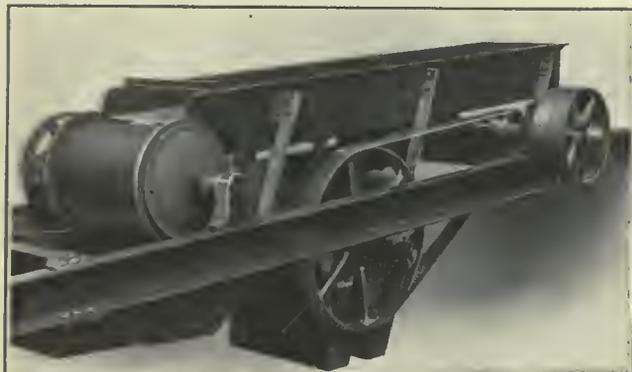
FIG. 1. TWO-POLE MAGNETIC SEPARATOR
