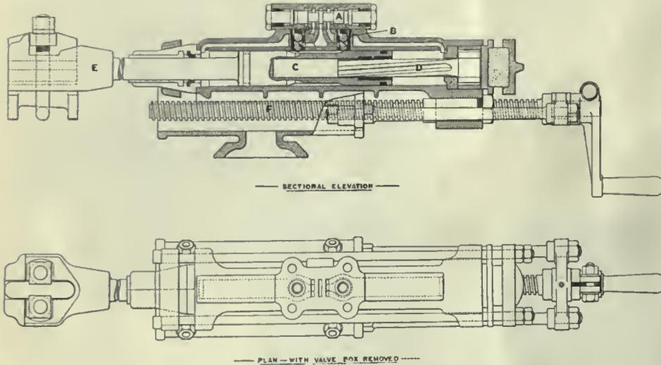
FIG. 2. THE HOLMAN 2½-IN. STOPPING AIR-VALVE DRILL
