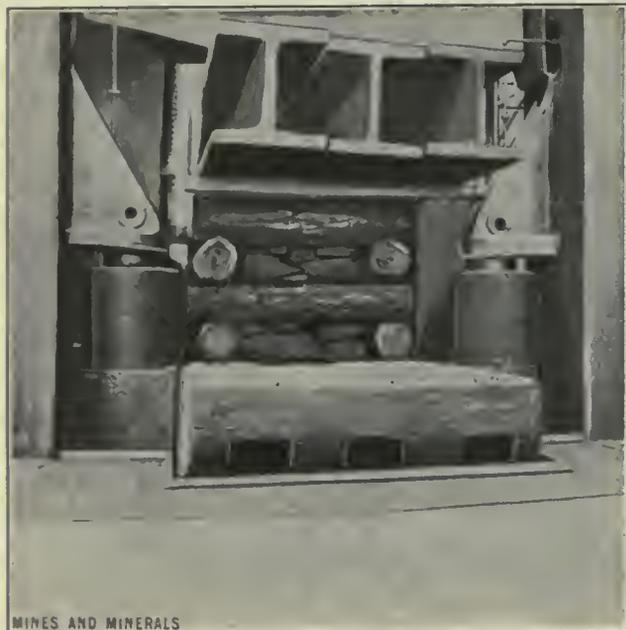
FIG. 3. CRUSHING A TIMBER CRIB
