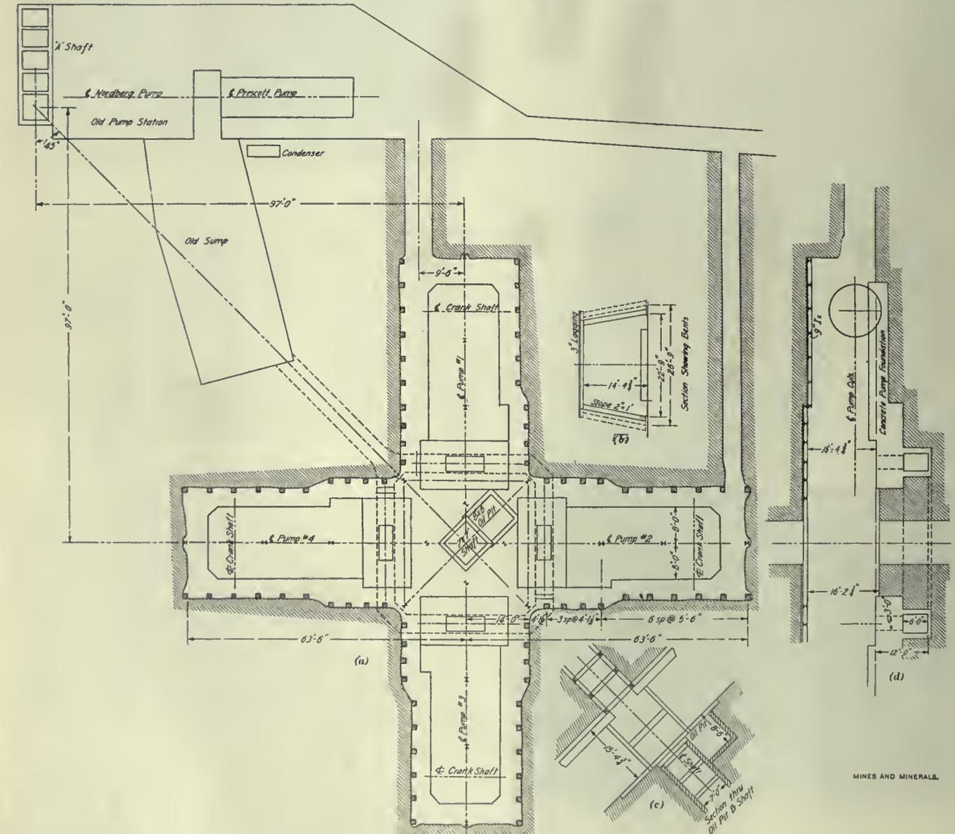
FIG. 1. PLAN OF PUMP STATION, 1,200-FOOT LEVEL "A" SHAFT
