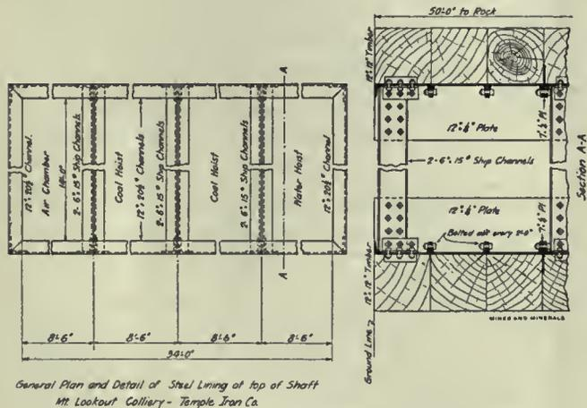
FIG. 2. STEEL-LINED SHAFT
