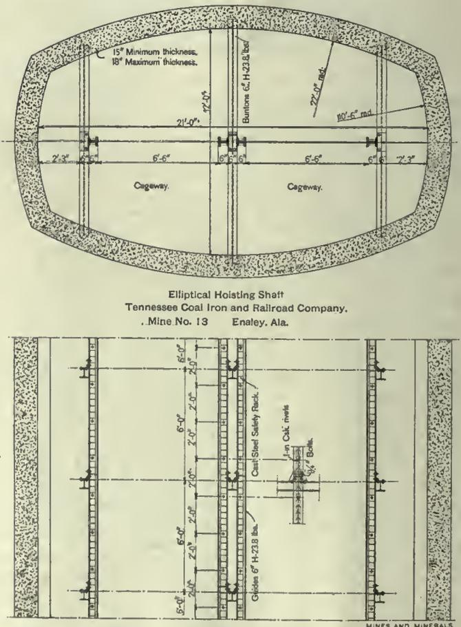
FIG. 5. ELLIPTICAL CONCRETE HOISTING SHAFT, WITH H SECTION BUNTONS AND GUIDES
