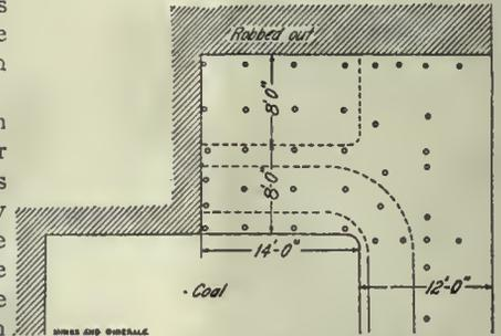
FIG. 10. COAL EXTRACTED, PLACE READY TO MAKE LAST FALL IN 42-FOOT CENTER ROOMS
