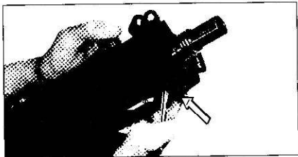
FIG. 13 Removing Pin Securing Receiver Group
