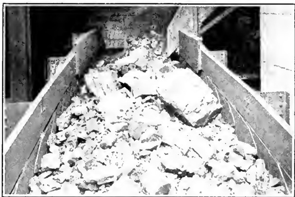
Coal discharging from inspection table on flight conveyor of 4,000 tons daily capacity. Note coarse character of coal.
