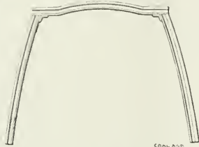
FIG. 1. CURVED "TIMBER SETS" IN GERMAN MINES
