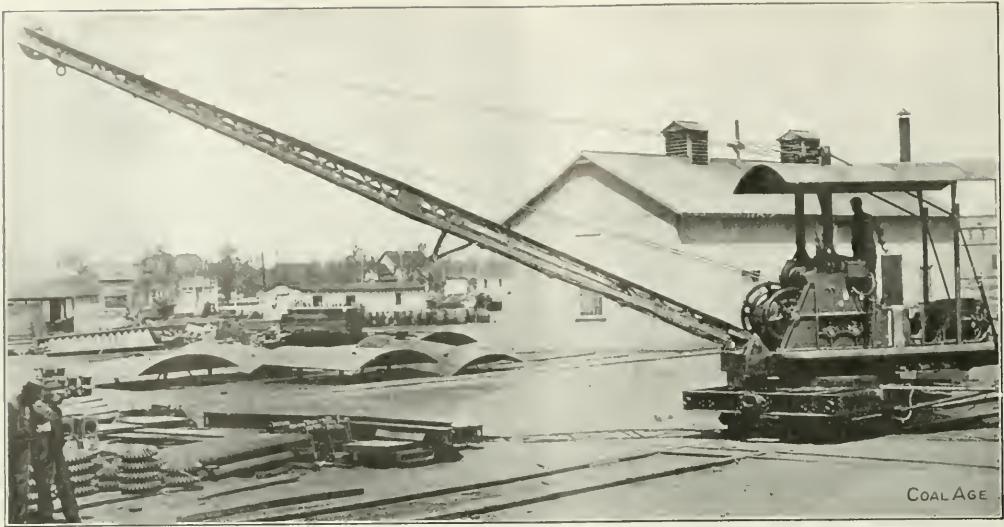
COAL-UNLOADING CRANE DRIVEN BY CONTINUOUS-CURRENT MOTOR OF THE MINE-LOCOMOTIVE TYPE
