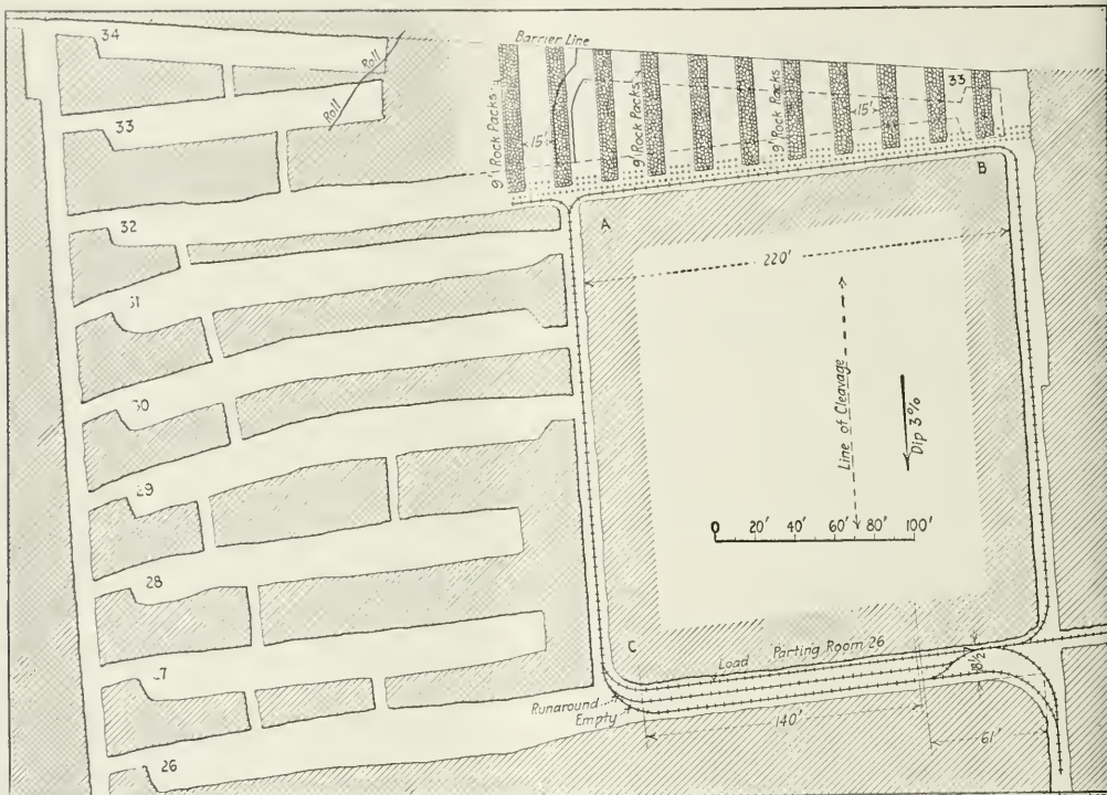
FIG. 1. SHOWS METHOD ADOPTED BY ONE COMPANY THAT CHANGED FROM ROOM-AND-PILLAR TO THE LONGWALL SYSTEM
