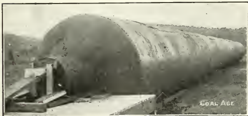
THE STEEL EXPLOSION GALLERY USED TO EXHIBIT THE EFFECT OF REPLACING BLACK POWDER BY PERMISSIBLE EXPLOSIVES
