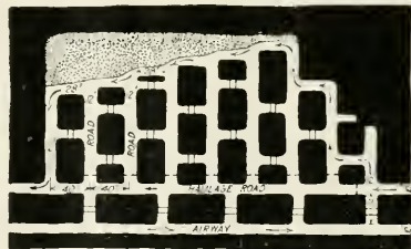
PLAN OF DRIVING DOUBLE STALLS
