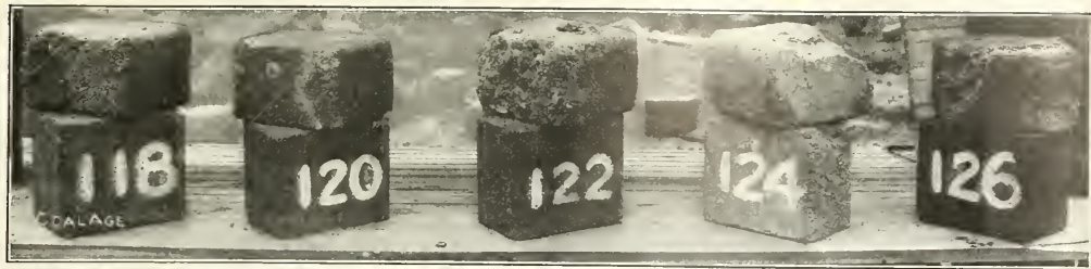
SAMPLES OF BRIQUETTES, SHOWING EFFECTS OF WEATHERING ON DIFFERENT TYPES
