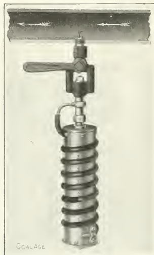
CROSS-SECTION OF PIPE WITH PITOMETER IN POSITION
