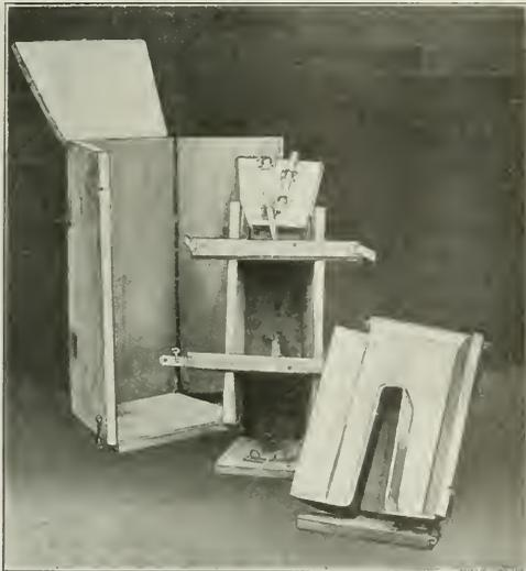
FIG. 2. FORMS USED IN CONSTRUCTION OF SWITCH BOX
