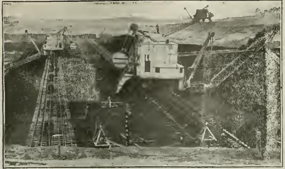
Brown Lignite Averaging Forty Feet in Thickness but Half Water Mined by Removing Sixty Feet of Overburden by Bucket Excavator—Central Power Plant Uses 7,000 Tons of Coal Daily
