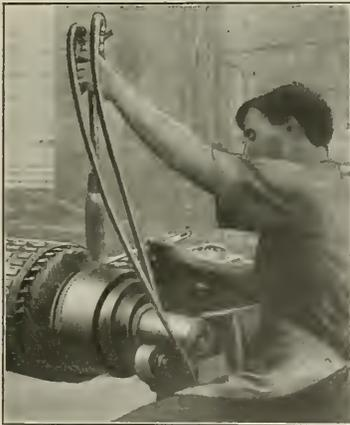
FIG. 1. SOLDERING AN ORDINARY COMMUTATOR
