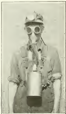
MASK IN POSITION The mask is used as subsidiary to oxygen breathing apparatus in mine-rescue work.
