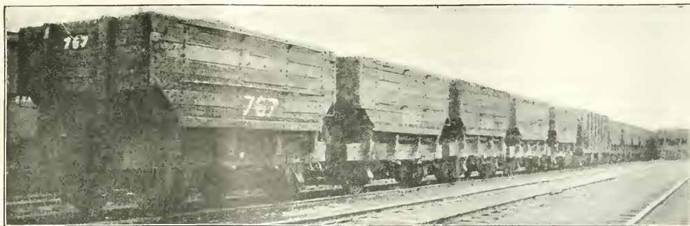
COAL-CAR EQUIPMENT OF SYDNEY & LOUISBURG R.R. IN YARDS OF PRINCESS COLLIERY These cars are of the type formerly used in the anthracite region of Pennsylvania
