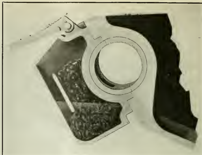
FIG. 3. OIL AND WASTE LUBRICATION APPLIED TO AN ARMATURE BEARING
