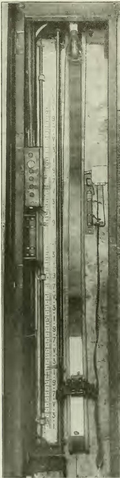
FIG. 3. AUTOMATIC DEVICE FOR REGULATING OIL-BINDER FEED
