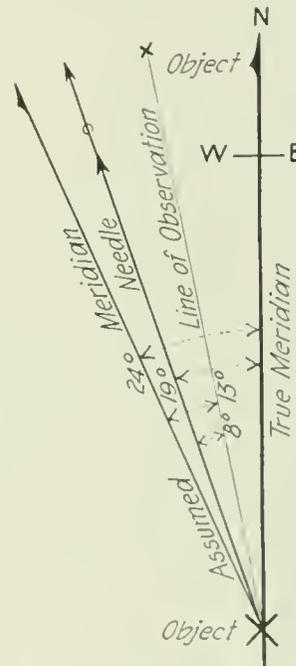
meridian is given by adding this bearing referred to the assumed meridian to its true bearing, which gives an angle of 24 deg. to the west of the true meridian, and the bearing of the assumed meridian is N 24 deg. W.
