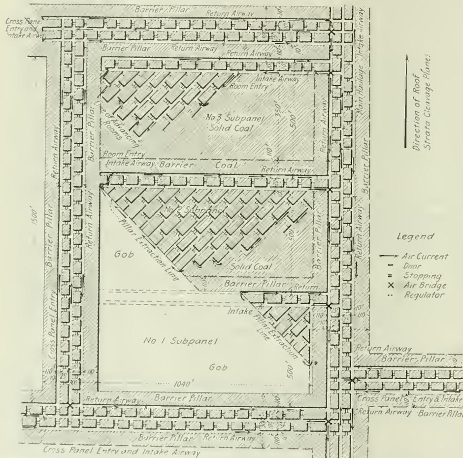
METHOD OF EXTRACTION BY SUBPANELS WITHIN A LARGER PANEL
