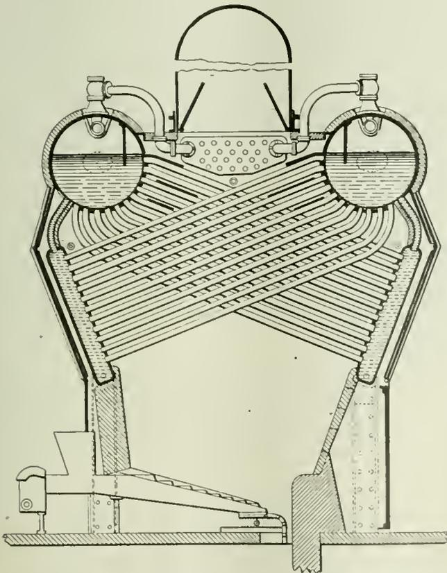
FIG. 1. VERTICAL SECTION OF BURTON BOILER
