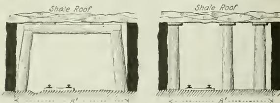
which shows both the method of supporting the roof with a boom resting on two posts and the plan I suggest of posting the entry.
