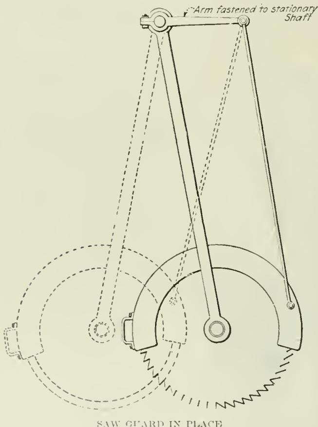
shield between the man operating the cutoff saw and the saw itself. When the saw is pulled forward by means of a lever a semicircular shield is thrown between the operator and the saw, just allowing sufficient space for the timber to pass between the saw and the shield. The accompanying diagrammatic illustration shows how this device operates.
