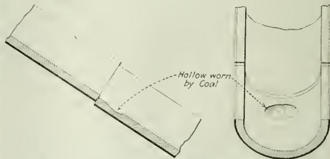
FIG. 2. LOWER LINING SECTION DEPRESSED
