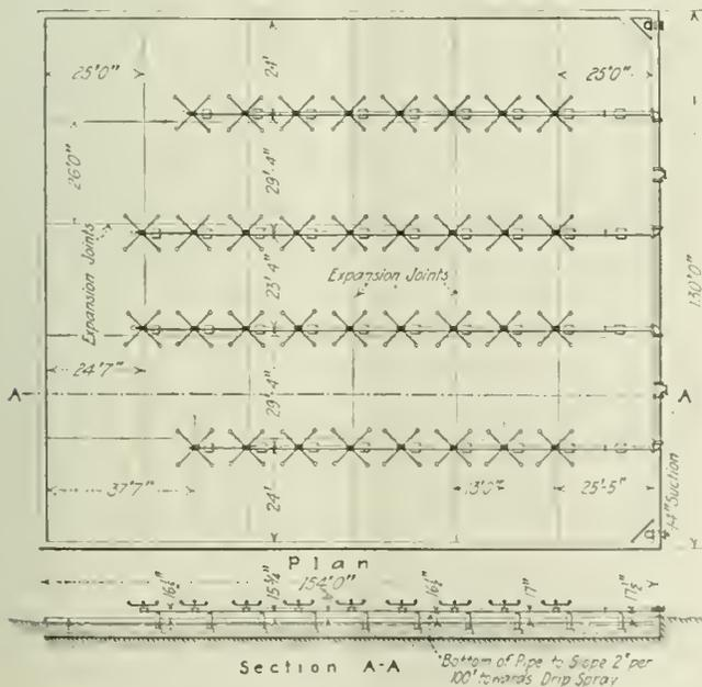
FIG. 5. PLAN AND CROSS-SECTION OF THE SPRAY POND
