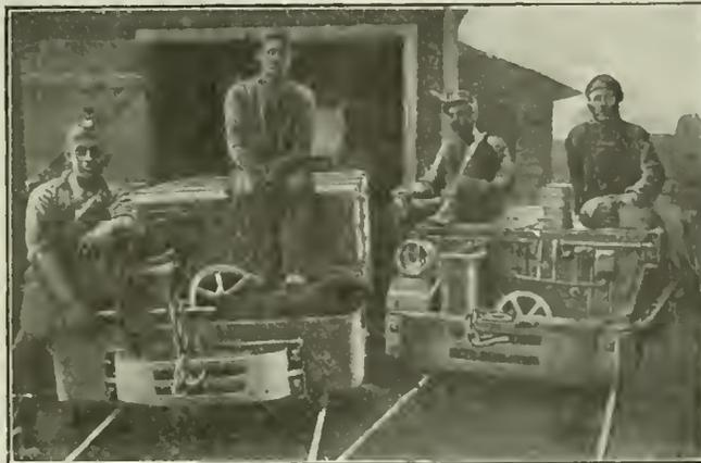
FIG. 1. TWO EARLY STORAGE-BATTERY LOCOMOTIVES
