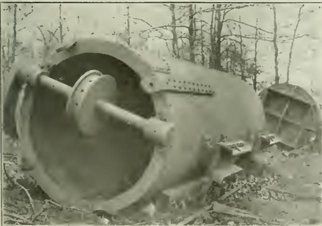
FIG. 2. PAIR OF BUCKETS FOR BAILING OUT SUMP
