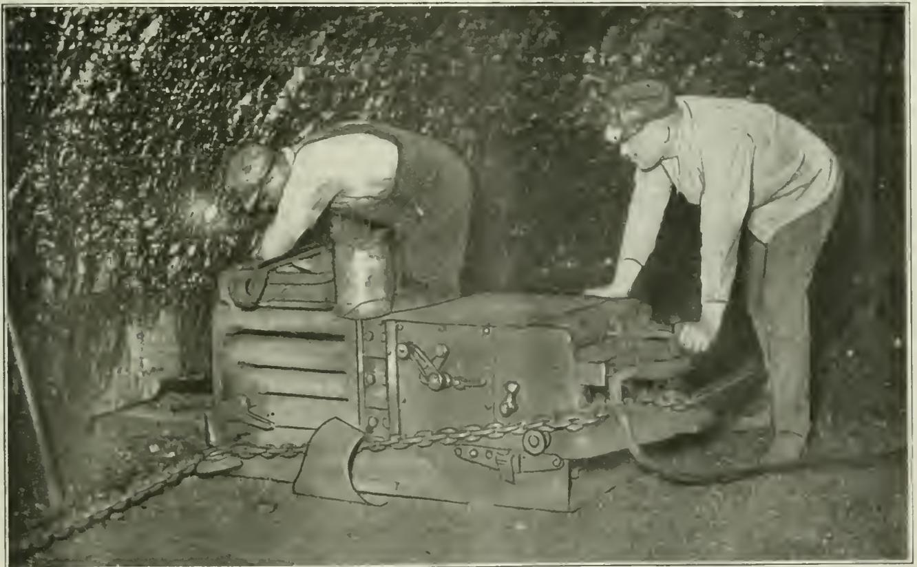
USING A SHORTWALL ALTERNATING-CURRENT COAL CUTTER IN A THICK SEAM
