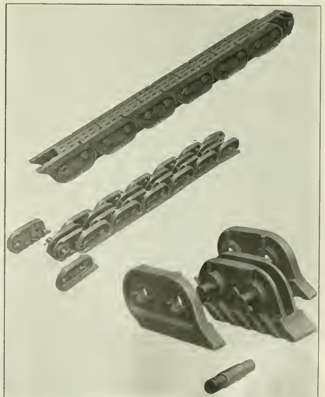
FIG. 2. DETAILS OF THE CONVEYING ELEMENTS
