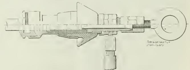
FIG. 3. POTHEAD SUSPENSION TERMINAL. Since the eye of this device is "alive," that is, at the cable potential, its support must be insulated. This is accomplished by means of a strain insulator.
