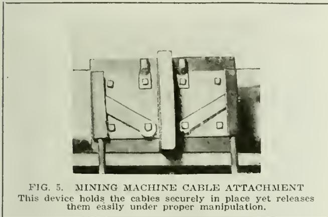
FIG. 5. MINING MACHINE CABLE ATTACHMENT
