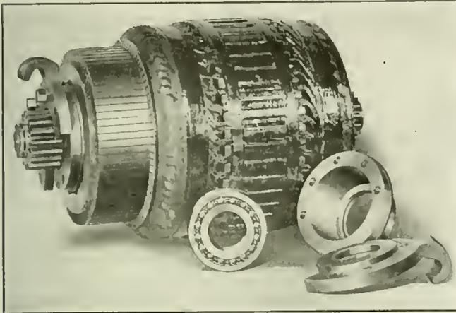
A LOCOMOTIVE ARMATURE AND ONE OF ITS BEARINGS
