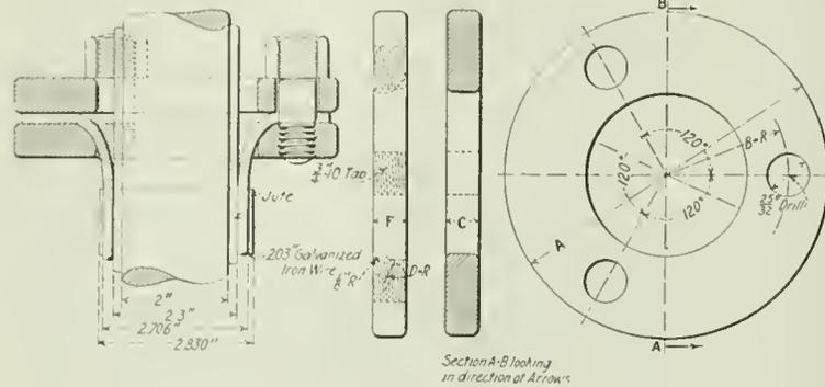
FIG. 9. DETAILS OF A FLANGE CABLE SUPPORT
