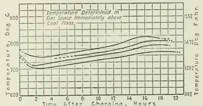
FIG. 6. TEMPERATURE OF VAPOR ABOVE COAL
