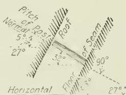
5 deg., the pitch of the post, or the angle it makes with the horizontal, is  $27 + 5 = 32$  deg., as indicated in the figure.
