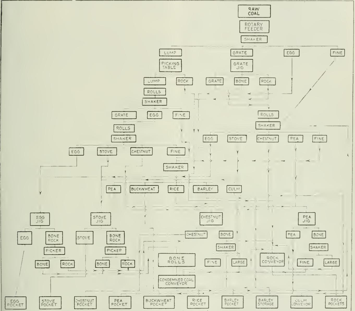
FLOW SHEET OF THE REMODELED OLD FORGE BREAKER
