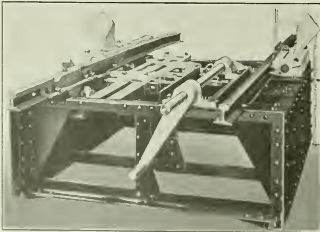
SUBSTANTIAL MOUNTING MAKES THE FEEDER RIGID. The horns are opened by the descending cage and close when it leaves the landing.
