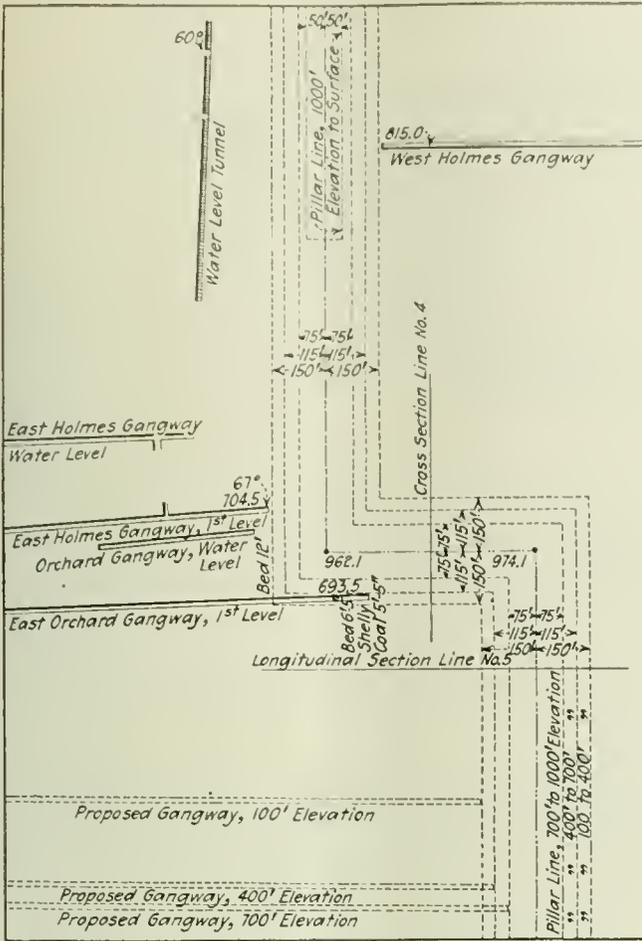
FIG. 11. A BARRIER PILLAR ESTABLISHED BETWEEN ADJOINING MINES
