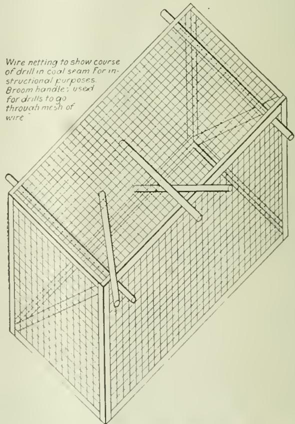
Wire netting to show course of drill in coal seam for instructional purposes. Broom handle, used for drills to go through mesh of wire.
