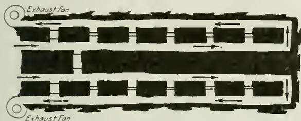
doors are so arranged in the mine that they can be readily adjusted to turn the two circulations into two or more splits ventilating the entire mine.
