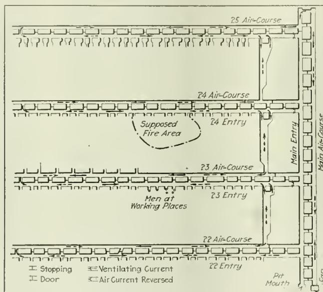
FIG. 1. DIAGRAM OF A MINE VENTILATING SYSTEM
