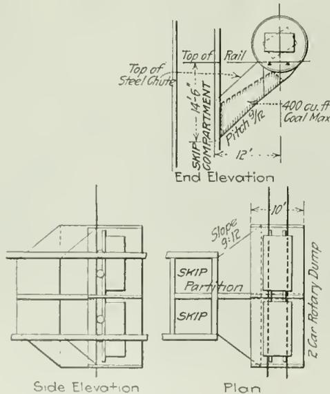
FIG. 1. PROPOSED SHAFT STATION AT PENNSYLVANIA SHAFT
