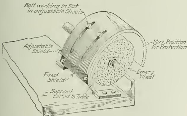
As emery wheels have a tendency at times to break and fly to pieces the master mechanic of the Burnside Colliery of the Philadelphia & Reading Coal & Iron Co. near Shamokin, Pa., has designed a special adjustable shield to cover such wheels.
