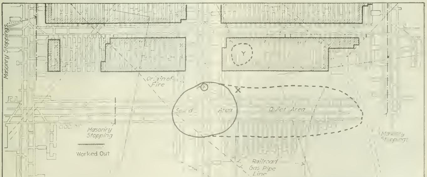
FIG. 3. DETERMINATION OF A FIRE AREA IN A MINE HAVING 300 FEET OF COVERING
