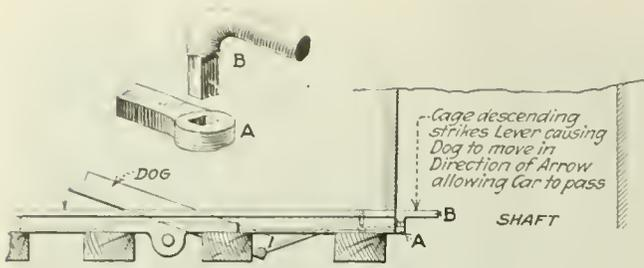
FIG. 4. CAGE-OPERATED CAR STOP OR DOG
