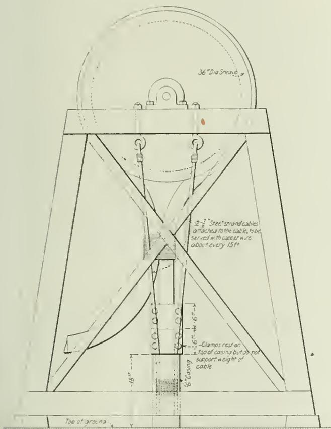
FIG. 7. SUSPENDING A CABLE FROM A SHEAVE
