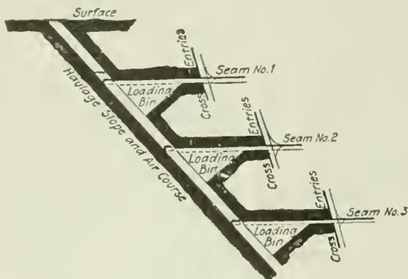
SHOWING STEEP HAULAGE SLOPE AND GANGWAY LEVELS IN THREE SEAMS
