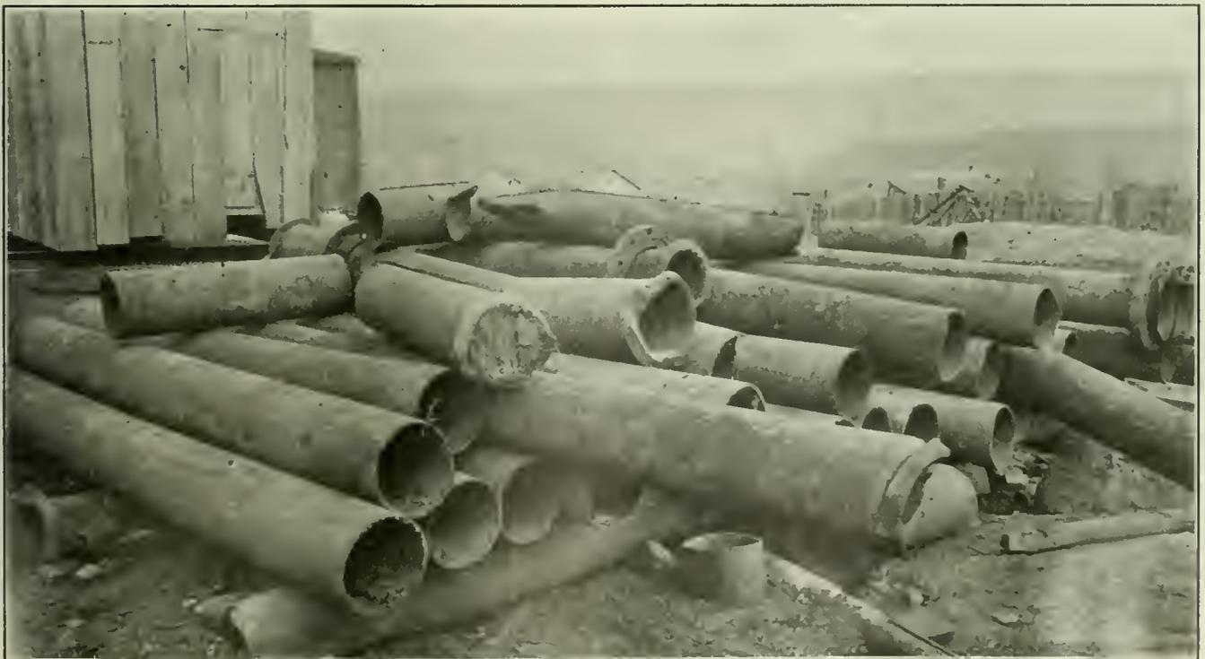
**FIG. 9. SECTIONS OF THE 8-IN. AIR LINE THAT FELL DOWN THE SHAFT**
