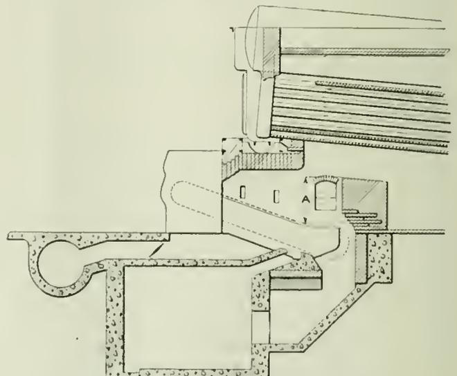
**FIG. 4. SECTIONAL ELEVATION OF STOKER**
