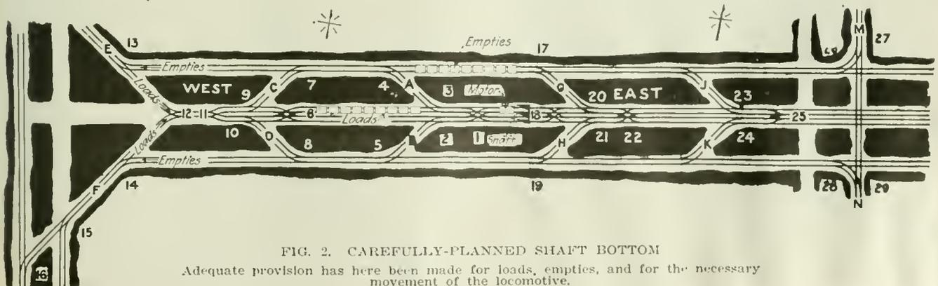
FIG. 2. CAREFULLY-PLANNED SHAFT BOTTOM
