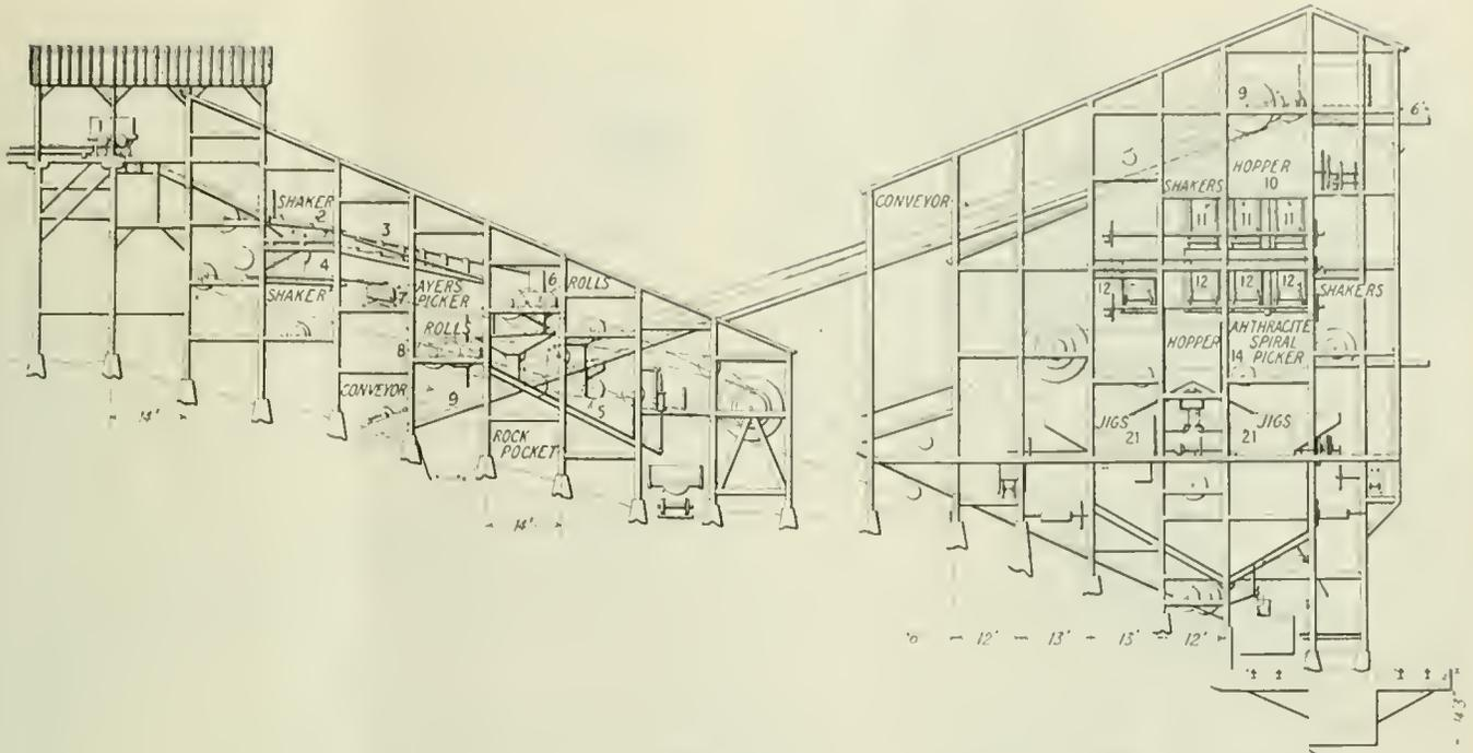
FIG. 1. CROSS-SECTION OF THE ROCK-SEPARATOR HOUSE AND BREAKER
