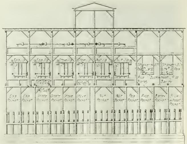
FIG. 1. CROSS-SECTION SHOWING SHAKERS, JIGS AND POCKETS
