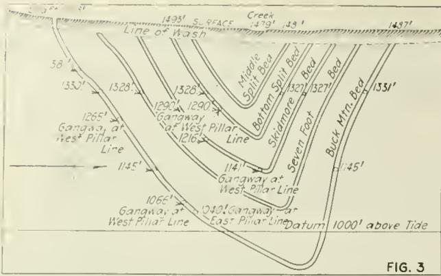
FIG. 3. VERTICAL SECTION ON THE LINE OF THE BARRIER PILLAR SHOWN IN FIG. 2
