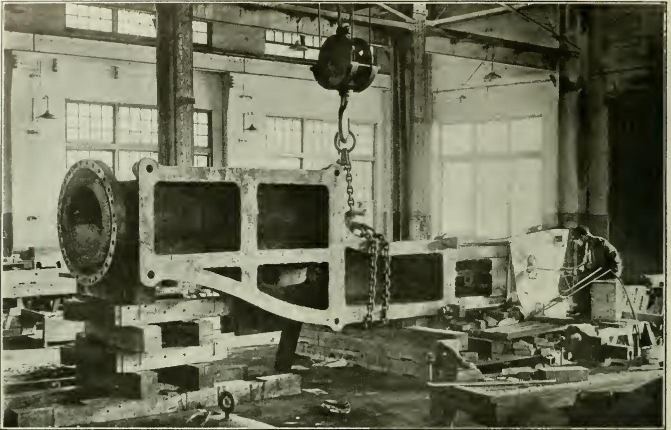
FIG. 4. WELDING THE ENGINE FRAME IN THE SHOP
