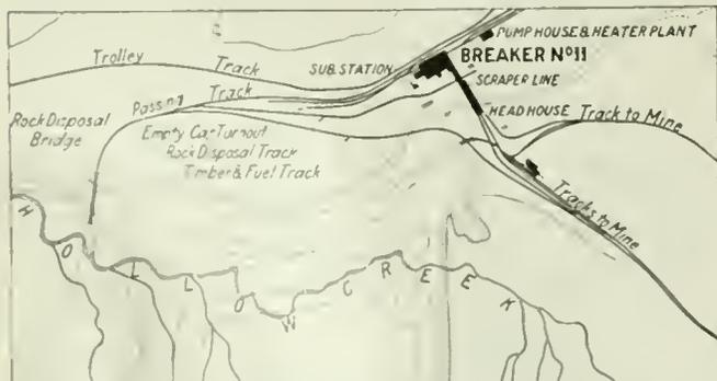
FIG. 3. PLAN OF THE BREAKER SURROUNDINGS Showing the relation of the yard tracks to the breaker, and the tracks by which buildings, tracks, roads, rock and the like is disposed of and timber and fuel delivered.
