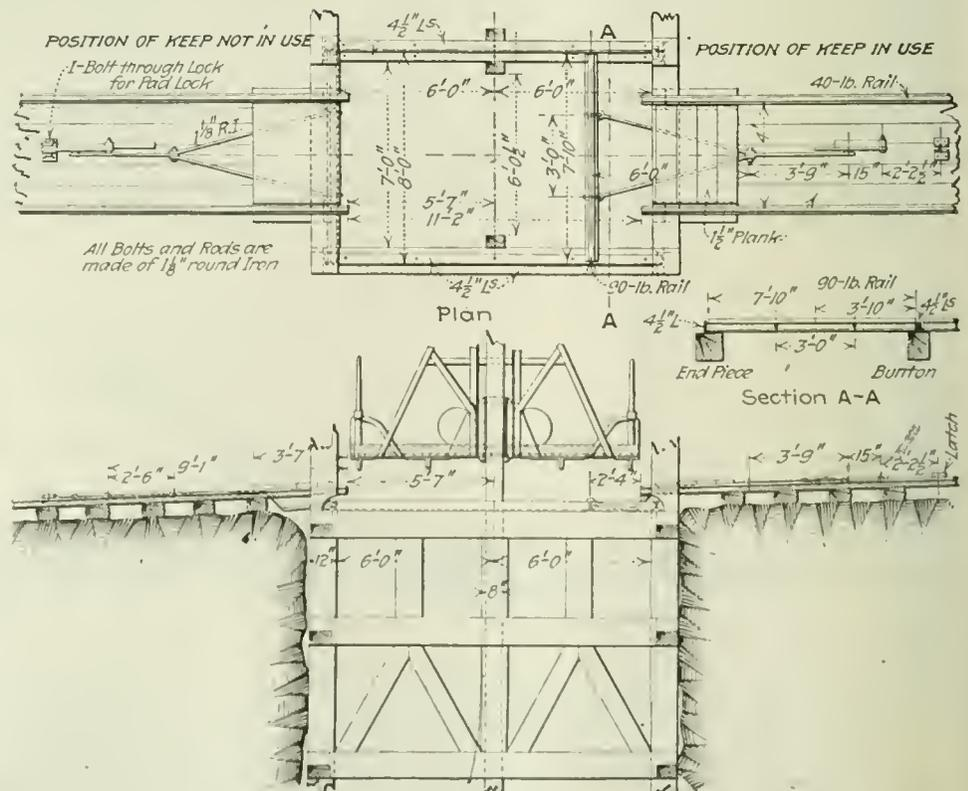
ously described are only 10 ft. wide. Fig. 3 shows the plans of this shaft station in detail.
