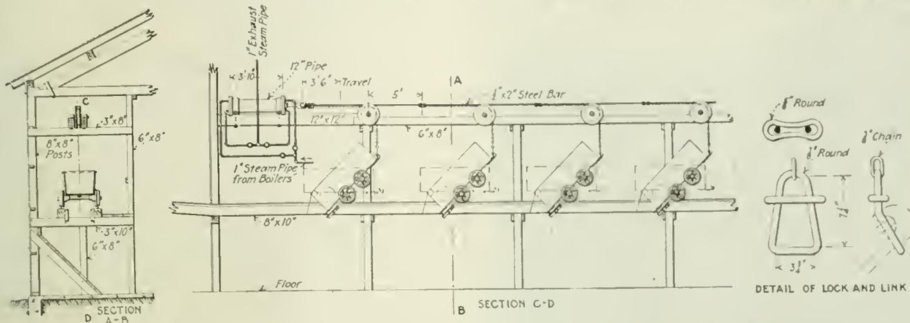
CONSTRUCTION DRAWING OF THE CAR DUMPING MECHANISM. DETAILS OF LOCK AND LINK ON RIGHT
