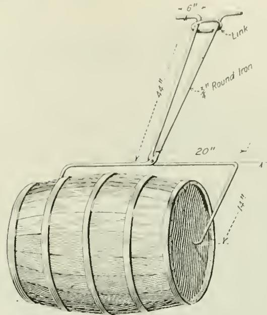
HOW THE BARREL TONGS ARE USED
