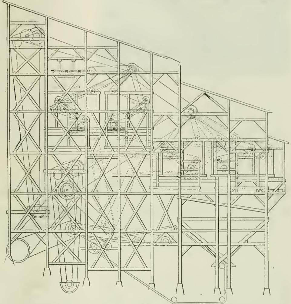
FIG. 5. ARRANGEMENT OF MACHINERY IN OLD WASHER
