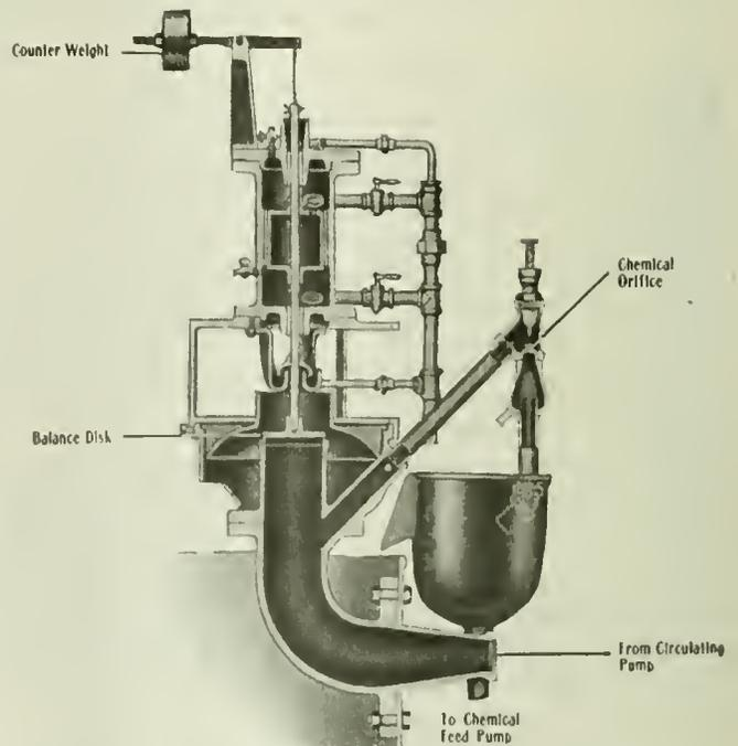
FIG. 2. CHEMICAL PROPORTIONER This device, accurately, automatically and in proper proportions, feeds chemicals to the softening apparatus.
