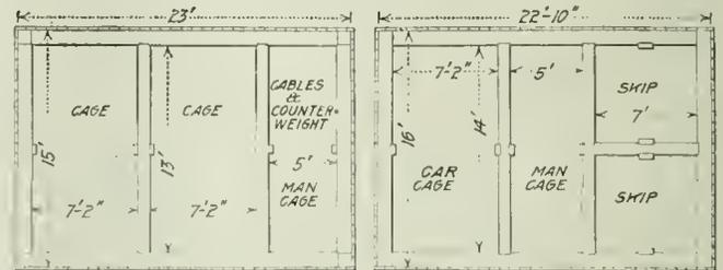
FIGS. 2 AND 3. CROSS-SECTIONS OF THE RICHARDS AND PENNSYLVANIA SHAFTS
