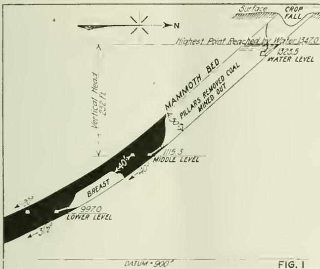
FIG. 1. SECTION THROUGH KEHLEY RUN MINE
