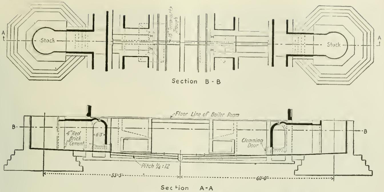
FIG. 6. PARTIAL PLAN AND CROSS-SECTION AT CENTER LINE OF STACKS
