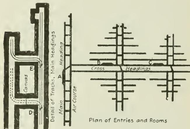
headings and rooms is shown on the right; while an enlarged detail plan of the main heading and tracks is shown on the left.
