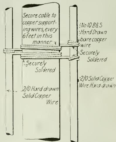
FIG. 6. A POWER CABLE AND ITS SUPPORTING WIRES
