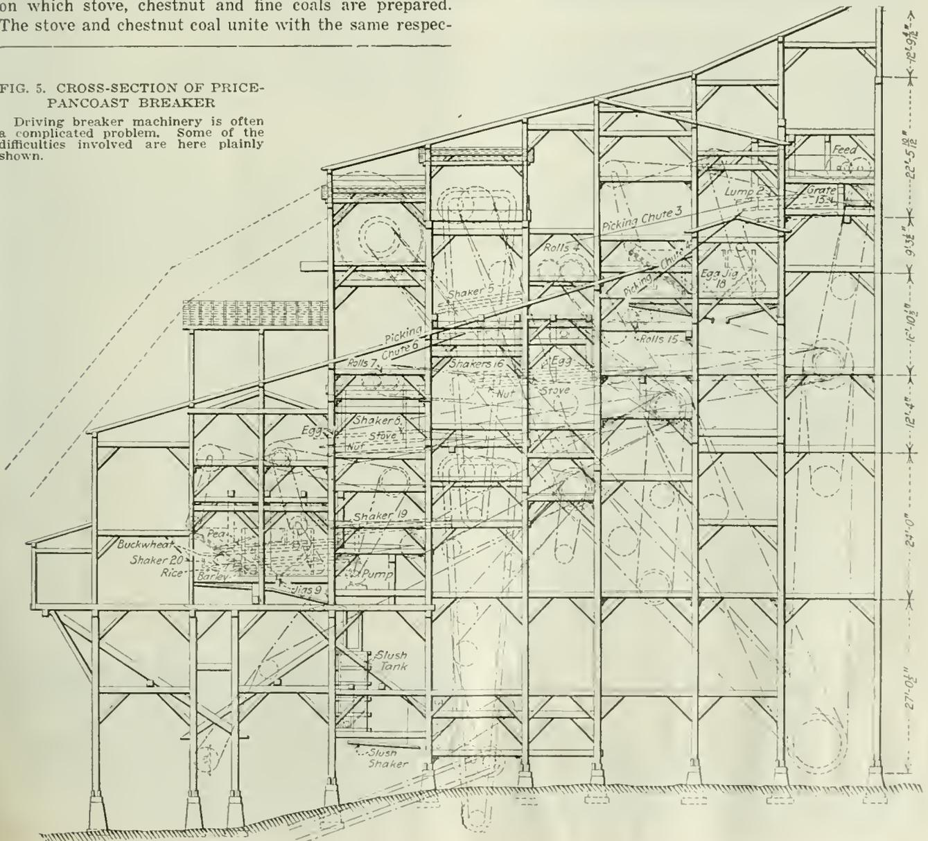
tive sizes from shakers 8 and 16 and are treated with them as has already been described. The fine coal from shaker 18 is passed to a four-decked shaker (20) on which is also treated the fine material from shakers 8 and 16. Five sizes are made on this shaker—pea, buckwheat, rice, barley and culm. The pea, buckwheat, rice and barley pass directly into their respective pockets, while the culm is returned to the mine for filling purposes.
