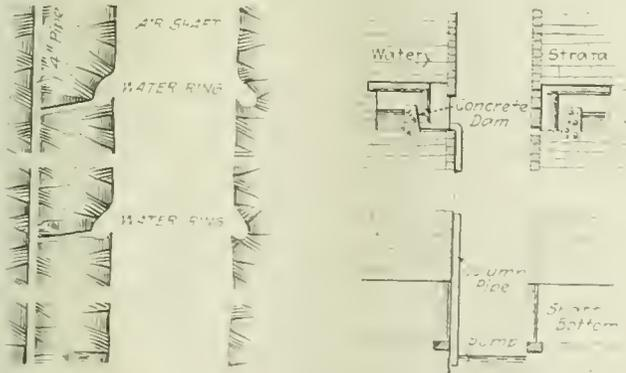
SHOWING TWO TYPES OF WATER RINGS FOR DRAINING A WET SHAFT
