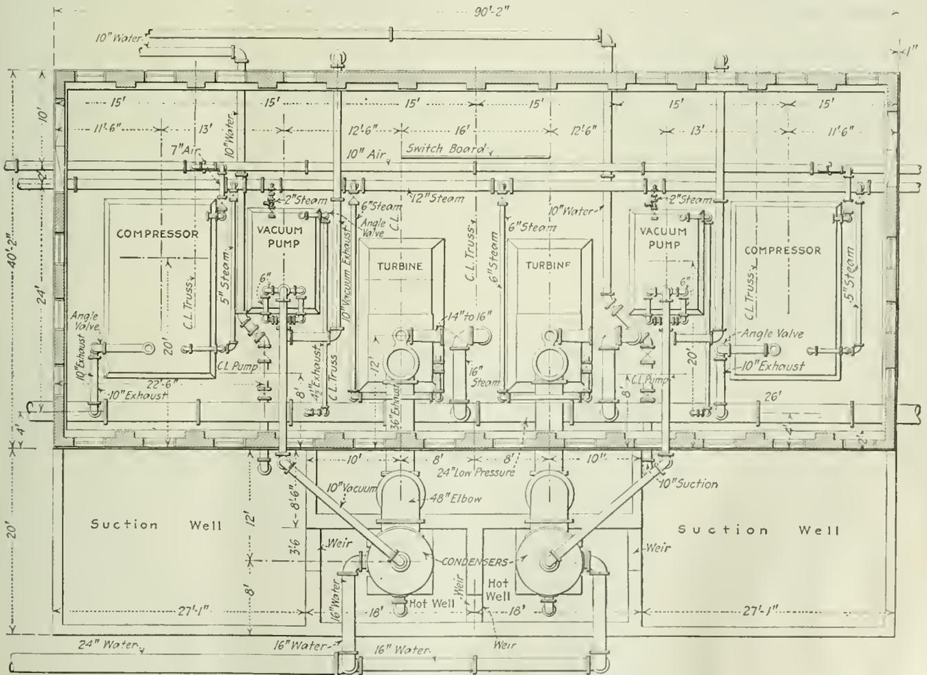
FIG. 1. PLAN OF THE PRICE-PANCOAST POWER HOUSE, SHOWING ARRANGEMENT OF MACHINERY
