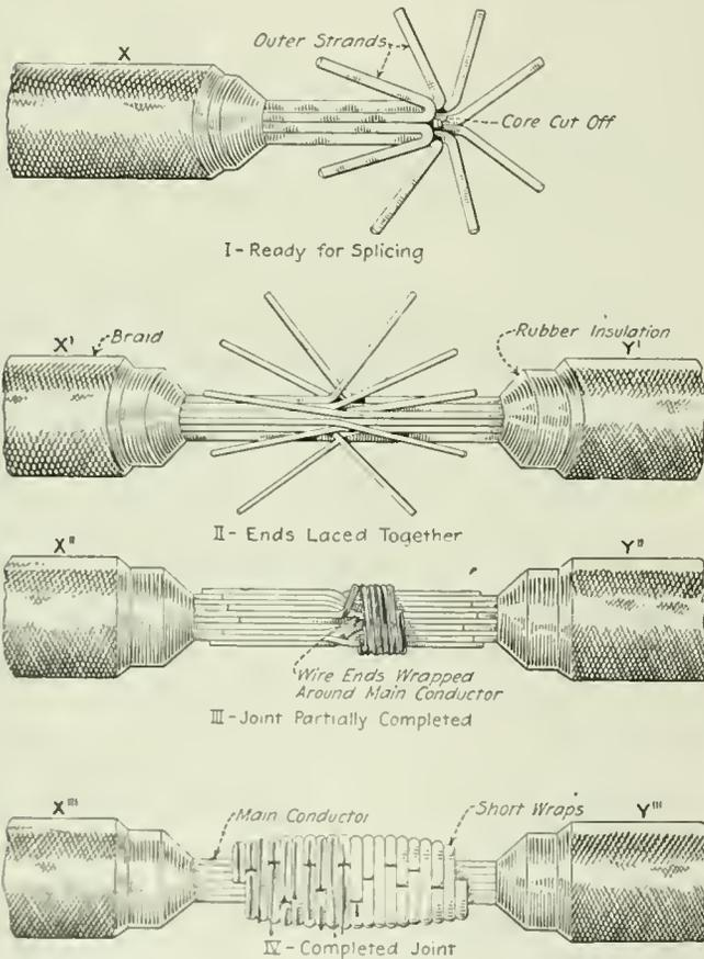
SPlicing A STRANDED CONDUCTOR
