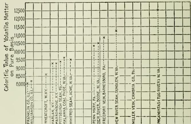
FIG. 3. CALORIFIC VALUES OF VOLATILE MATTER FOR TYPICAL COALS ON THE "PURE COAL" BASIS
