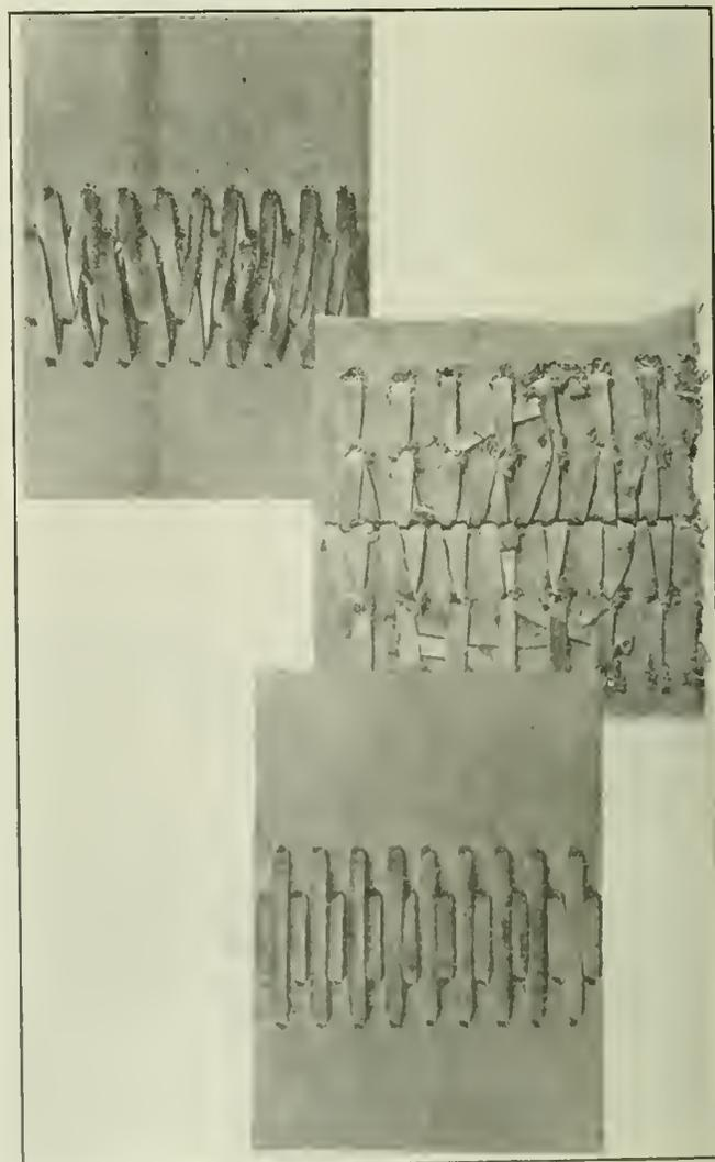
**CORRECT AND INCORRECT METHODS OF LACING A BELT**
