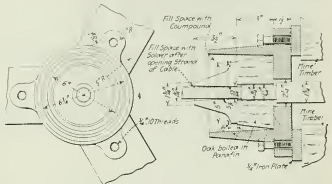
FIG. 2. INSULATED CAST-IRON BLOCK SUSPENSION. This is a modification of C, Fig. 1, adapting it to cables carrying appreciable voltage. The cast-iron block into which the cable is soldered is insulated from its surroundings.
