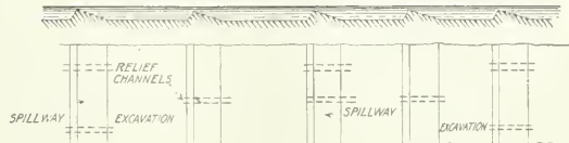
Plan FIG. 9 LONGITUDINAL SECTION OF RIVER WITH SUGGESTED EXCAVATION LEAVING SPILLWAYS TO ADMIT OF MAXIMUM PRECIPITATION AND MINIMUM OF SCOUR
