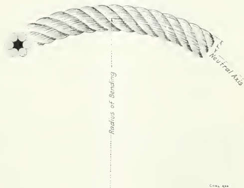
FIG. 2. DIAGRAM SHOWING ARC OF ROPE, NEUTRAL AXIS, RADIUS OF BENDING AND RADIUS OF ROPE
