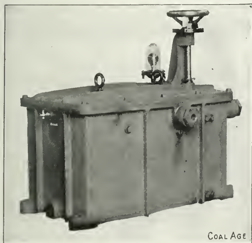
FIG. 1. OIL-IMMERSED STARTER AND CONTROLLER
