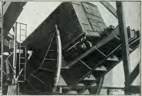
INTERIOR VIEW OF THE TURBO-GENERATOR HOUSE AND THE CRADLE BOX-CAR LOADER
