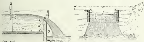
LONGITUDINAL CROSS-SECTION AND FRONT VIEW OF WEIR, SHOWING IMPORTANT DIMENSIONS
