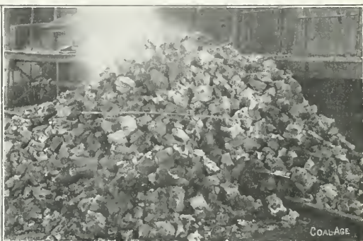
COKE AFTER BEING PUSHED FROM THE OVEN. IT IS NOT LARGE AND COLUMNAR LIKE BEEHIVE COKE
