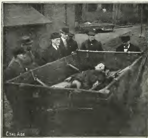
A SPRING STRETCHER FOR USE IN A MINE CAR
