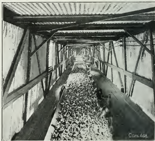
COAL PASSING FROM TIPPIE TO RESCREENER ON RUBBER BELT
