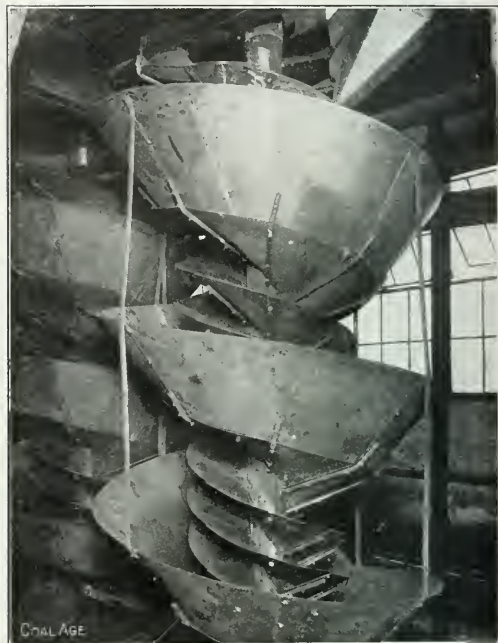
ONE OF THE TWENTY-EGHT SPIRALS BY WHICH DIRT AND LOW-GRADE COAL ARE REMOVED
