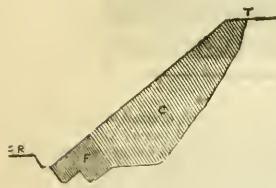
Section of Gravel counterfort, and footing, introduced into a Slip.
