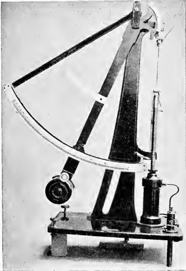
FIG. 50. SCHOPPER TENSILE MACHINE
