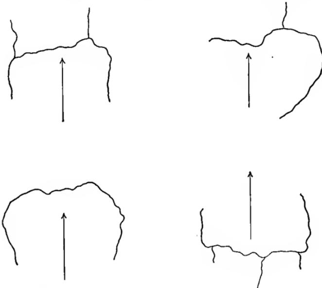
FIG. 43. LINES OF RUPTURE IN MULLEN TEST
