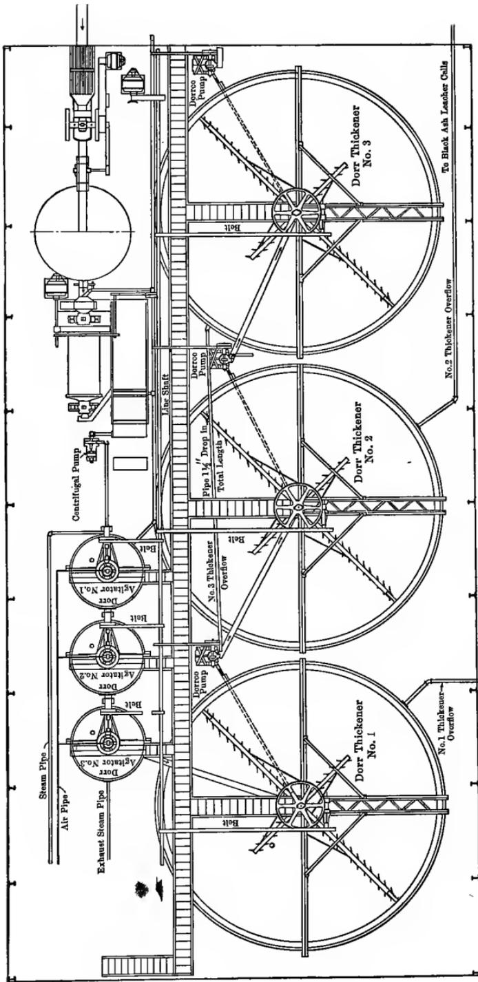
FIG. 9. PLAN OF CONTINUOUS CAUSTICIZING PLANT
