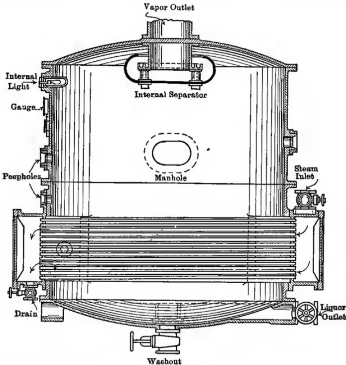
FIG. 19. ZAREMBA EVAPORATOR VERTICAL CROSS SECTION OF ONE EFFECT
