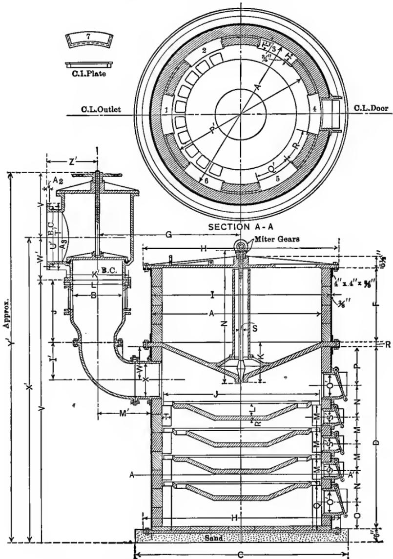
FIG. 24. VESUVIUS SULPHUR BURNER, SECTIONAL VIEW
