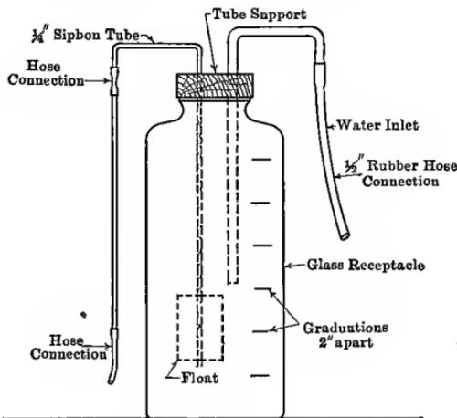
FIG. 38. APPARATUS FOR DETERMINING GRIT IN FILLERS
