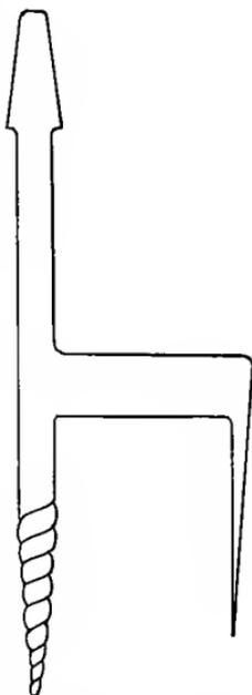
FIG. 40. CUTTER FOR SAMPLING PULP
