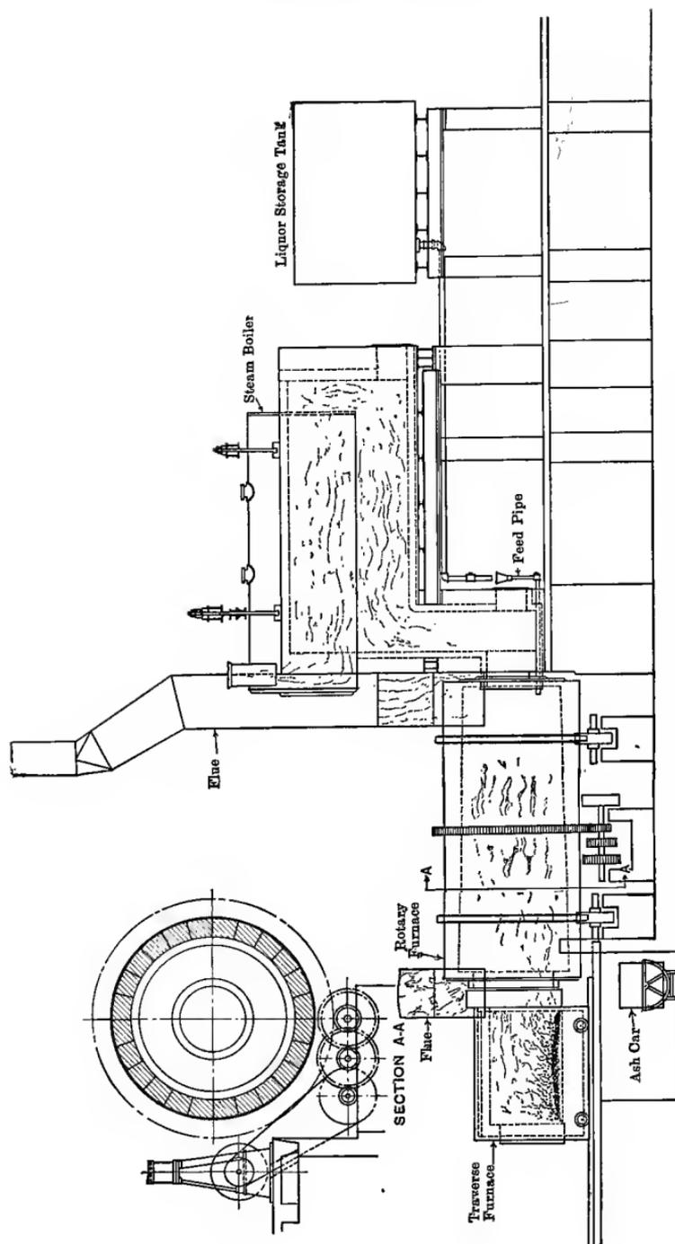
FIG. 20. SODA RECOVERY OR BLACK ASH FURNACE
