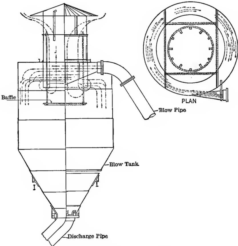
FIG. 16. BLOW TANK OR SEPARATOR
