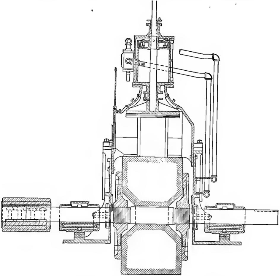
FIG. 32. THREE-POCKET GRINDER SECTIONAL ELEVATION
