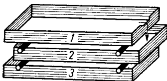
FIG. 79. Pans for crystallization of TNT (Pascal [5]).
