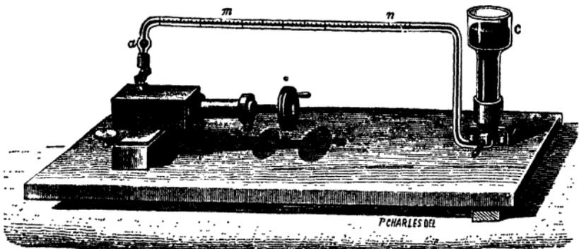
FIG. 8.—Apparatus of Bonnier and Mangin, for analysis of gases given off by plants. *c*, Reservoir of Mercury; *m n*, graduated tube; *v*, screw of piston, which enables the gas to be drawn into the graduated tube and measured; and after it the potash and pyrogallic solutions successively, each being thoroughly brought into contact with the gas in the dilatation *a*.
