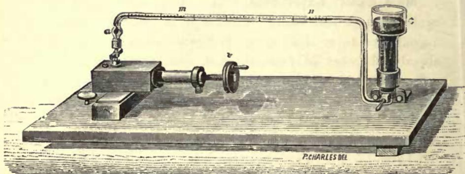
FIG. 8.—Apparatus of Bonnier and Mangin, for analysis of gases given off by plants. *c*, Reservoir of Mercury; *m m*, graduated tube; *v*, screw of piston, which enables the gas to be drawn into the graduated tube and measured; and after it the potash and pyrogallic solutions successively each being thoroughly brought into contact with the gas in the dilations *a*.
