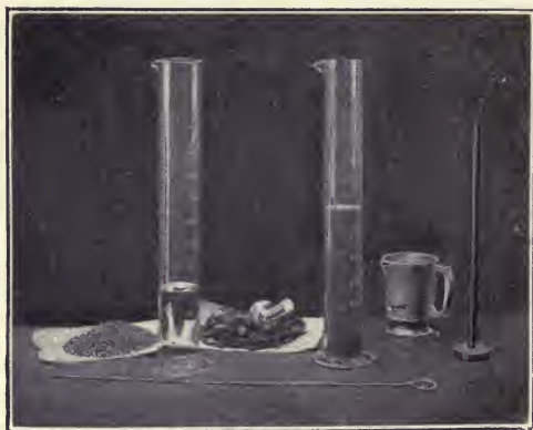
FIG. 28.—Apparatus for determining proportion of voids in aggregates.
