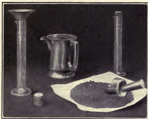
FIG. 27.—Apparatus for determining whether aggregates require washing before use. (By courtesy of the Associated Portland Cement Manufacturers, Ltd.)
