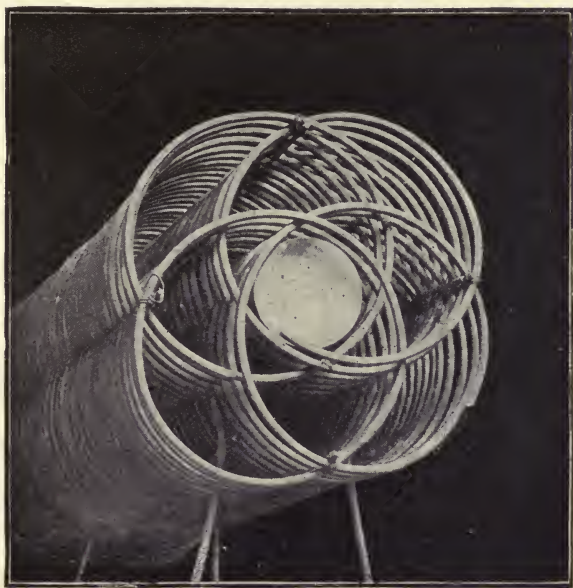
FIG. 55.—Core with Anchored Spirals. End View. ( Courtesy of Reinforced Metal, Ltd. )
