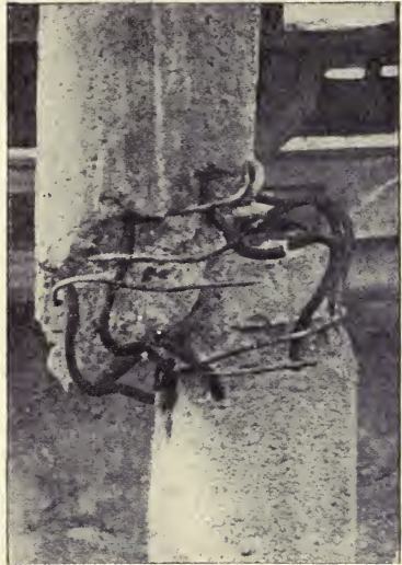
FIG. 77.—Overloaded Column, with Insufficient Longitudinal Reinforcement.
