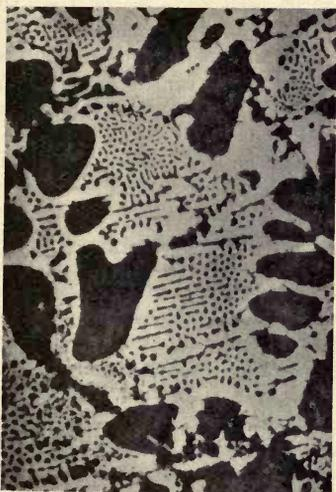
FIG. 54.—Showing process of balling-up of constituents of eutectic (sample F, 0.23 per cent. sulphur). Magnified 120 diameters.
