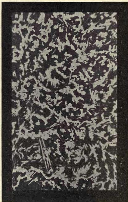
FIG. 110.—White Cast Iron. Etched.
