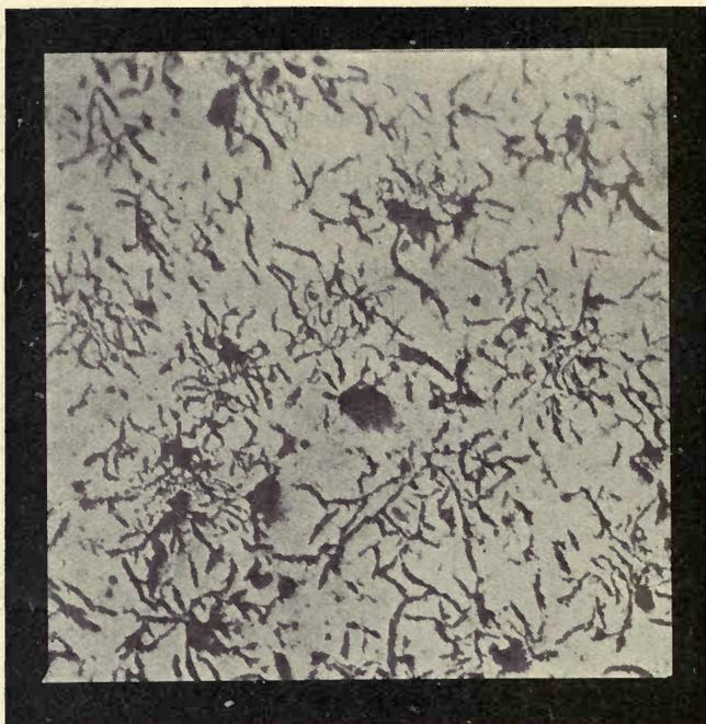
FIG. 105.—Baffle plate, heated to 800° C.
