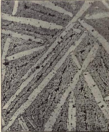
FIG. 60.—Iron-carbon-sulphur alloy (4·37 per cent. carbon).
