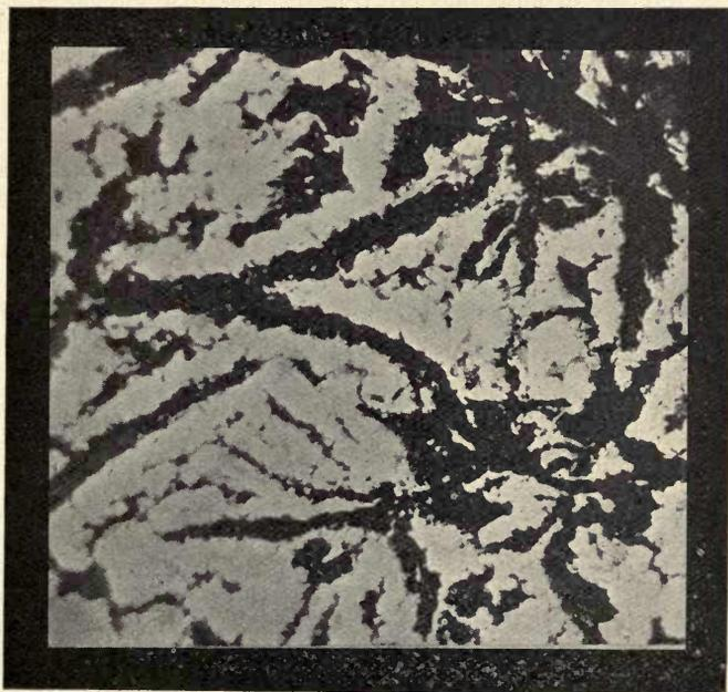
FIG. 109.—Stove pipe, heated for period at 700°-750° C.
