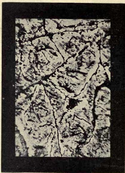
FIG. 21.—Grey cast iron. Etched  $\text{HNO}_3$ . Magnified 52 diameters.
