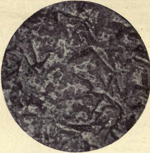
FIG. 5.—Etched picric acid in alcohol. Magnified 60 diameters.
