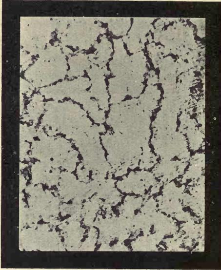
FIG. 24.—Ferro-silicon. 31.2 atom per cent. silicon =  $\text{Fe}_2\text{Si}$ .
