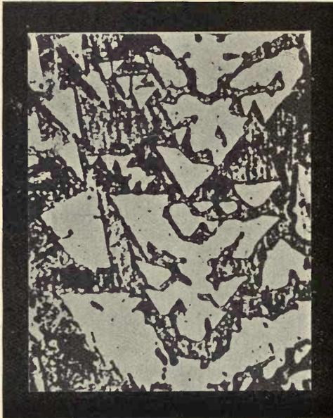
FIG. 25.—Ferro-silicon. 42.4 atom per cent. silicon showing  $\text{Fe}_2\text{Si}$  in eutectic matrix.
