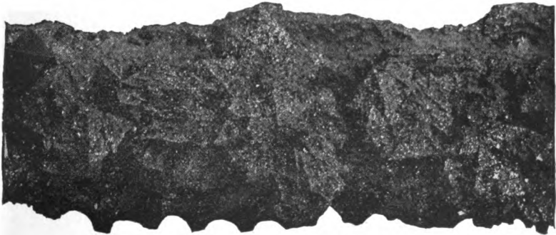
FIG. 6.—Aggregations of Octahedral Crystals of Cast Iron.
