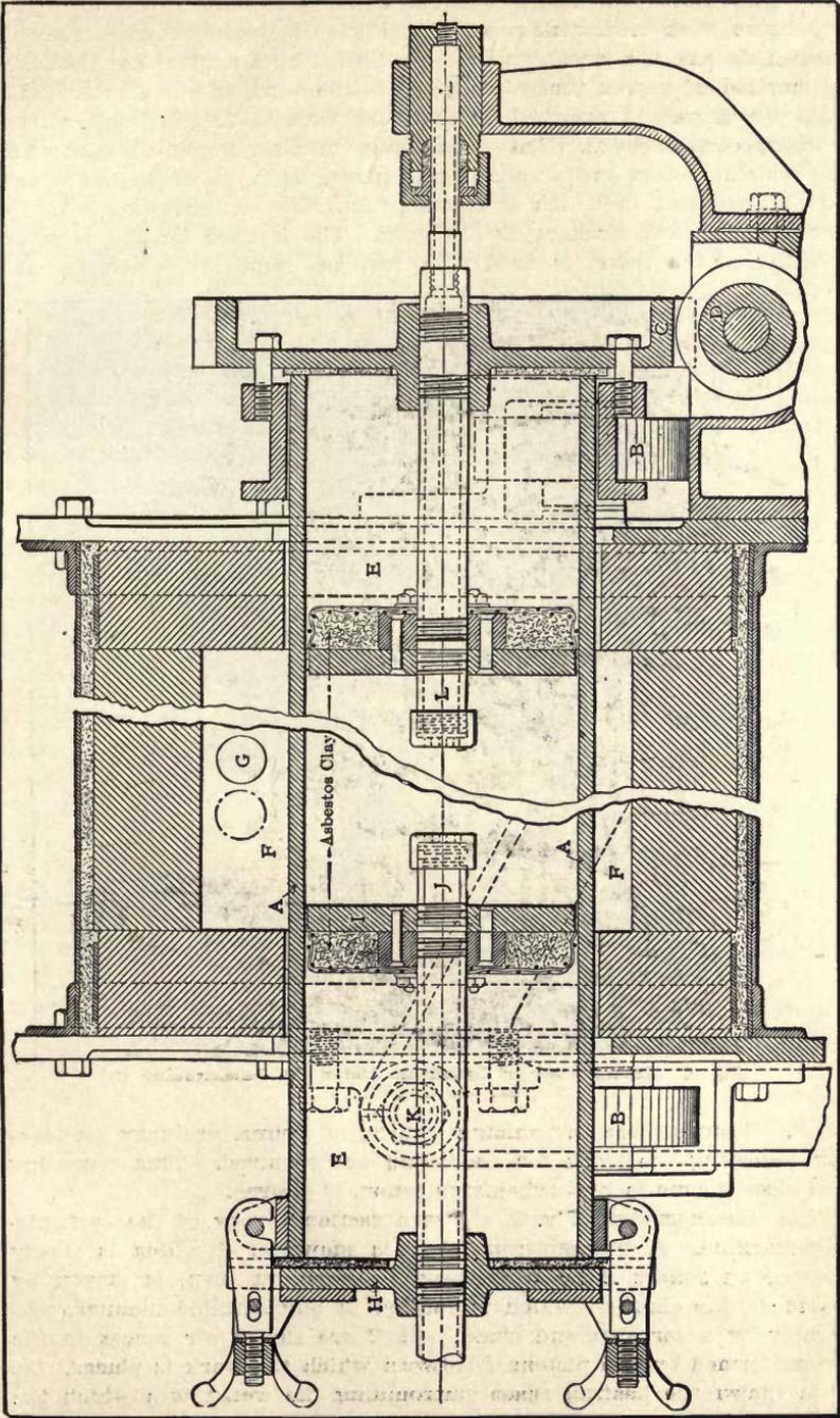
Fig. 3. Revolving Cylindrical Retort brought out by the American Gas Furnace Company for Casehardening by Gas
