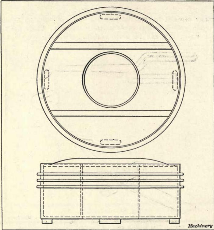
Fig. 3. Large Circular Box with Hole in Center for the Circulation of the Gases of Combustion
