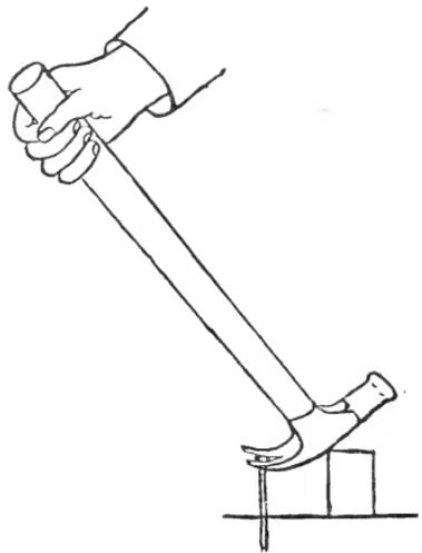
partial drawing commences, and each partial drawing should be about  $\frac{1}{2}$  in. to  $\frac{5}{8}$  in. in amount, in order not to bend the nail, or strain the hammer handle. I have seen workmen break hammer handles and nails resist drawing when neither would have occurred had the above simple direction been followed. Mark 10 off from 100 for every bent nail.
