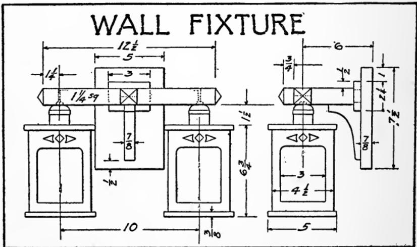
are now in order, the smaller one being mortised to match the central arm. The curved bracket remains to be shaped up, after which the whole may be put together, using glue and a few nails so placed as to be invisible. The completed wall
