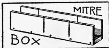
hold it tightly against one side and then work the saw back and forth in the slits cut in the sides.
