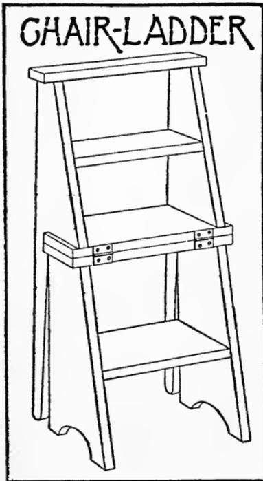
after which secure them firmly in place. The step, half-way between the seat and the floor, is now to be placed, and the back half of our chair is complete. To finish the front half it is only necessary to make the other half of the seat-board and the lower step, and with them connect the two front portions of the sides previously prepared. When the two halves are now placed together, they
