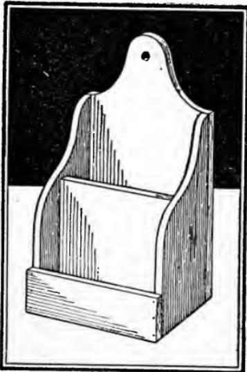
The two side pieces should be about a half inch thick, and the back, front and center piece about three-eighths. To get a pattern for the sides, mark out four rows of one-inch
