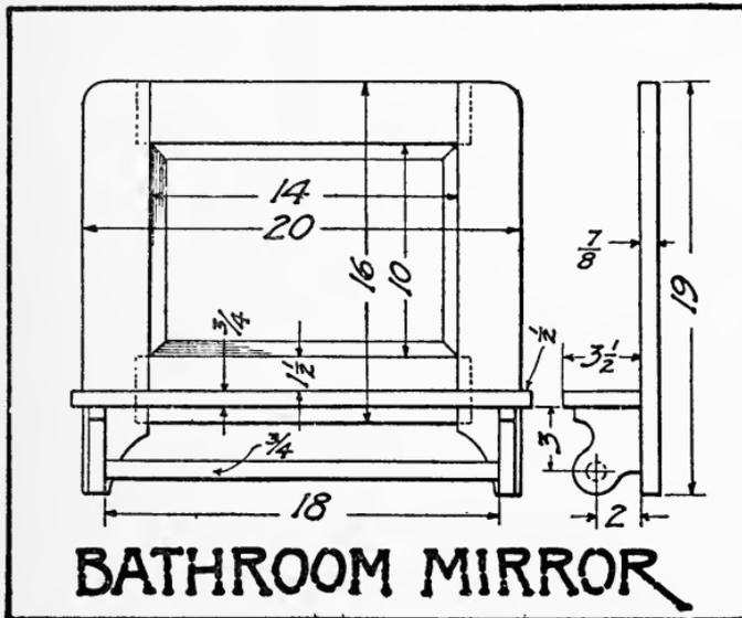
out the back edges around the opening to hold the glass. The vertical pieces, it will be noted, extend downward to hold the shelf-brackets, which may now be made ready. If a roller-towel is to be used, one bracket must have a hole clear through, so that the roller may be withdrawn. It then remains only to make the shelf and assemble the parts. Glue the mortises; fasten the other pieces with screws from behind, and glue.
