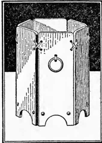
mark one board from another, but use the compasses on each one separately. Six quarter-inch holes must now be bored in each piece as indicated, due care being taken not to tear off any splinters.
