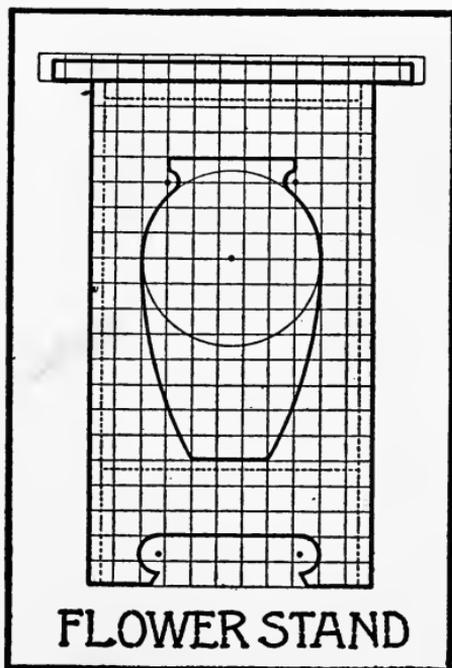
with a sharp pencil. Saw out the large opening, and shape up the feet, all very carefully, so as not to tear off any splinters and thus spoil the outline. Trim off the edges, and smooth with sandpaper, after which the four sides may be nailed together.
