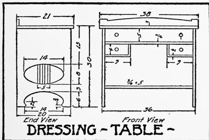
snugly fit in the three slats in each end opening, securing each slat with glue and a wire nail at each end. It now only remains to make and fit the drawers—and our table is complete.
