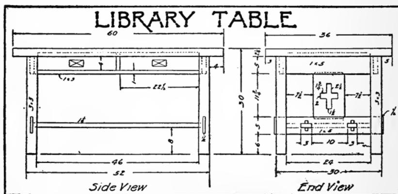
inch boards, reinforced around the edges with a narrow board, to give it a massive appearance. The top was then covered with a dark shade of imitation leather, fastened with large-head, dull-finished brass nails.
