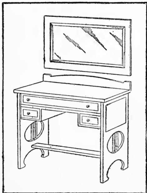
foot-rail are to be trimmed up to their respective widths and to the same length. As soon as the top has been made ready, the two sides are to be set up and connected. On account of the direction of the grain in that portion of each side just below the elliptical openings,
