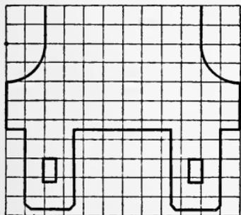
The panels are of three-eighths-inch board, in which is cut the mission cross. These panels should be mortised above and below into the crosspieces for a distance of about one-fourth of an inch. The entire
