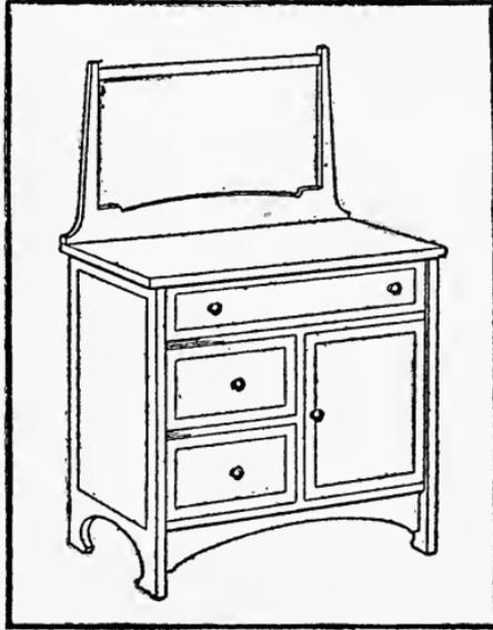
After closing in the back, it only remains to fit on the door and to make the three drawers. If desired, the two smaller drawers may be omitted and a door substituted, thus simplifying the construction somewhat.
