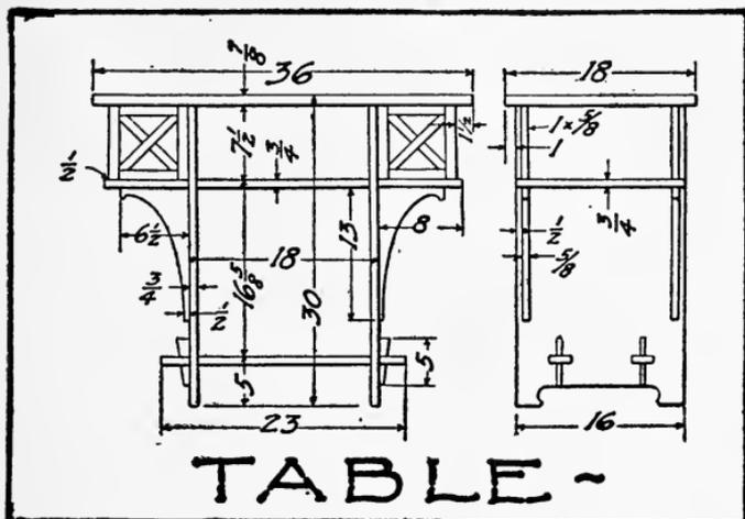
Make the outer frames of the four rectangular panels first, and see that they fit in place before going further. Place one diagonal and then put in the halves of the remaining one.
