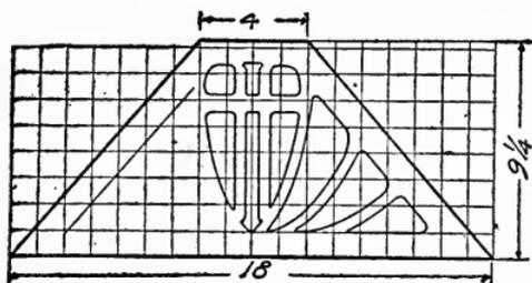
Quite the most difficult feature will be the construction of the shade. The dimensions of one of the four sections are given in the accompanying sketch. Accurately lay out the pattern on a sheet of paper and transfer it to each of the four pieces, which may be of several materials. If wood is used, the cross grain at the top and bottom must be reënforced with strips glued on the inside. Considerable care will be necessary in fitting the corner seams and in sawing out the pattern.
