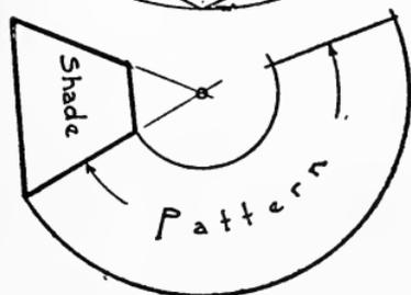
pattern: on a large sheet of paper draw out the shade and then continue the slanting side lines up to an intersection; with this point as a center draw a large and a small circle as shown, after which it only remains to step off a distance along the larger arc equal to the circumference
