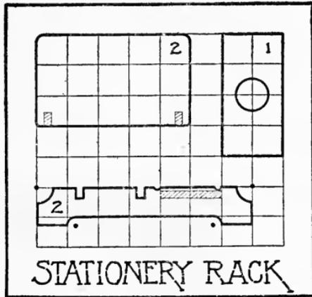
the sides are perfectly parallel and stand straight. It now only remains to find something round for a cover for the ink pot. If a suitable cover cannot be found, simply cut out a neat disc of thin wood and fasten a small knob on top in the center.
