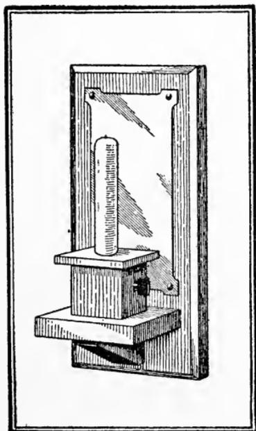
In the electric candle sconce illustrated an ordinary key socket, such as is used on drop lights, is neatly boxed in with the key projecting from one side. The box is then mounted on a small shelf in front of a piece of polished brass or copper to serve as a reflector. When the woodwork is neatly finished and a frosted candle-shaped electric lamp is used, the effect
