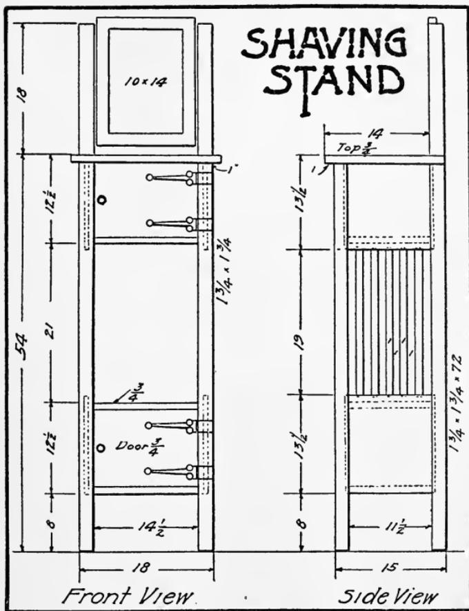
tie sides connected together, after which the top can be fastened on with glue and screws from the inside.
