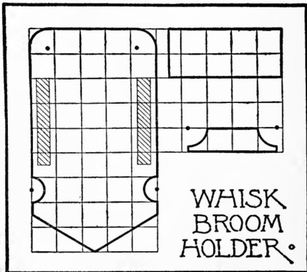
rub the edges smooth with a piece of sandpaper wrapped on something round that will fit the curves. Before nailing up, hold the pieces together and put in the broom to make sure that it will fit. If it is very large or very small, some change may be necessary. Fasten the sides on by small brads driven in from behind, and while the front may also be nailed on, a neater appearance will result if it is fastened with glue and put under a heavy weight
