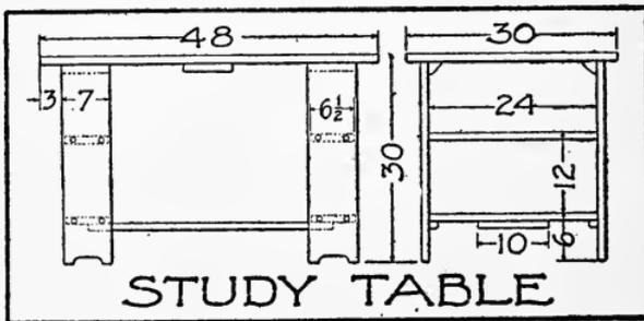
the drawing. If it is desired to have the top look heavier, nail on strips on the under side all the way around and exactly even with the edge. After the table is stained and waxed, cover the top
