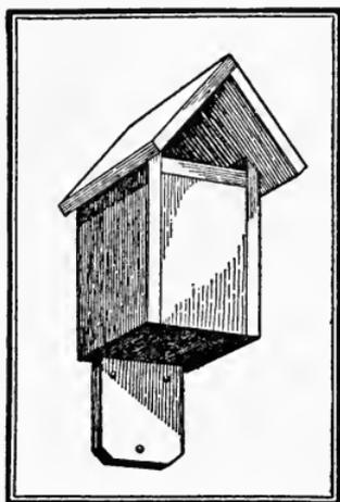
cover the ridge with a strip of zinc or tin to shed the water. It is a good plan in sawing out the entrance to make the outside diameter somewhat larger than the inside, as this will tend to keep the water from trickling inside during a driving rain.
