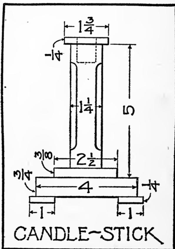
ing, but the small top block should be glued on as we did before. As you sand-paper the edges of the different pieces smooth, test them often with the square to make sure that you are not rubbing one side down more than another. This applies par-
