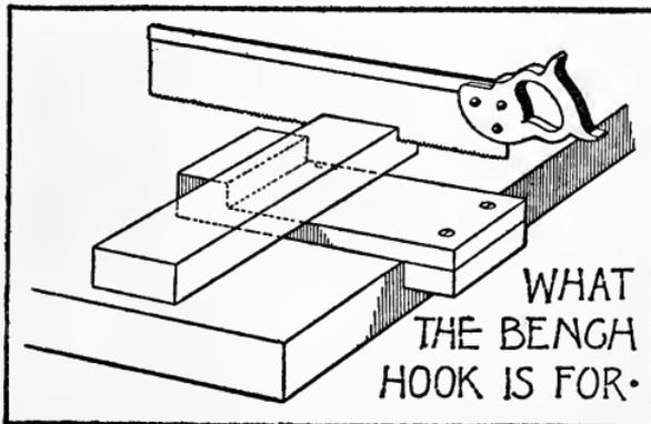
one must have what is called a bench hook. The way it is used is clearly illustrated, but its full advantage cannot be appreciated
