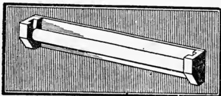
about a half inch thick and twenty inches long, although this measurement may have to be changed a little if the toweling is of some special width. The shape of the end blocks is clearly shown in the drawing. A hole about a half or three-quarters of an inch in diameter is to be bored in the center half-way
