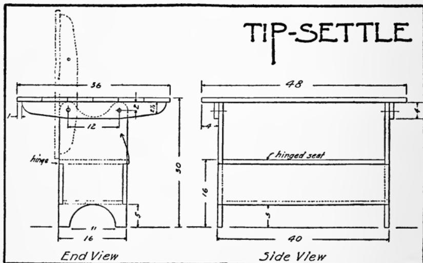
front and back edge of each end board should be notched to a depth of one inch, in order that the front and back boards may be set in flush. After boring two three-fourths-inch holes for the hinge pegs, the ends may be set aside. The front and back boards next demand our attention. These require nothing further than trimming up square and to the proper dimensions. The end boards may
