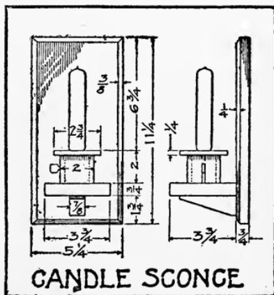
will then be made of one-quarter inch material so as to inclose the socket. A quarter-inch slot will then be made in the center of one side so that the box may be slipped down over the key of the
