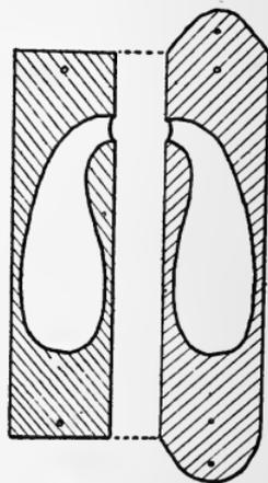
to be fitted in in a manner that will permit of its removal for cleaning. This may be accomplished by securing it in place by driving in about three nails through the sides so as to engage the bottom board. If the proper length nail is chosen and the heads allowed to project about a quarter of an inch they may be readily withdrawn when it is desired to remove the bottom.
