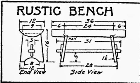
on the underside near each end to receive the supports, the latter should be taken up. Mark out the outline and positions of the mortises for the footrail. These, together with the tops and bottoms, must all be cut at a uniform angle,
