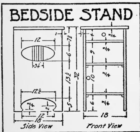
The making and fitting of the drawers in the usual manner will now require attention, after which the three small slats in the elliptical opening of each side are to be placed. As mortises are here im-
