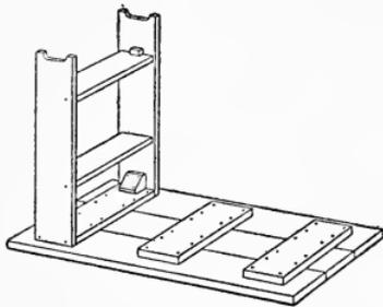
the same length and exactly as long as the cross boards previously nailed underneath the top. In putting together, first nail the two legs and two shelves of each end together. Place the top
