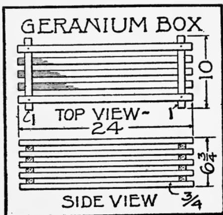
the bottom, and it is a simple matter to add a pair of sides and then a pair of ends until they are all in place. Use the square to make sure that the sides and ends are going up squarely, and always nail in at an angle so that the nails of the next pair of strips will not interfere.
