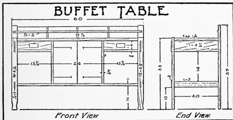
pieces all square with one another. The top board is now to be prepared. If a board of the required width cannot be found it will be necessary to glue up two smaller pieces, but in either case be sure to take particular care in finishing the upper surface and the exposed end wood.
