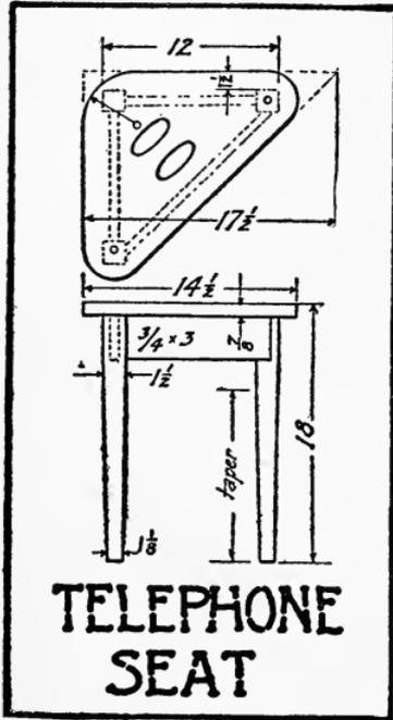
around the periphery to hold the 'phone in place. The supporting arm will be fastened across the bottom at right angles to the grain of the tray. A piece of round tubing or steel about six inches long is then securely fastened into the arm and a suitable hole bored into the stand so that the whole may swing freely.
