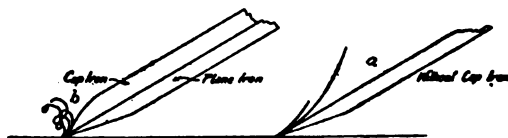
Fig. 115. The action of the cap iron
