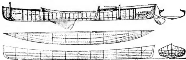
Decked Cruising Canoe, Folding Centreboard and Drop Rudder.
