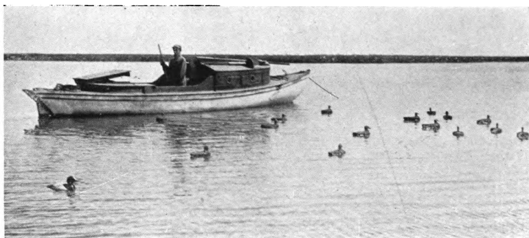
THE HUNTING CABIN LAUNCH Engine is under the lazarette astern.
