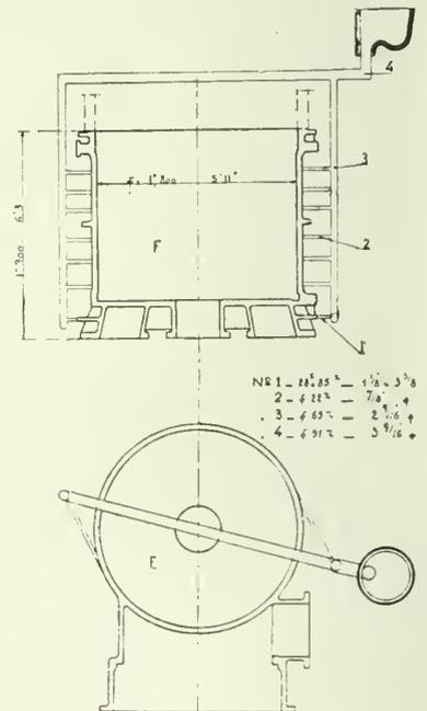
Fig. 6—The arrangement of the runners and risers.
