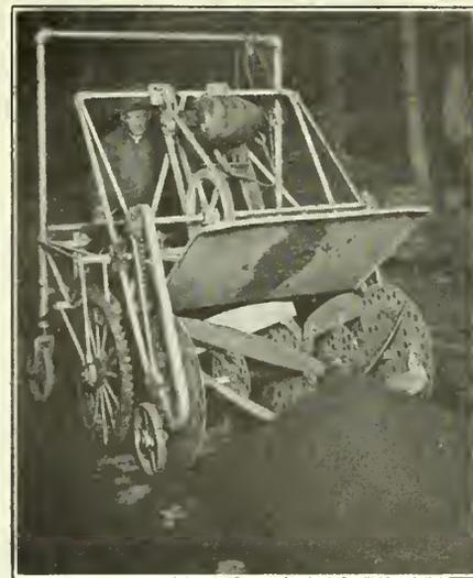
Sand cutting machine in operation.
