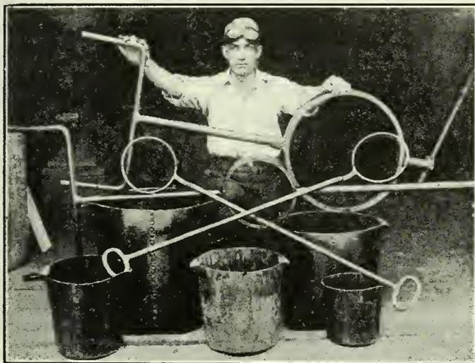
All the ladles in this picture are Oxy-Acetylene Welded. That's the *Damp* method! They are made of steel throughout and because of this will give service possible in no other ladles. Built in capacities to meet all your requirements.
