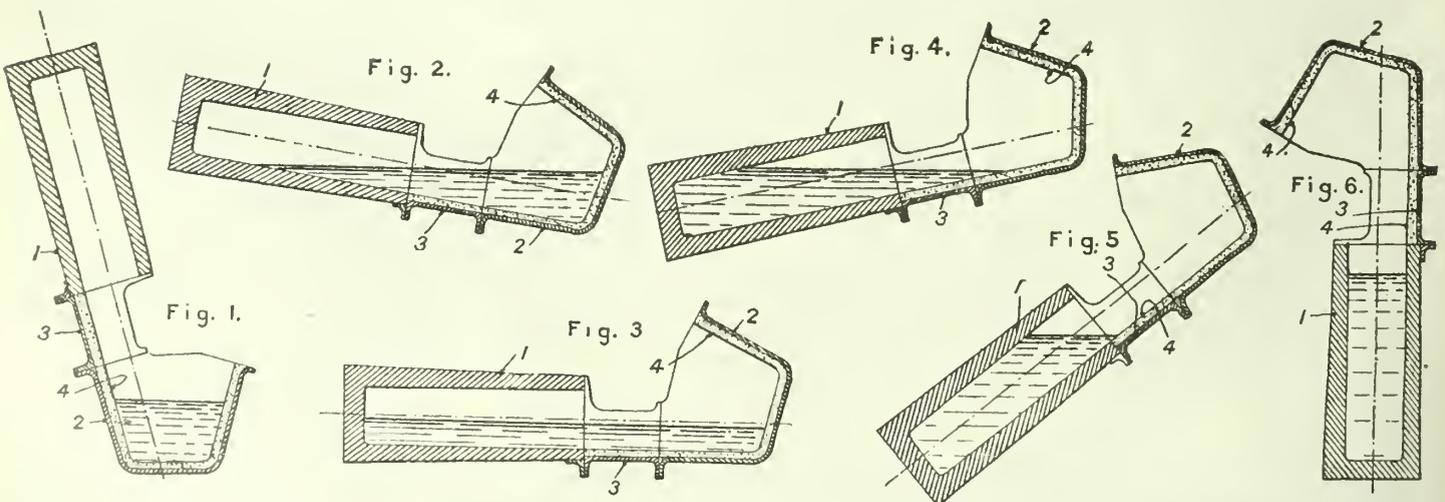
Fig. 1 Shows the three sections of the apparatus together with the refractory lining. Figs. 2-6 show the different position of the metal until it arrives in the ingot mold.
