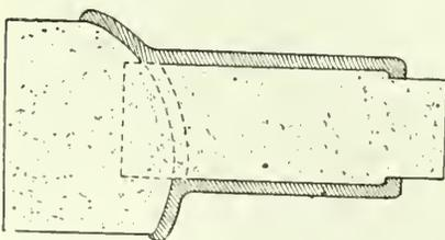
Fig. 2.—Same casting being molded on its side with two cores fitted together to form the inside.
