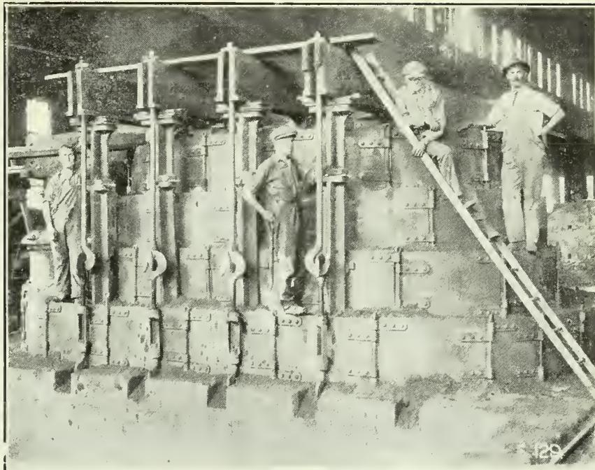
Fig. 8.—Mould for runner section of 11,300 H.P. turbine closed ready for pouring. Attention is drawn to the sectional style of flask.
