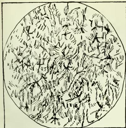
Fig. 11.—Structure of Alloy. 91 per cent. Zn+6 per cent. Cu. + 3 per cent. Al. X 18.
