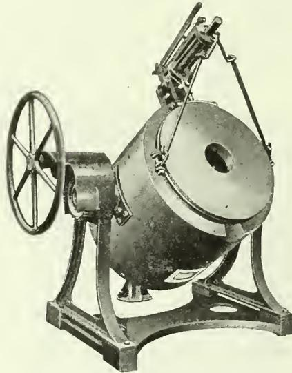
Fig. 3.—Crucible furnace, same as Fig. 2, tilted as in pouring.
