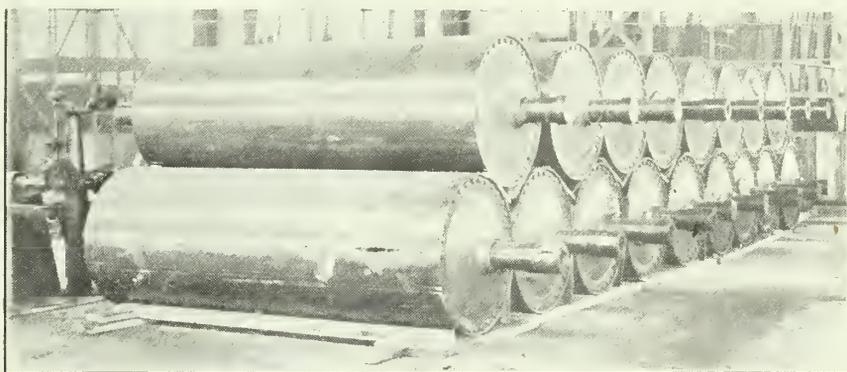
Group of finished semi-steel Dryers. These are loam castings, cast on end in special casting pits, of which there are two, one 8 ft. 6 in. dia., one 12 ft. 0" dia.; both 16 ft. deep.
