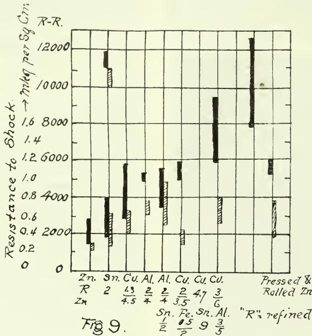
Fig. 9.—Comparison of the tenacity of zinc and zinc-alloys (Chill-cast.) The resistance to rupture (in Kg per 1000 sq. mm of the breaking cross-section) and the impact tenacity (MKg per sq.cm) represent the mean value from numerous experiments with worked bodies.
