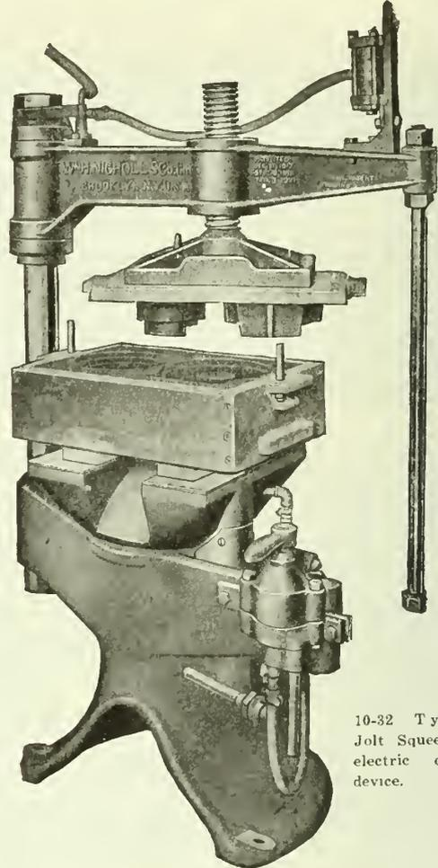
10-32 Type E Jolt Squeeze and electric drawing device.
