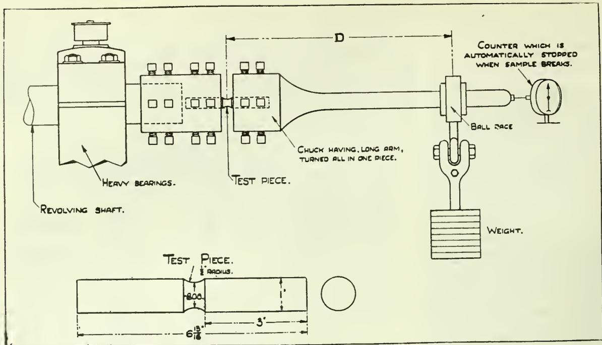
Fig. 6.—Apparatus for rotary fatigue test by the Wheeler method.
