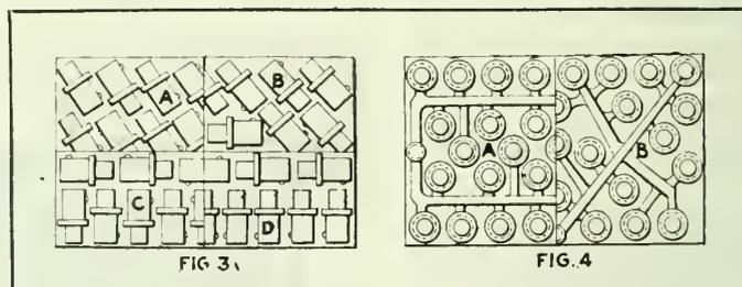
mold. This was 17 in excess of the number of patterns spaced on the two-part flask plates as originally designed, and from which not one casting free from porosity was obtained.
