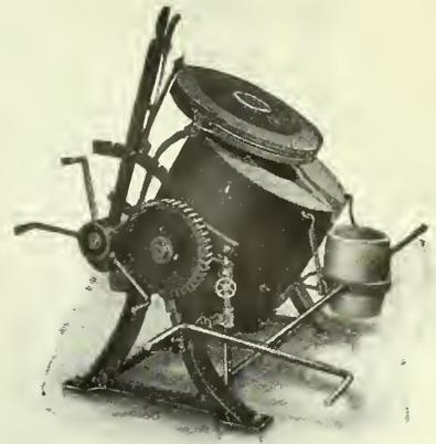
**P**OURING from a full crucible into a mold set on the ground or on a stationary platform has one great disadvantage. There is sloping, spilling, waste—due to the constantly changing and lowering of the crucible lip.
