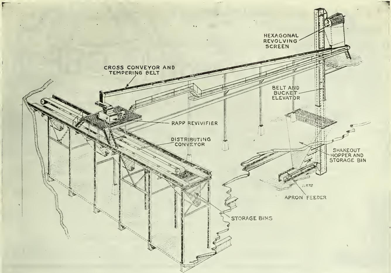
General arrangement of Link-Belt sand handling equipment. Wolff Mfg. Co., Chicago.
