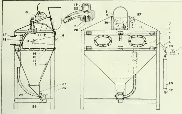
Construction details of sand-blasting cabinet.
