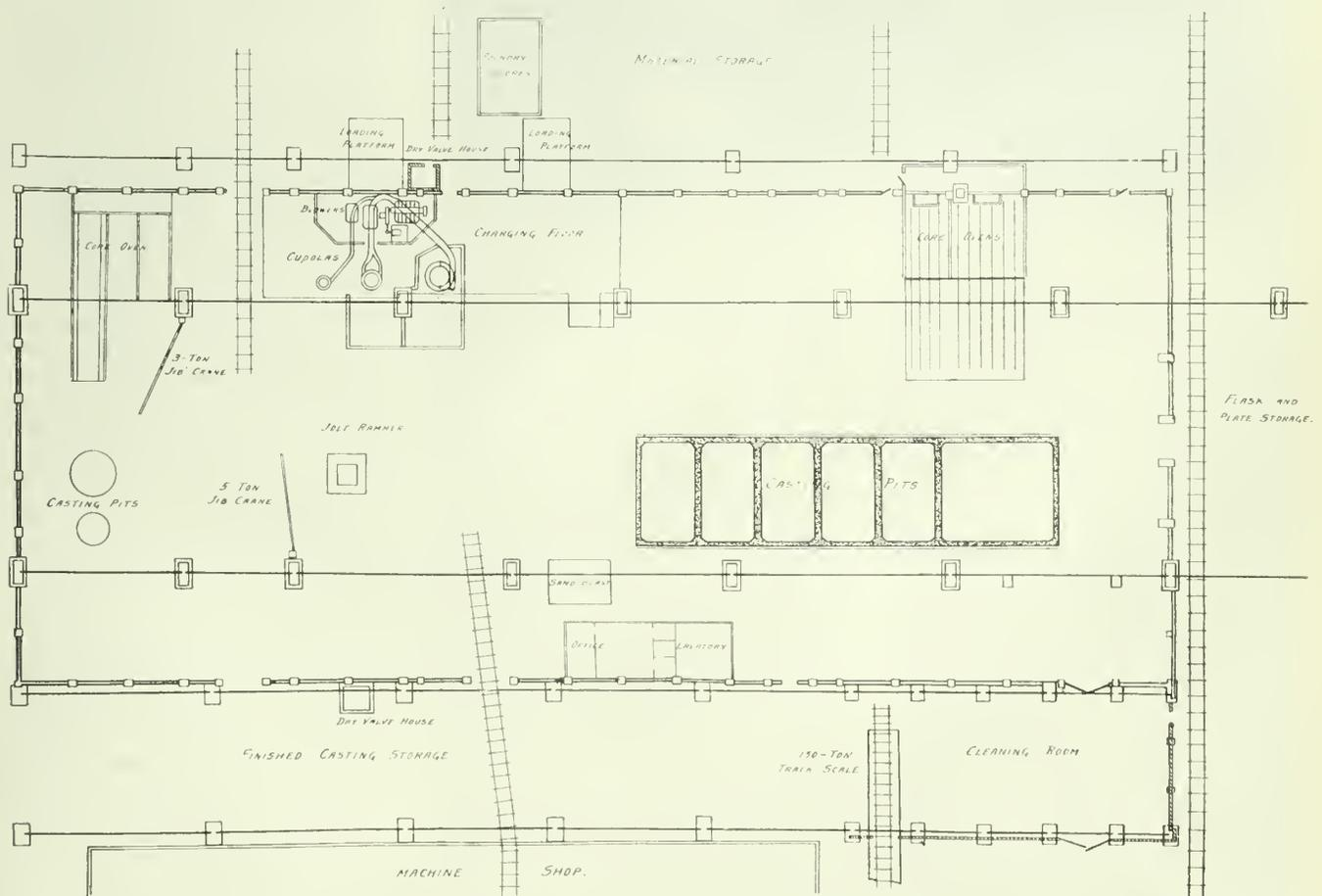
Fig. 1.—Plan view of foundry, Dominion Engineering Co., Lachine, Quebec, showing lay-out of different units of equipment.
