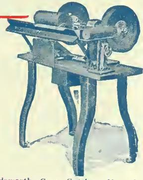
Wadsworth Core Cutting-off and Coning Machine.
