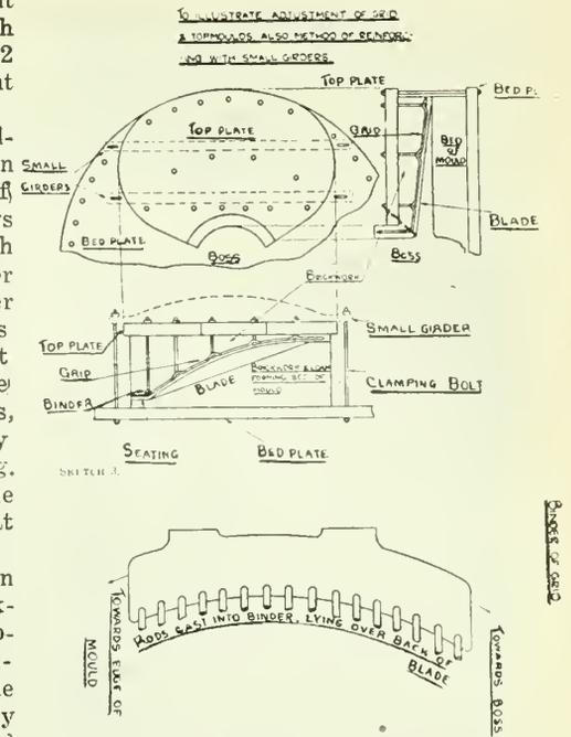
Top view shows grid. Center view shows cope clamped down with cover plate. Bottom shows binder rods
