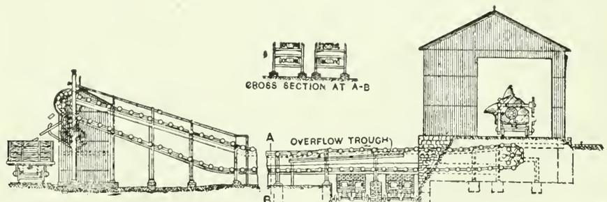
Plan of entire machine required for casting pig iron. The melted metal is under a roof while everything else is out of doors. The worst rain storm can do no harm as it will only assist in cooling the pigs, while the empty molds will be bottom side up, when returned.
