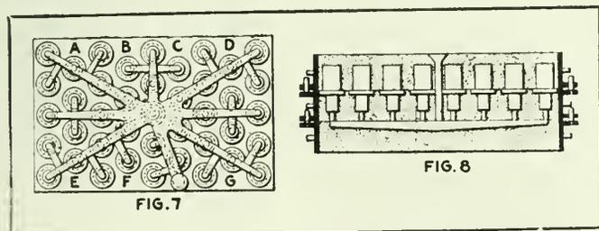
a hundred castings than one with the horn gate. This would appear to be a wild statement, but on analysis it develops that the handling of a single horn gate to place in correct position, or near it, and keep it there, involves molding skill of a high order. Moreover much time is consumed in the oper-
