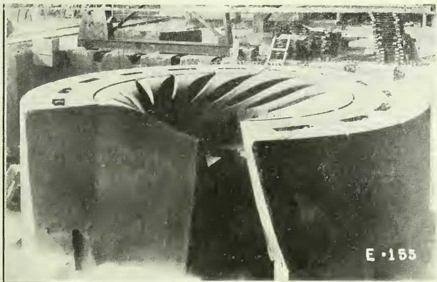
Fig. 7.—View in Foundry showing cores for runner of 41,000 H.P. turbine, being assembled in moulding pit.
