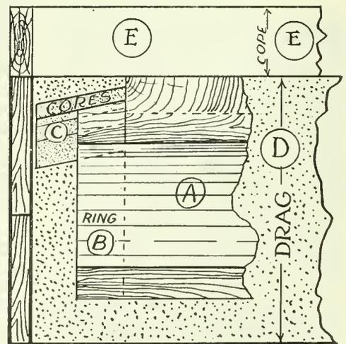
FIG. 2. BROKEN SECTION AT X.X. FIG. 1 SHOWING CORES
