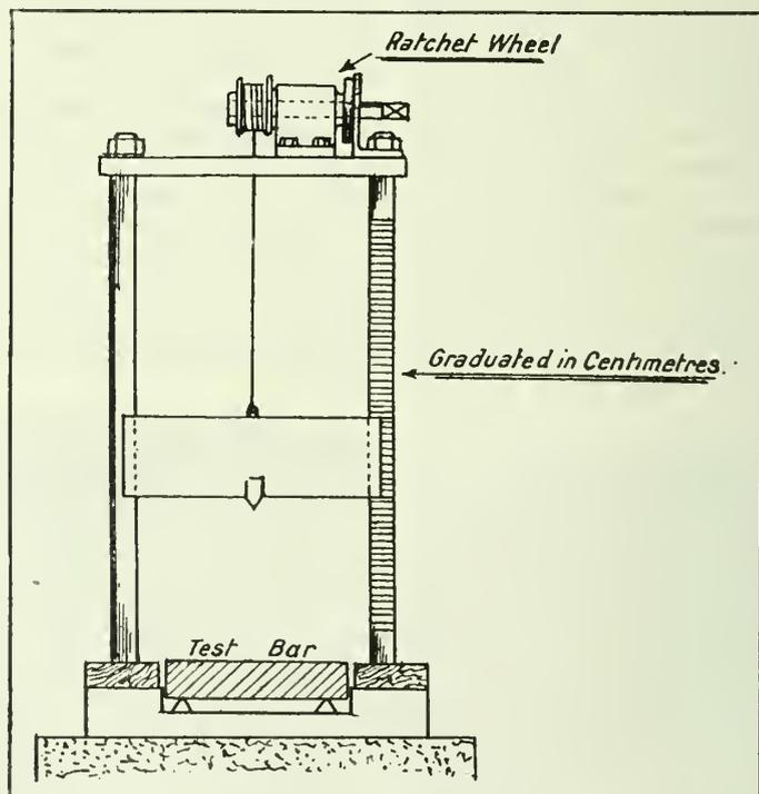
Fig. 7.—Machine used in Europe for testing Gray Iron for shock resisting properties.
