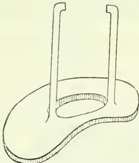
Fig. 1.—Sample casting which could be moulded just as it stands, and leave its own core.
