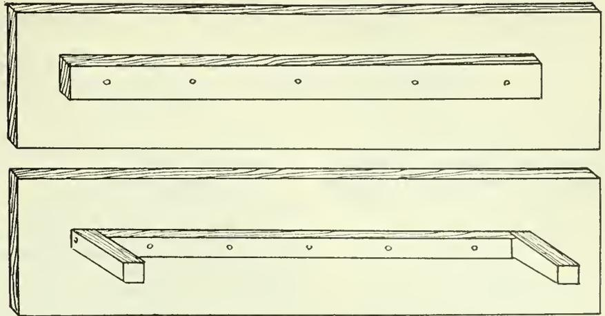
Bottom view shows clamp fastened to match board. Top view shows handle for lifting out the pattern.
