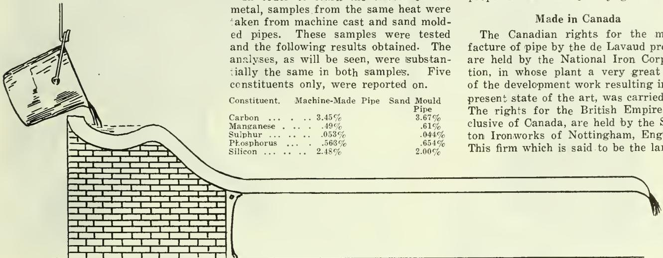
Fig. 2—Trough which extends entire length of the pipe, pouring the furthest end first.
