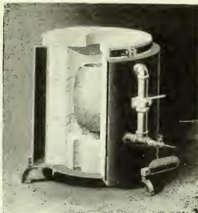
Fig. 1.—Stationary type of crucible furnace.
