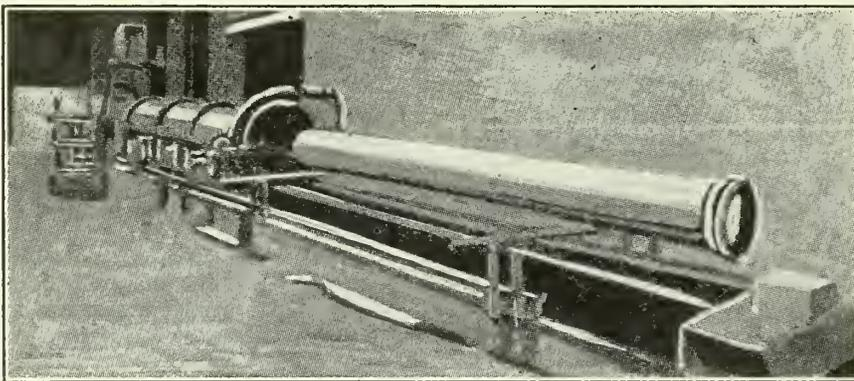
Fig. 1.—14 inch De Lavaud Pipe immediately after leaving machine.
