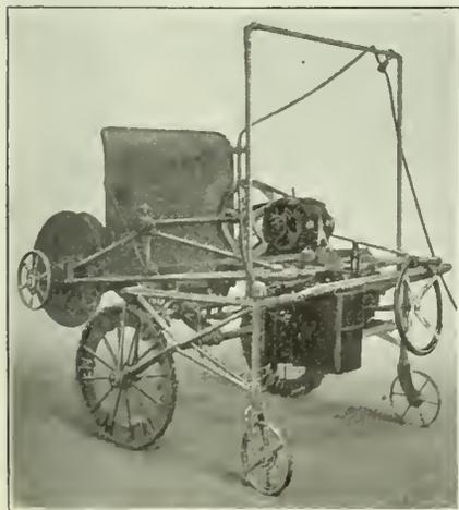
Power sand cutting machine—Type HP.
