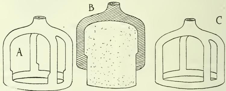
Fig. 3.—A shows casting with clearance for tap. B shows how the core was used to advantage. C shows casting made without core and without clearance for tap.
