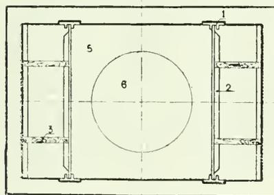
Fig. 7—A convenient casting pit.
