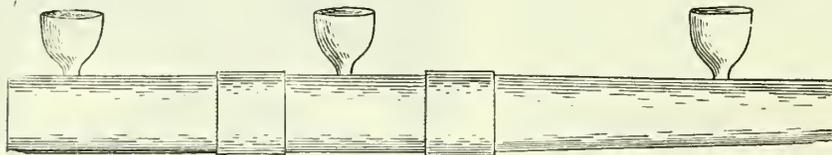
Fig. 1.—Casting which showed shrink under center feeding head.
