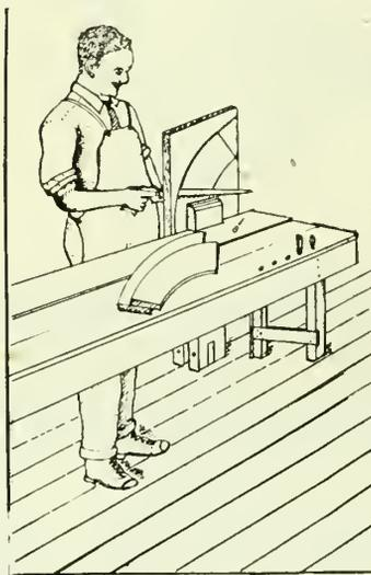
When we cut segments with a key-hole saw.
