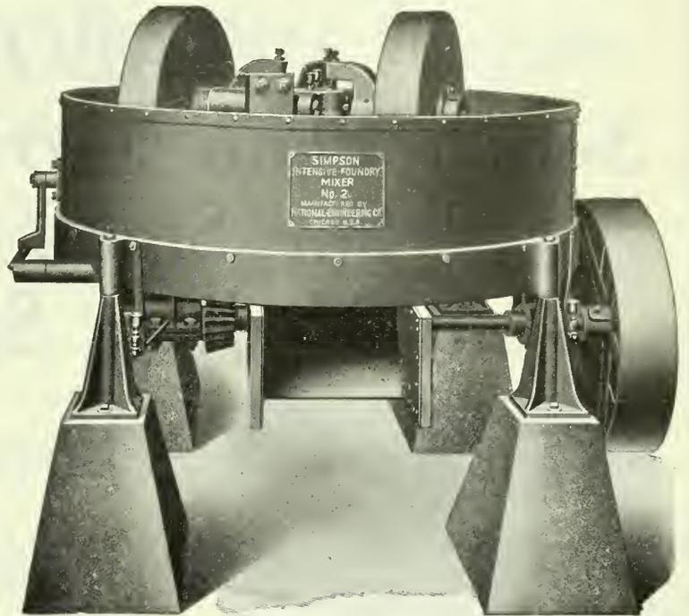
The Simpson Mixer reclaims old and worn-out sand for re-use, thoroughly amalgamates all mixtures and improves the quality of all castings. It operates with small H.P. and is so staunchly constructed that expense for repairs is seldom required. Made in four sizes.
