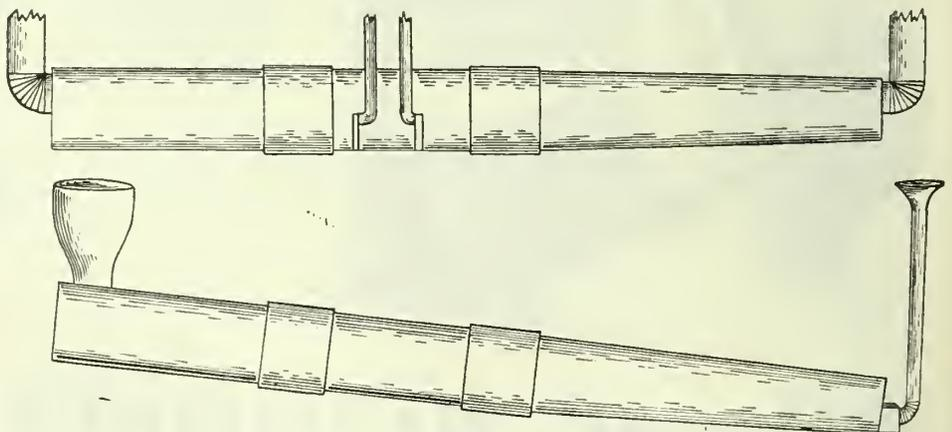
Fig. 2.—Same casting gated on the side and with riser on each end. Fig. 3.—Casting poured on incline. Riser could be at end similar to Fig. 2.
