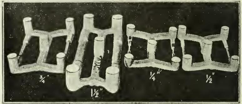
Fig. 1.—Method of casting round test bars.
