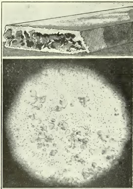
Upper picture is how copper casting appeared. Lower picture shows how it appeared when enlarged.
