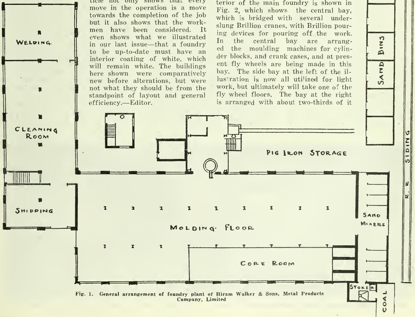
Fig. 1. General arrangement of foundry plant of Hiram Walker & Sons, Metal Products Company, Limited
