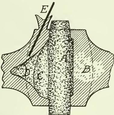
A shows usual way of chambering a hub. B shows castings shrunken internally. C, D, E shows method recommended.
