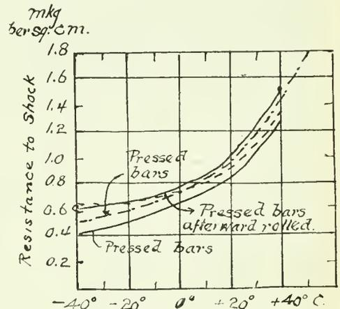
Fig. 5.—Dependence of the impact tenacity of the pressed zinc of various manufacturers upon the temperature
