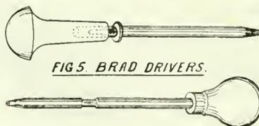
the tool is driven into the wood without bending it. It is not even necessary to use a nail set, for the driver will set the brad deep enough, whether it be hard or soft wood, cardboard, or leather. The brad driver should have a place in every patternmaker's tool kit.
