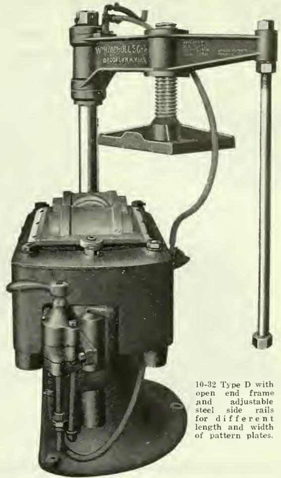
10-32 Type D with open end frame and adjustable steel side rails for different length and width of pattern plates.
