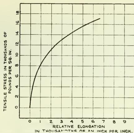
Fig. 2—Stress-strain diagram of alloy containing 92 per cent. aluminum and 8 per cent. copper.
