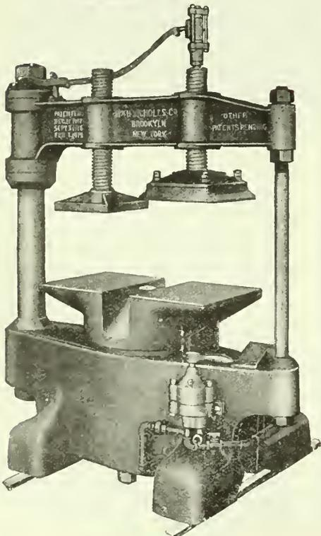
14-42 Combination Duplex Portable Jolt, Squeeze and pattern drawing device. This combination can be made up with three different types of heads or drawing devices.
