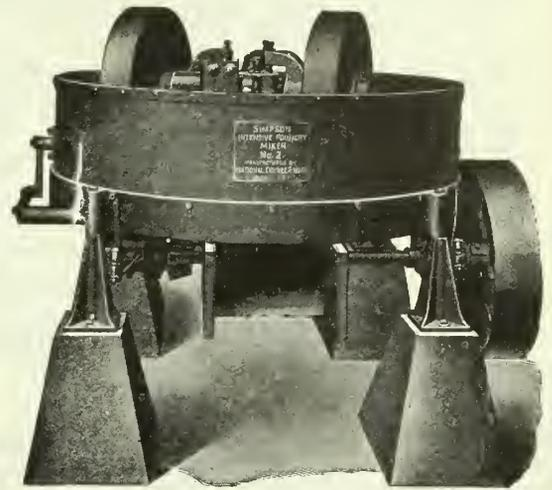
The Semi-Steel Test Foundry Co. also say that their Simpson Mixer gives them quality results for facing and core sand using both oil and pitch binders.
