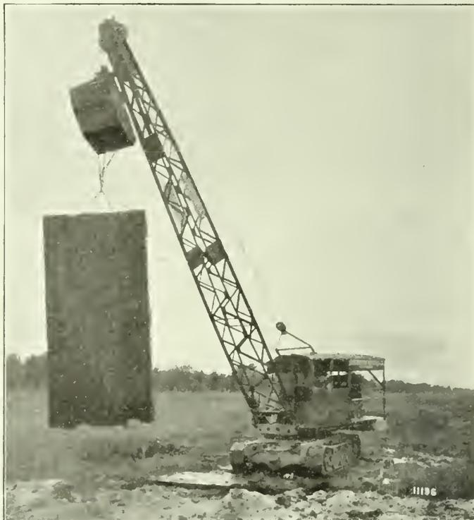
Crawler crane, carrying heavy load over uneven, swampy ground.
