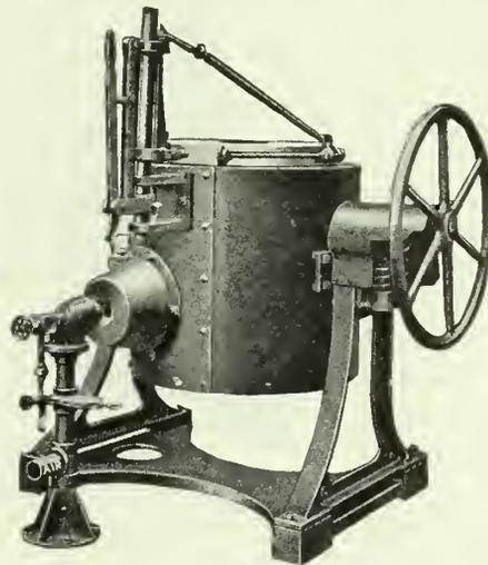
Fig. 2.—Tilting crucible furnace, similar to stationary type.
