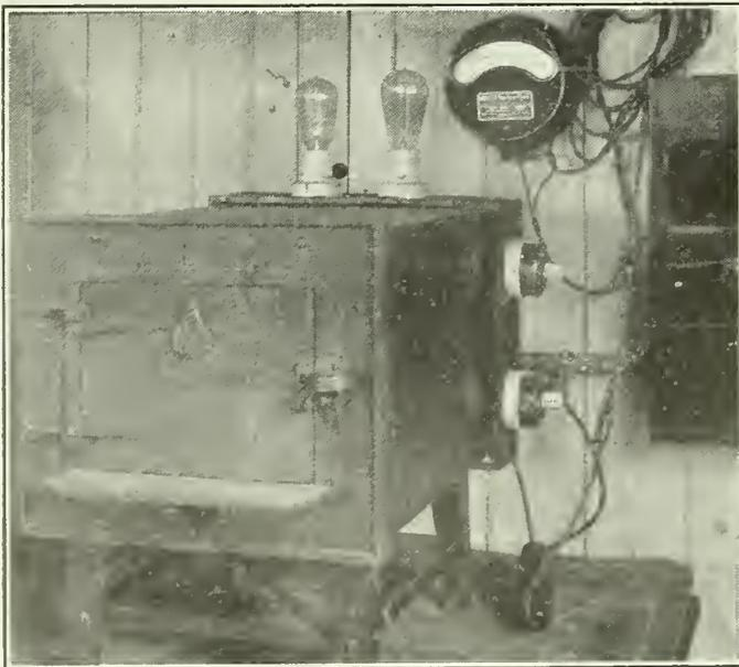
Electric furnace used by manufacturing jeweler in enameling name plates, society pins, etc., and also for hardening dies and tools.
