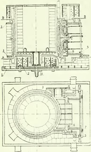
Fig. 5—Details of marine engine cylinder mold.
