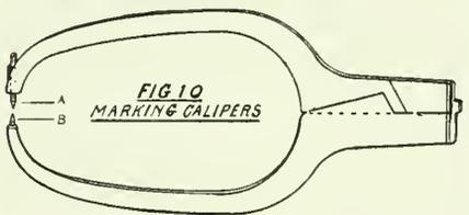
FIG 10 MARKING CALIPERS
