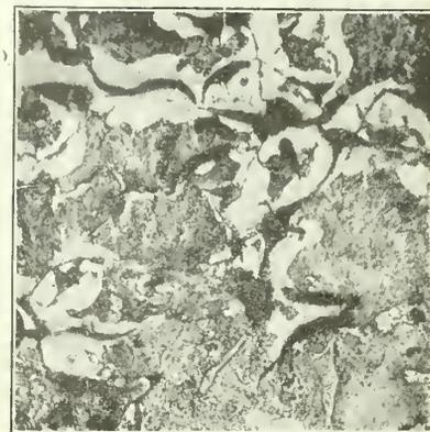
Micrograph No. 4—Thick end of wedge No. 2—10 per cent. semi-steel. (Notice smaller graphite flakes compared with micrograph No. 1.)
