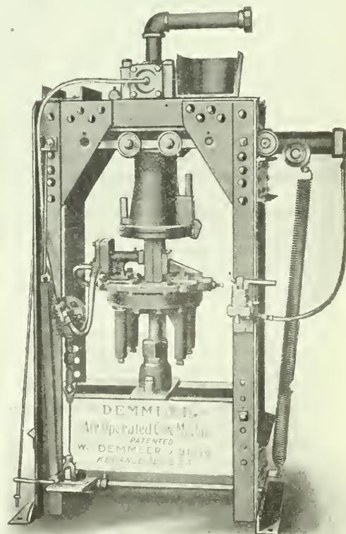
Demmler air operated core-making machine without the automatic sand elevator.
