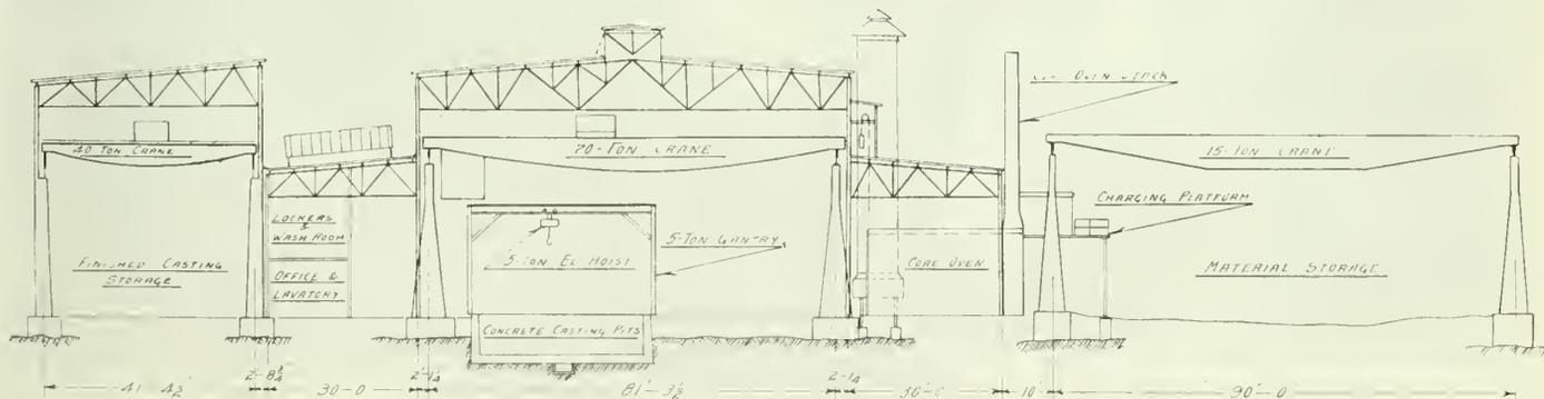
Fig. 2 Shows Cross section view of foundry department, Dominion Engineering Company, Montreal.
