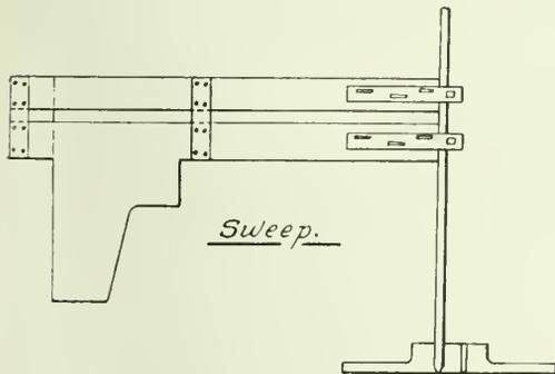
Fig. 2—Ordinary sweep and spindle which can be changed to suit any condition.
