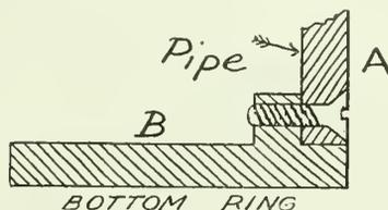
Showing method of securing shell to avoid undue weight on edge of wall.
