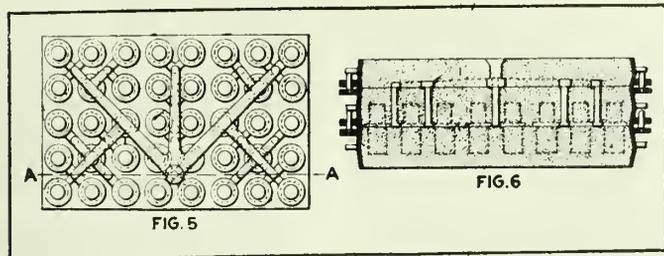
castings with only 16 upright feeders. This arrangement is of rather dubious advantage, but it can be adapted to some classes of work. Fig. 7 serves to illustrate how bad a runner layout can be to offset the virtues claimed here for overhead or bottom pouring.
