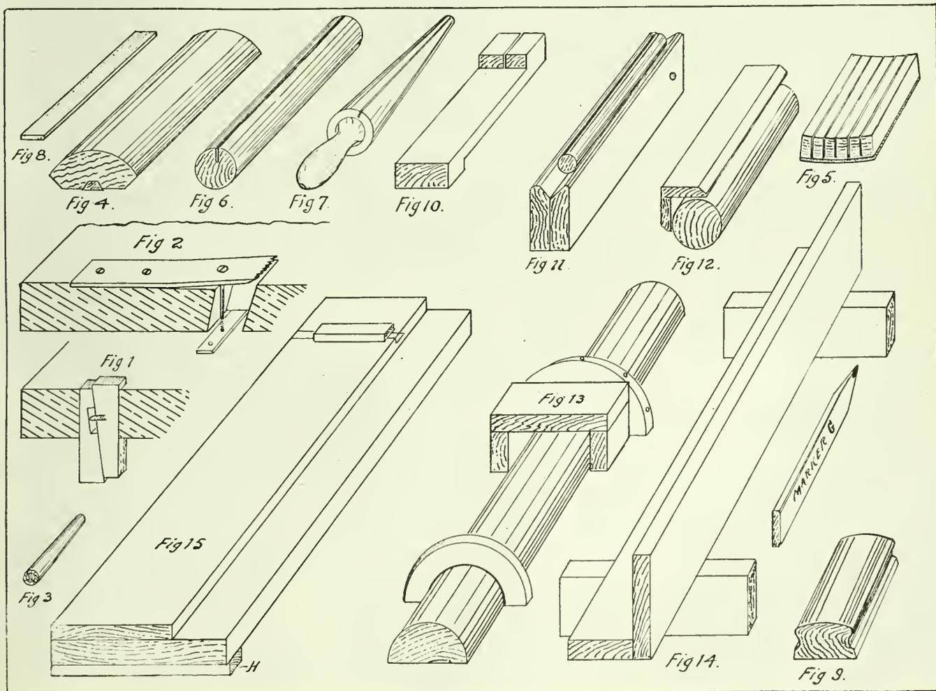
vides with the assistance of a screw driver, means of adjusting the stop, which is shown in Fig. 2. There are a larger number of mechanical bench stops on the market, some of them are really effective stops, and much to be preferred to any of the home made varieties. One operating from the side of the bench is most convenient.
