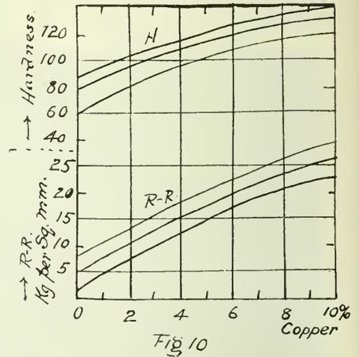
Fig. 10.—Influence of the amount of Cu in the Zn-alloys upon the tenacity and the hardness.
