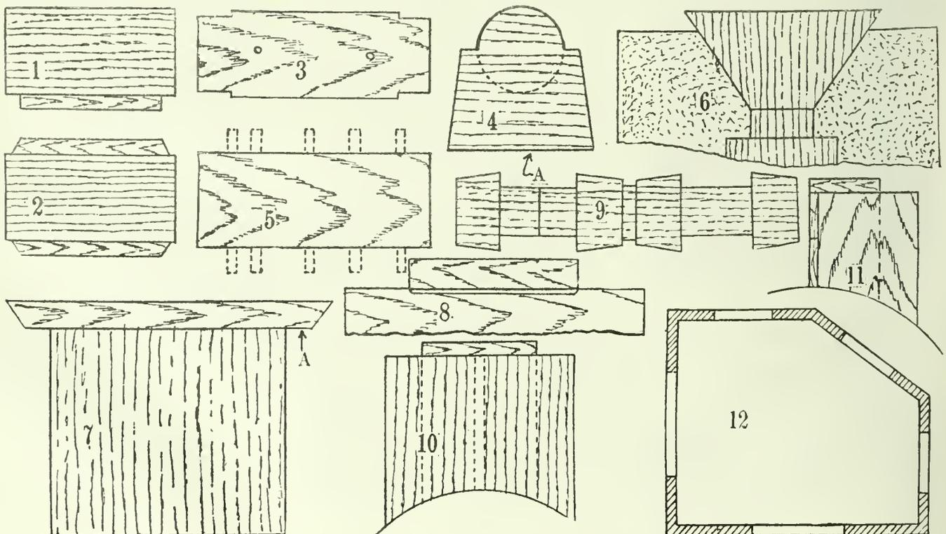
Twelve views of patterns, showing best way of molding in order to have cores placed to best advantage.
