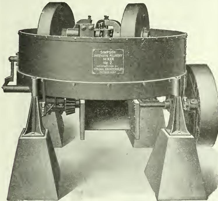
IN AN ORDINARY FOUNDRY of forty to fifty molders, the attention of one man is all that is ordinarily required to mix all of the core sand and facing sand for the entire shop, which is a very great saving of labor when compared with the very inefficient idea where every molder mixes his own facing sand by hand. Generally, the saving effected by the concentration of the sand mixing operations will amount to the price of the Mixer in a few months.
