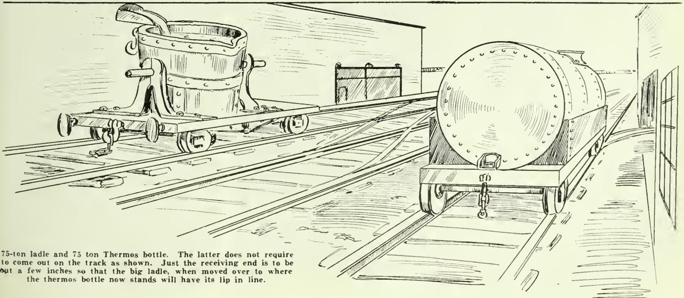
75-ton ladle and 75 ton Thermos bottle. The latter does not require to come out on the track as shown. Just the receiving end is to be put a few inches so that the big ladle, when moved over to where the thermos bottle now stands will have its tip in line.
