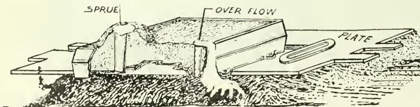
Burning patch on aluminum casting by flowing melted metal in one gate and out of another.
