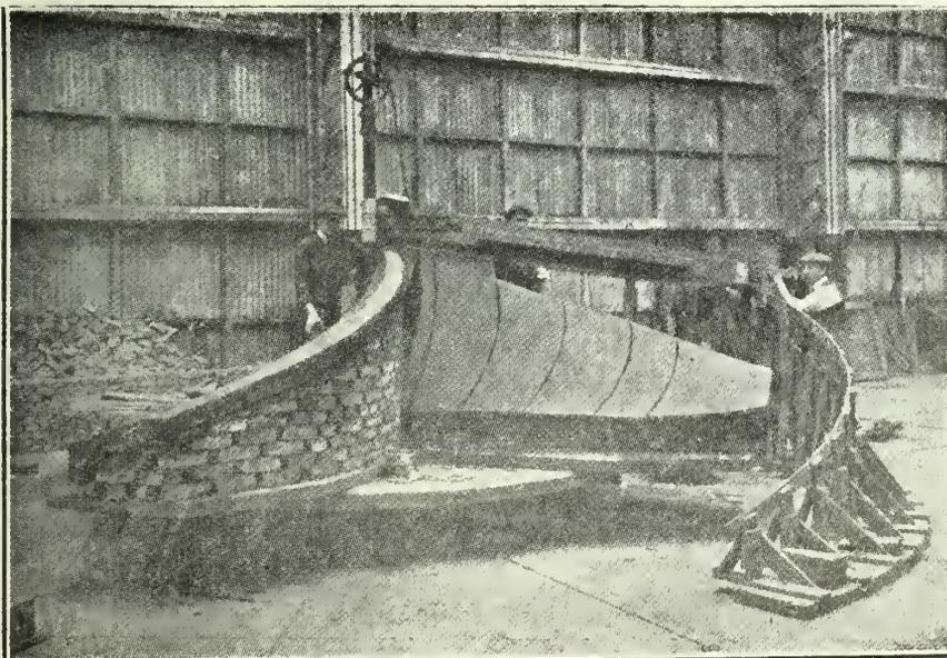
Fig. 1. Sweeping a blade. Note the guide or pitch piece to the right
