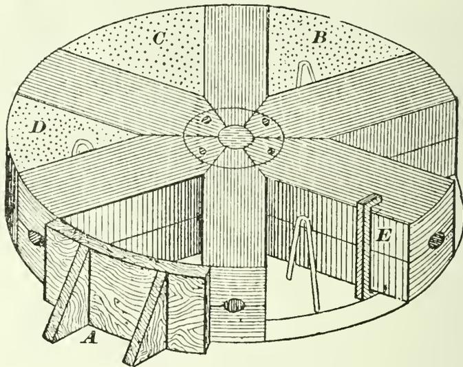
Fig. 1—Simple band wheel made up with cores and segment.
