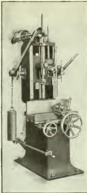
front of the machine. The drive is entirely self-contained; a countershaft is fitted in the base of the machine, and from this the drive is taken by belt to the chain mortising spindle.
