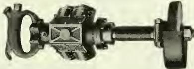
The size G, illustrated, is a "one man grinder," has 3300 r.p.m. Weight, 19 lbs. Adapted for grinding castings, etc.
