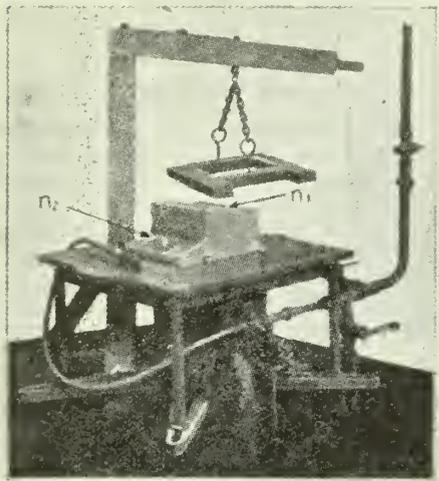
Fig. 1.—The molds are made on a jar ramming machine.
