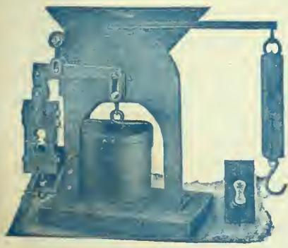
Wadsworth Core Testing Machine
