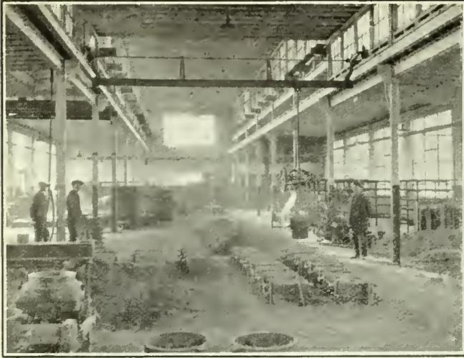
Fig. 2. Main bay of foundry showing Brillion crane in center
