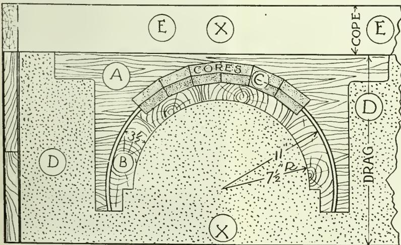
FIG. 1 SHOWING MOLD WITH SIDE OF FLASK REMOVED
