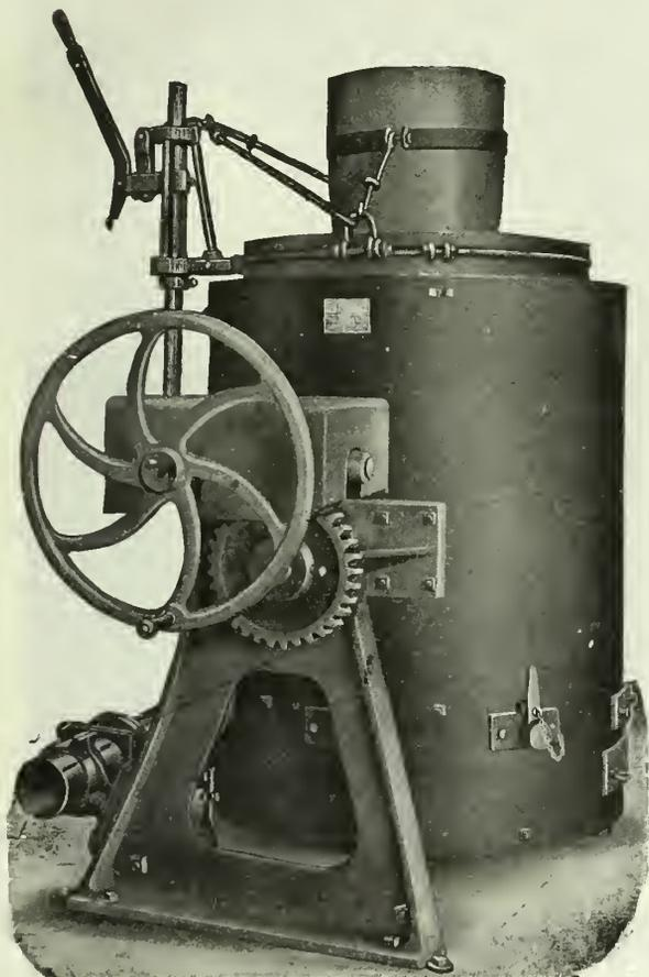
Tilting Crucible Coke Furnace
