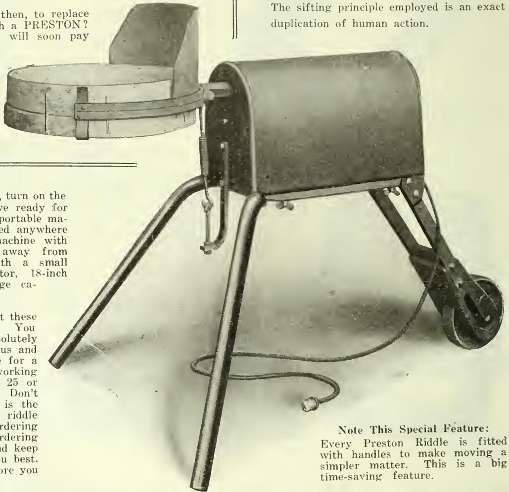
**S**CREW the socket in, turn on the switch and you have ready for action a light-weight portable machine that can be used anywhere in the foundry; a machine with all parts enclosed, away from dust; a machine with a small power-consuming motor, 18-inch hand riddle and large capacity.
