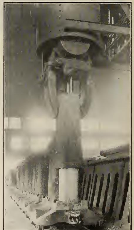
STRIPPING THE MOULD FROM THE HOT INGOT.
