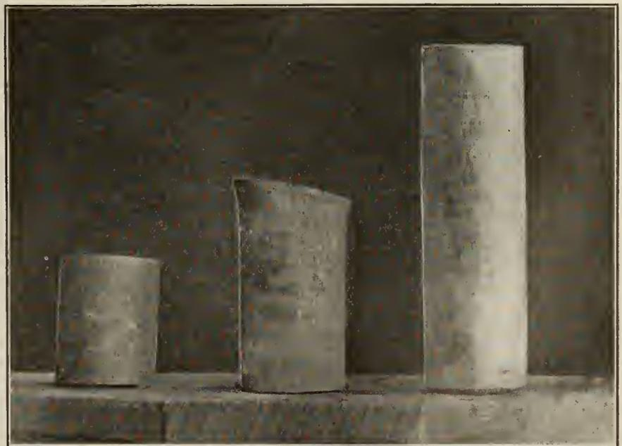
FIG. F—SHOWING STEEL BILLET, SHELL AFTER FIRST OR "PIERCING" OPERATION AND FINISHED FORGING.
