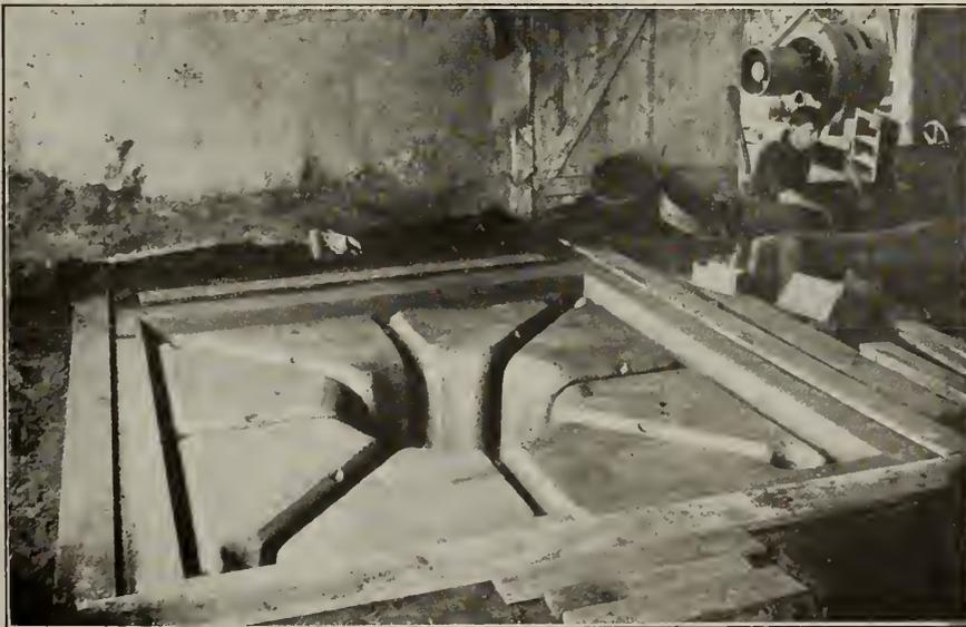
FIG. 2. COMPLETED GREEN SAND MOLD FOR ACCUMULATOR BASE.
