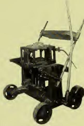
**T**HIS machine is a combination of a powerful squeezer machine with the Adjustable Drop-Plate Flask-Stripper, and thus gives the user practically the advantages of three machines in one—drop-plate, stripping plate, and squeezer.
