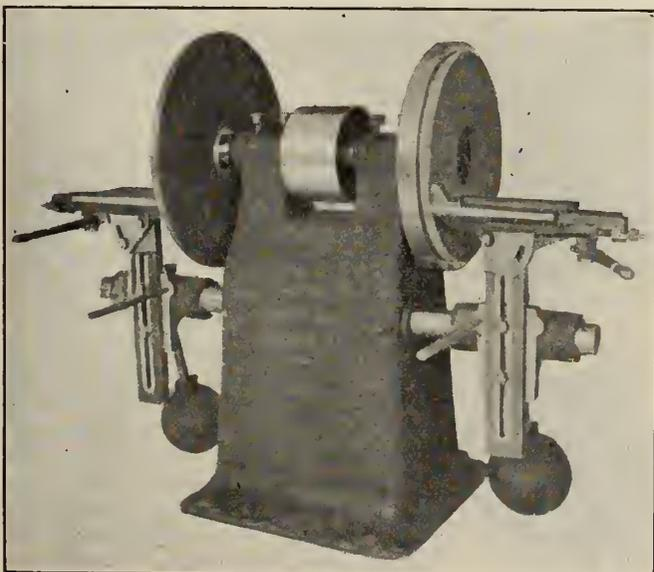
FIG. 1. NO. 17 GRINDER WITH 24-INCH DIAMETER WHEEL.
