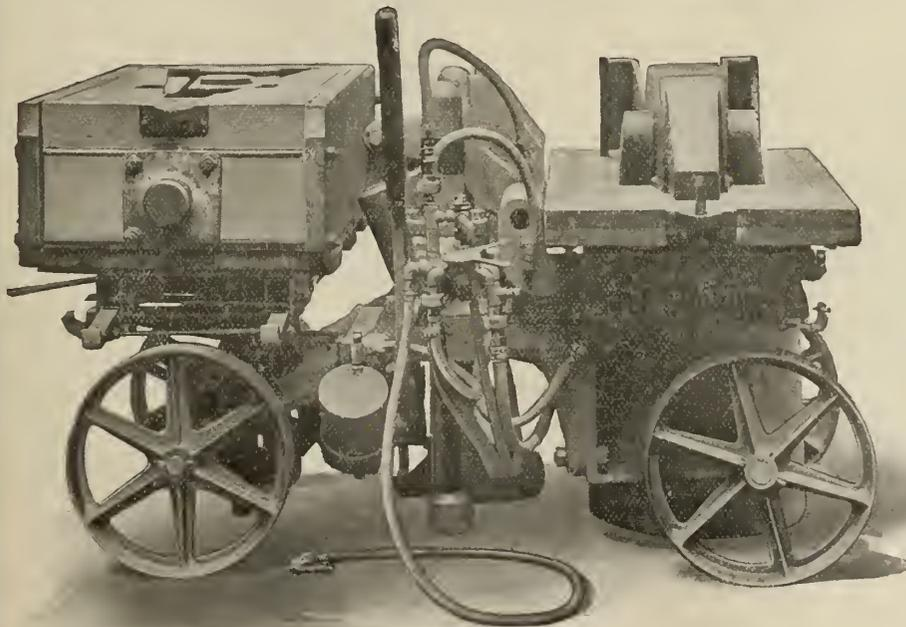
A distinctive Tabor achievement, being a combination of two exclusive Tabor features: the Shockless Jarring Machine and the Roll-Over Straight Draw Machine. Eliminates all ramming time and is suited to a wide variety of work. Send for Bulletin M-S-II.
