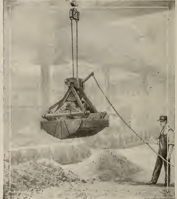
It works from any crane and can be attached or detached in a minute. That is one of the advantages of the
