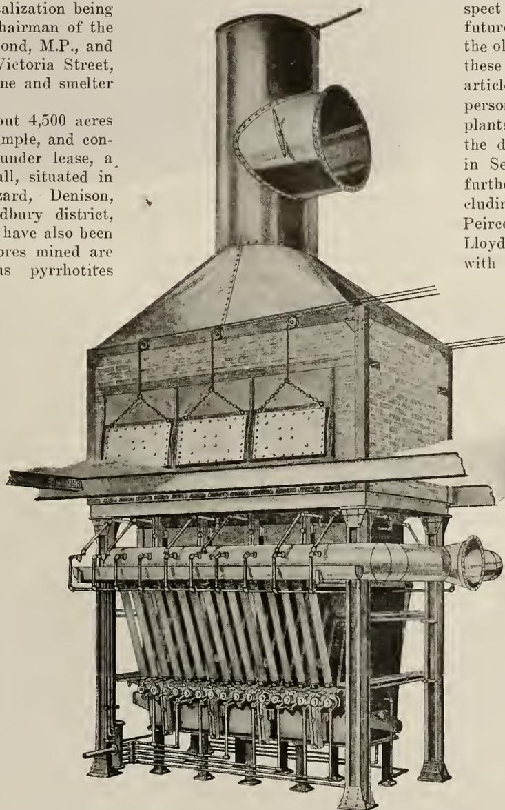
RECTANGULAR WATER-JACKETED COPPER BLAST FURNACE. ORIGINAL TYPE USED BY THE MOND NICKEL CO., 1909, VICTORIA MINES SMELTER (A.C. CO.).
