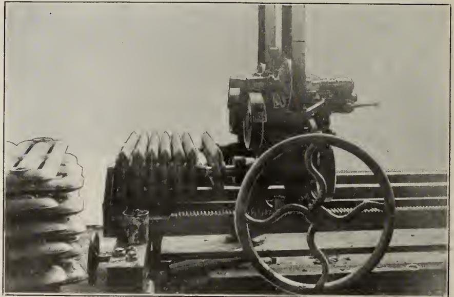
FIG. 7. RADIATOR ASSEMBLING MACHINE.
