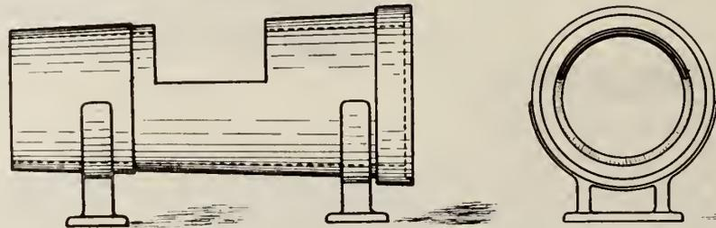
FIG. 20. JIG FOR TESTING TAPER AND OUTSIDE DIAMETER OF BACK ENDS.
