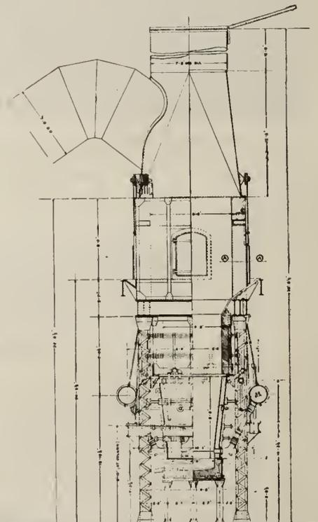
VERTICAL TRANSVERSE SECTION OF COPPER BLAST FURNACE (A.C. CO.), 1912. MOND NICKEL CO.
