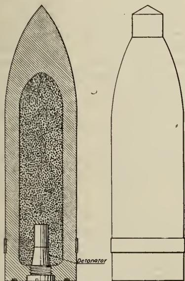
FIG. 1. SIMPLEST FORM OF EXPLOSIVE PROJECTILES.
