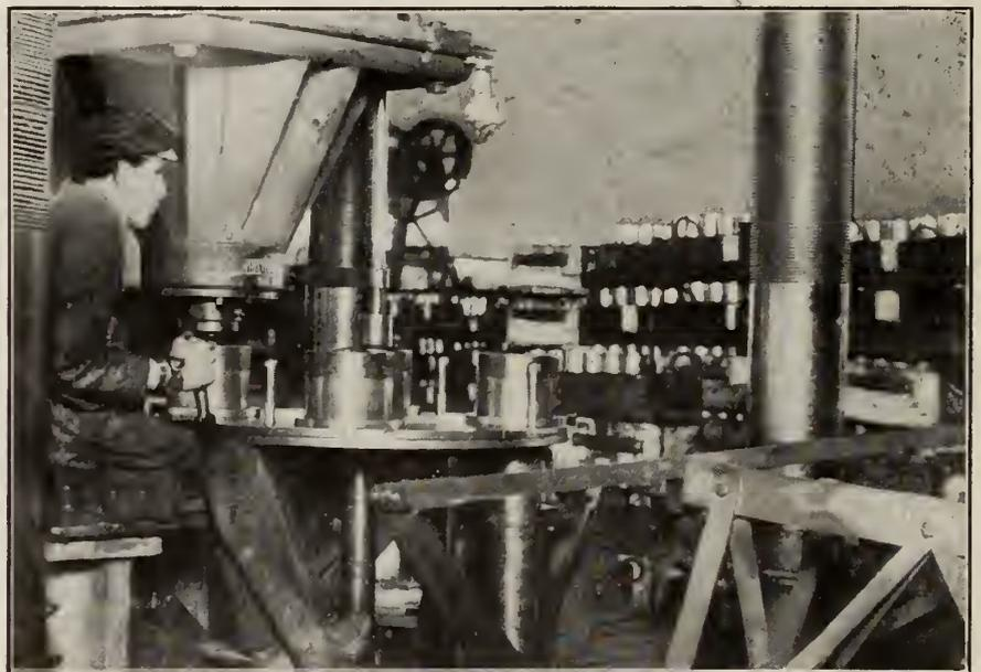
FIG. 8. INDENTING 18-PDR. SHRAPNEL SHELL CARTRIDGE CASES ON A 500-TON HYDRAULIC PRESS.
