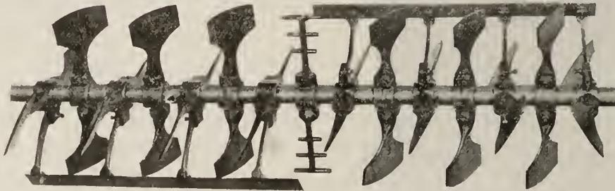
These are the paddles used in a Standard, which **mix** the sand 100 times a minute and not merely turn it over as you would with a shovel. That is why foundries tell us they save from 5% to 50% of Binder.
