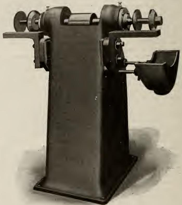
FIG. 2. GRINDING MACHINE WITH BALL BEARINGS.
