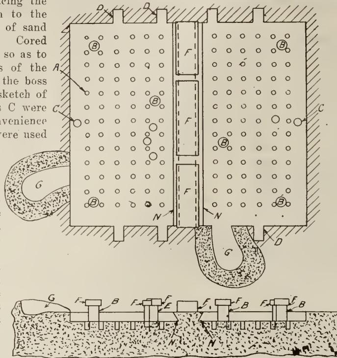
FIG. 5. GREEN SAND MOLD FOR COPE PLATES.
