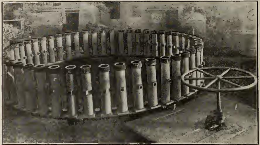
FIG. 4. BATTERY OF INGOT MOLDS READY TO BE Poured.
