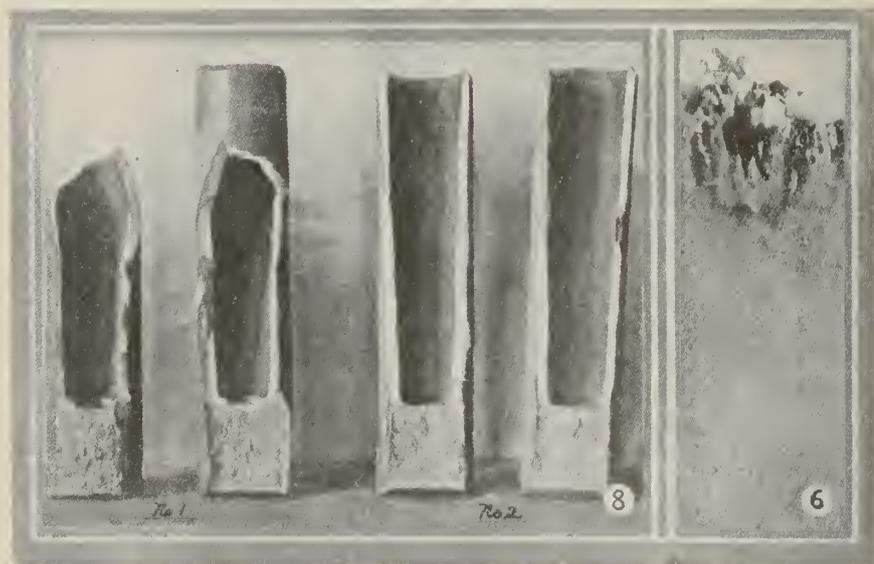
Fig. 6. Etching on axis line to determine amount of segregation. Fig. 7. Shell to gings from blanks (1) and (2) of Fig. 7, split open for inspection.
