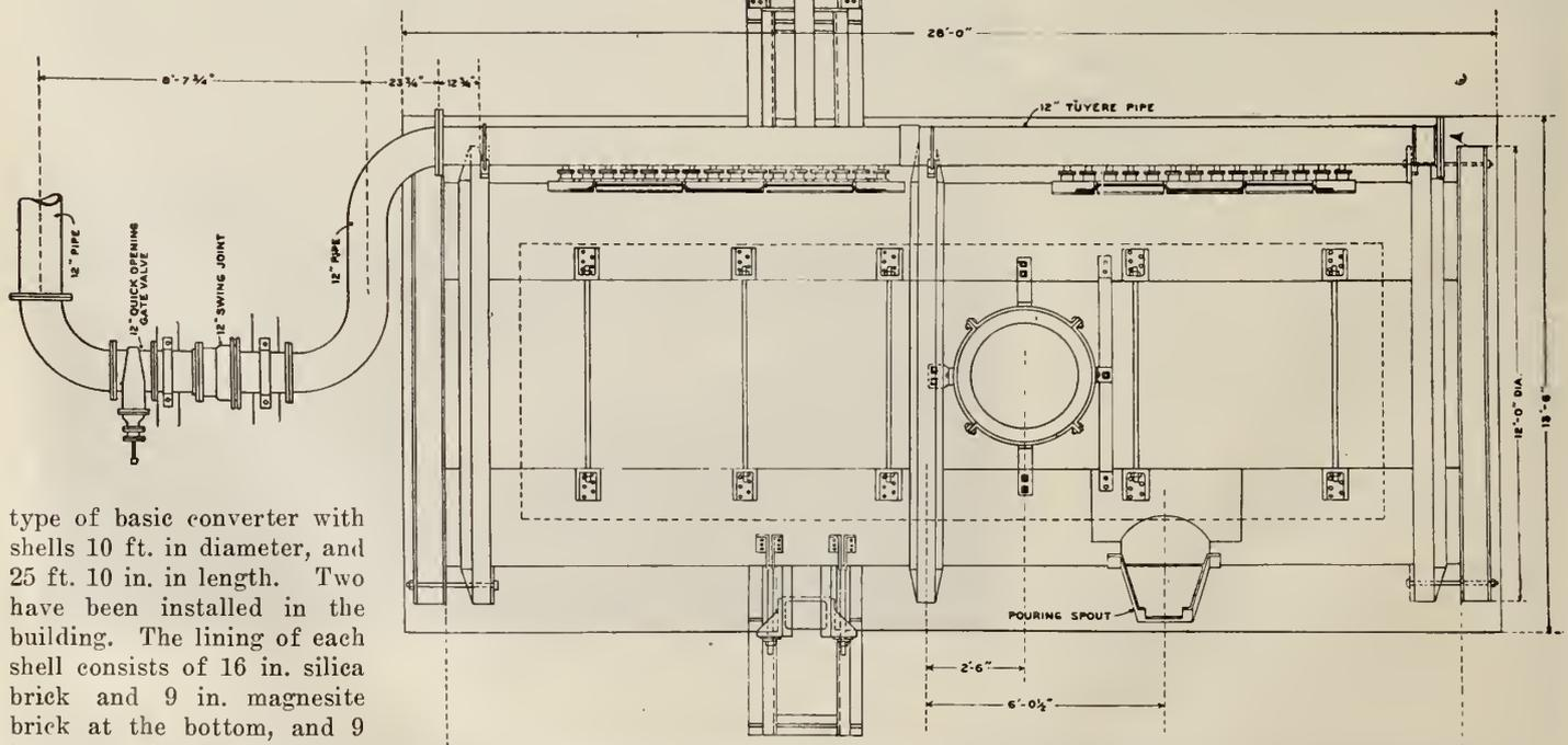
type of basic converter with shells 10 ft. in diameter, and 25 ft. 10 in. in length. Two have been installed in the building. The lining of each shell consists of 16 in. silica brick and 9 in. magnesite brick at the bottom, and 9 in. magnesite brick at the top. At the tuyeres, special
