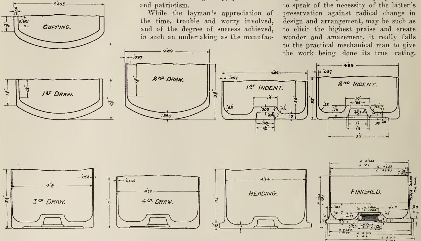
FIG. 23. SERIES OF OPERATIONS THROUGH WHICH THE 4.5 HOWITZER CARTRIDGE CASE PASSES IN THE PROCESS OF MANUFACTURE.
