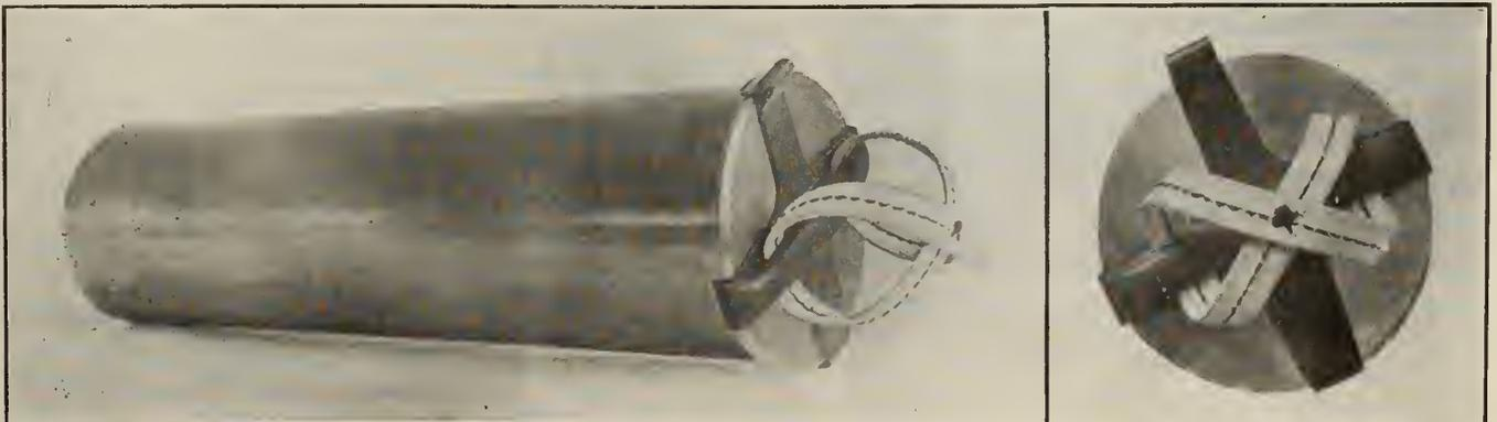
CARTRIDGE CASE WITH DRAWING CLIP ATTACHED.
