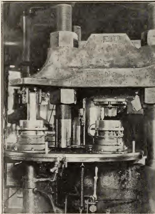
FIG. 15. HEADING 18-PDR. SHRAPNEL SHELL CARTRIDGE CASES ON AN 800-TON HYDRAULIC PRESS.
