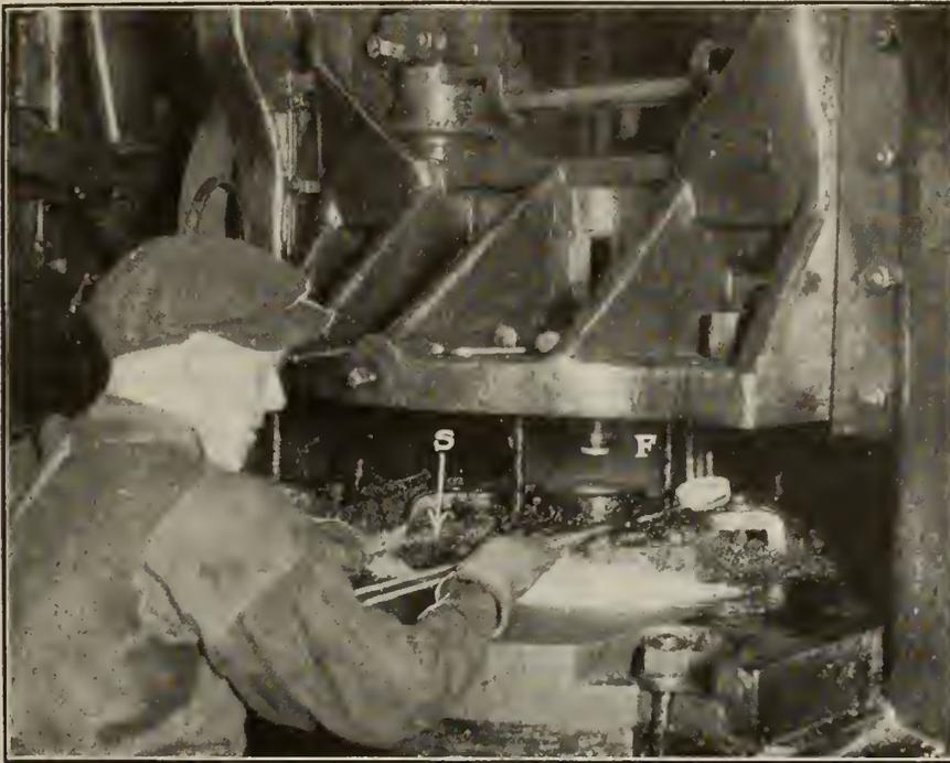
FORGING SOCKETS FROM BRASS SLUGS.
