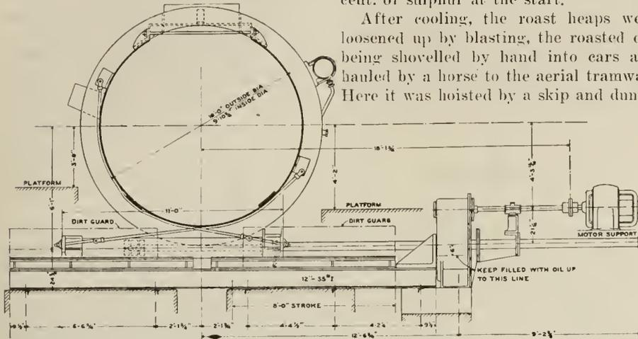
BASIC COPPER CONVERTER, PEIRCE-SMITH TYPE, MOND NICKEL CO. TRANSVERSE SECTION SHOWING ATTACHMENT OF TILTING MECHANISM (A.C. CO.).
