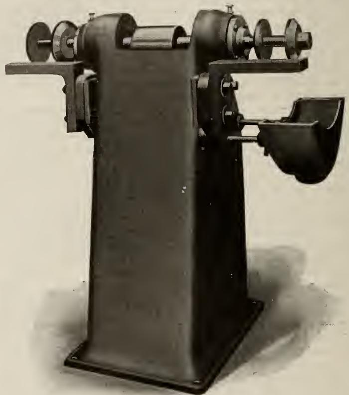
FIG. 2. GRINDING MACHINE WITH BALL BEARINGS.
