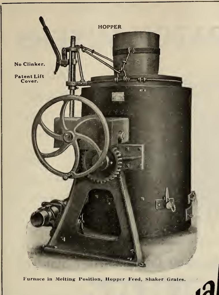
Furnace in Melting Position, Hopper Feed, Shaker Grates.
