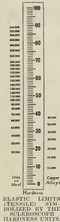
under the scleroscope and the diamond pointed steel hammer allowed to drop on the polished part of shell. The hammer rebounds and the figure at which it stops is noted by the operator. This is repeated several times, the shell being moved round each time. The hardness required of shrapnel shells must be around 45, a slight variation above or below being allowable.
