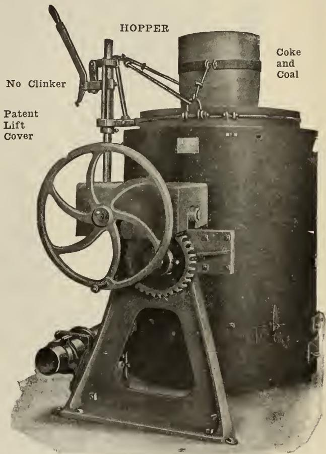
Furnace in Belting Position, Hopper Feed, Shaker Grates.
