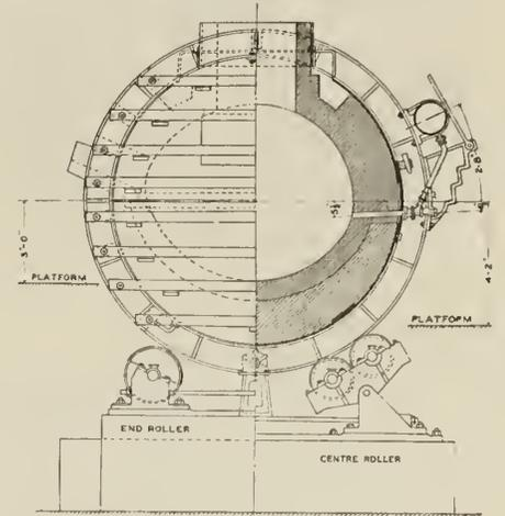
BASIC COPPER CONVERTER, PEIRCE-SMITH TYPE, MOND NICKEL CO. TRANSVERSE SECTION THROUGH WIND BOX AND TYRE ON RING NEAREST THE TILTING MECHANISM (A.C. CO.).
