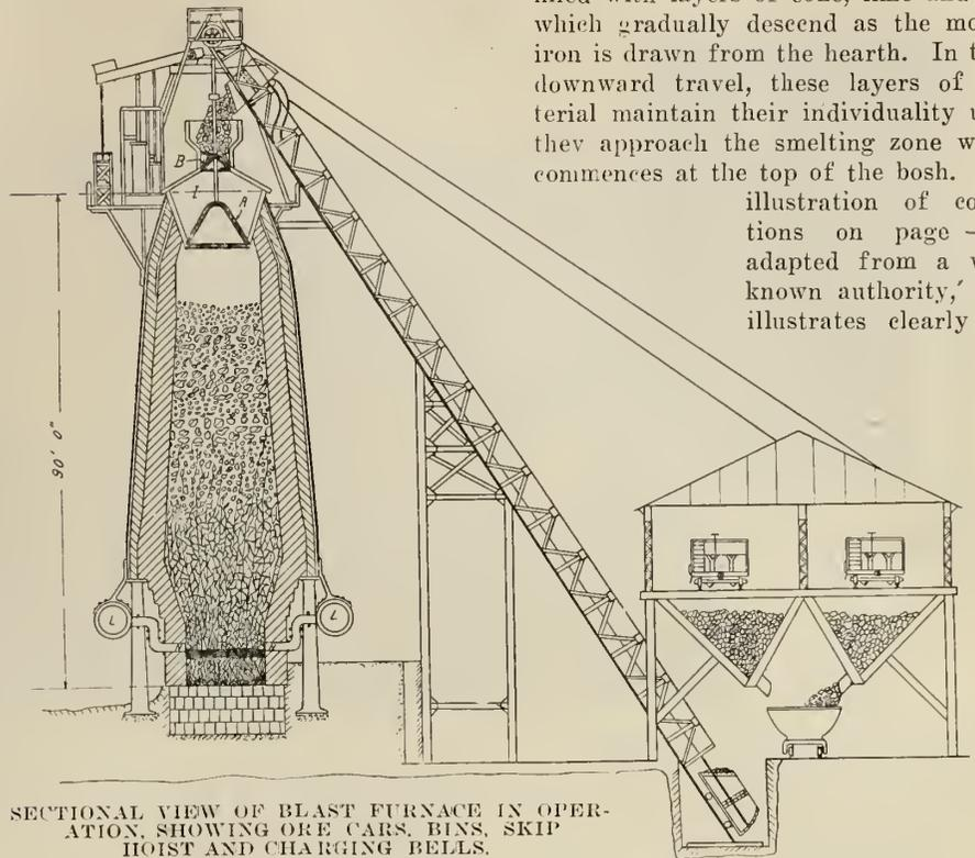
SECTIONAL VIEW OF BLAST FURNACE IN OPERATION, SHOWING ORE CARS, BINS, SKIP HOIST AND CHARGING BELLS.
