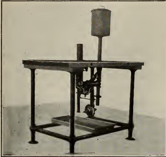
SHRAPNEL SHELL SPRAYING APPARATUS.
