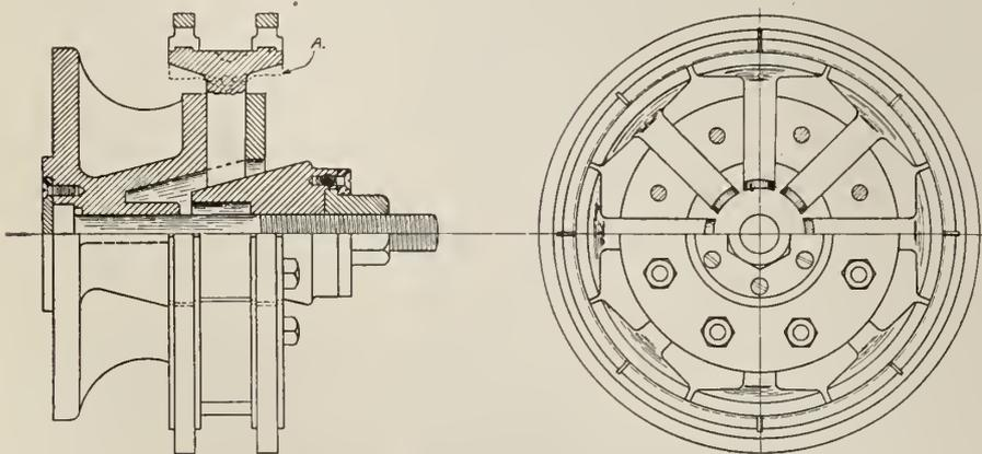
FIG. 4. IMPROVED DESIGN OF EXPANDING CHUCK.
