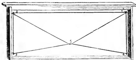
The method of wiring by means of wire nails driven through side bars of frame and bent to form a hook will be readily understood from sketch.
