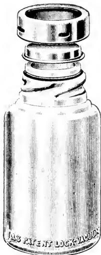
is placed on this ring, the top part—fitted with a patent screw—is put on the top and then given a half turn; this pressing the cap on to rubber ring makes the bottle absolutely air and water tight. The jar also answers splendidly for fruit preserving, and the caps, being made of very hard metal, can be used over and over again without damage. This gives them a great advantage over the ordinary screw cap, which cannot generally be used a second time."
