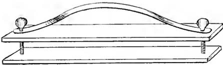
at our smith's, as shown in sketch, to clamp six frames together, which they do to perfection, providing they have shoulders or pins to keep them apart, holding the frames as firm and rigid as if they were one piece. The thumbscrews
