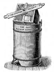
The principle upon which their merit consists is an onter cage of sheet-metal upon which are fastened strips of metal edgeways to form a rest for the wire mesh necessary for the honey-comb to rest upon. These strips edgeways offer no resistance to outflow of honey, at the same time do not allow of the wire hulging, although the wire-netting used is finer than that used in the old form of extractor.
