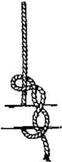
Used in hauling timber. Pass the end of the rope around the timber. Then lead it around its standing part and bring it back to make two or more turns on its own part. The strain will hold it securely.
