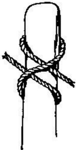
Used to fasten one pole to another in fitting up scaffolding; this knot holds snugly; is not liable to slip laterally. Hold the standing part in left hand, then pass the rope around the pole; cross the standing part, making a second turn around the pole, and pass the end under the last turn.
