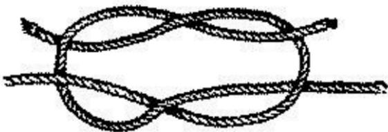
If the ends are not crossed correctly when making the reef knot, the false reef or granny is the result. This knot is always bad.
