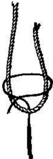
For joining a cord to a rope. May be easily made from diagram.
