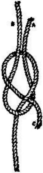
This knot is used in bending the sheet to the clew of a sail and in tying two rope-ends together.
