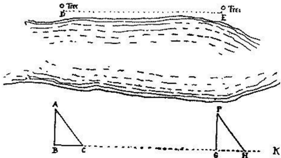
To measure the space between two distant objects, D and E. Line A B on one, then move this right-angled triangle until F G is lined on the other, with B G in line with G H. B G
