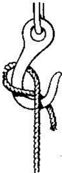
Used to secure a rope to a hook. The standing part when hauled tight holds the end firmly.
