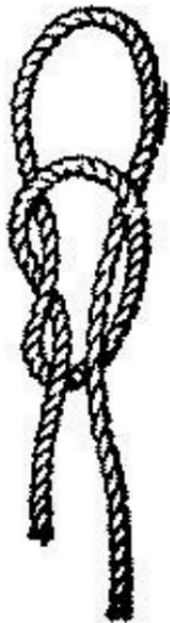
A bight is first formed and an overhand knot made with the end around the standing part.
