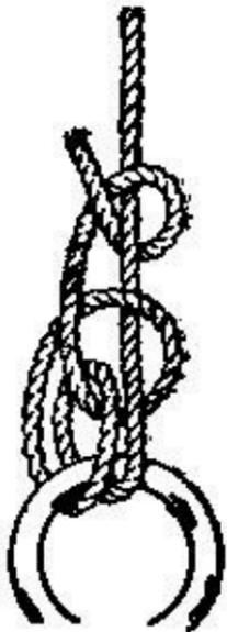
Used aboard yachts for bending on the gaff topsail halliards. It consists of two turns around a spar or ring, then a half hitch around the standing part and through the turns on the spar, and another half hitch above it around the standing part.
