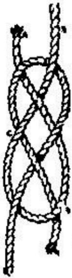
Used in uniting hawsers for towing. Is easily untied by pushing the loops inwards.
