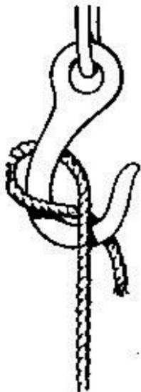
Used to secure a rope to a hook. The standing part when hauled tight holds the end firmly.
