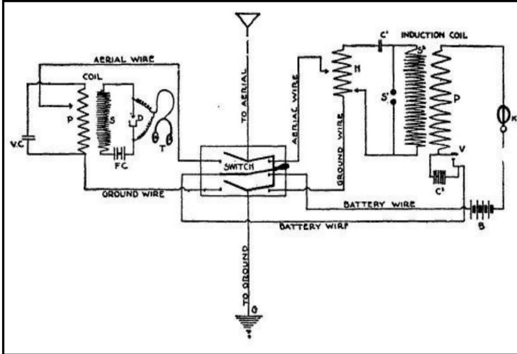
The first thing to do is to build an aerial. First find out how long your location will allow you to build it, and how high. It ought to be at least 50 to 60 feet high and about 70 to 100 feet long. The main point in building an aerial is to have it {211} well insulated from the ground, and all connections in wire perfectly solid. It is advisable to solder every connection and to make your aerial strong as it has a great deal to do with the working qualities of the station.
