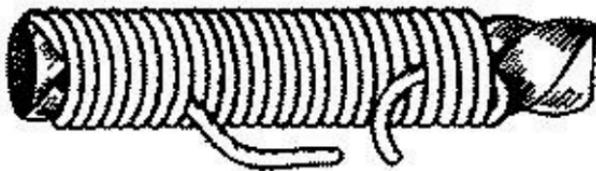
Lay the end of a piece of twine along the end of the rope. {49} Hold it to the rope with the thumb of your left hand while you wind the standing part around it and the rope until the end of the twine has been covered. Then with the other end of the twine lay a loop back on the end of the rope and continue winding the twine upon this second end until all is taken up. The end is then pulled back tight and cut off close to the rope.
