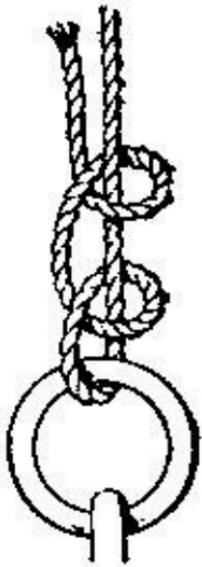
Useful because they are easily made and will not slip under any strain. Their formation is sufficiently indicated by the diagram.
