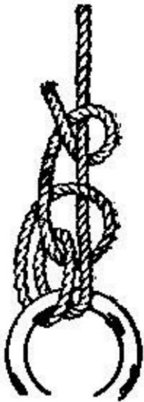
Used aboard yachts for bending on the gaff topsail halliards. It consists of two turns around a spar or ring, then a half hitch around the standing part and through the turns on the spar, and another half hitch above it around the standing part.
