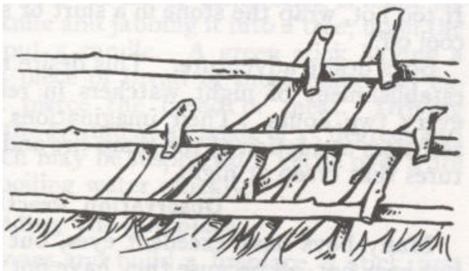
Fig. 2. Method of thatching
