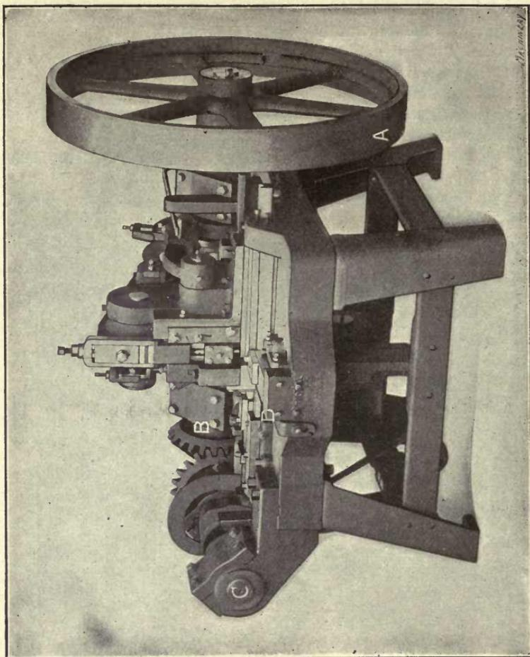
Fig. 39. "National" Hot-forged Nut Machine used exclusively for the Manufacture of Square Nuts from Rectangular Bar Stock
