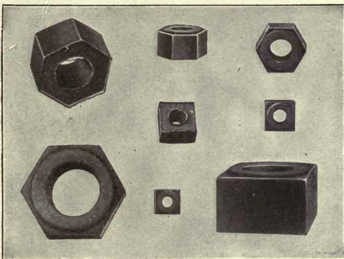
Fig. 38. Group of Square and Hexagon Nuts, showing Character of Work turned out in Hot-pressed Nut Machines
