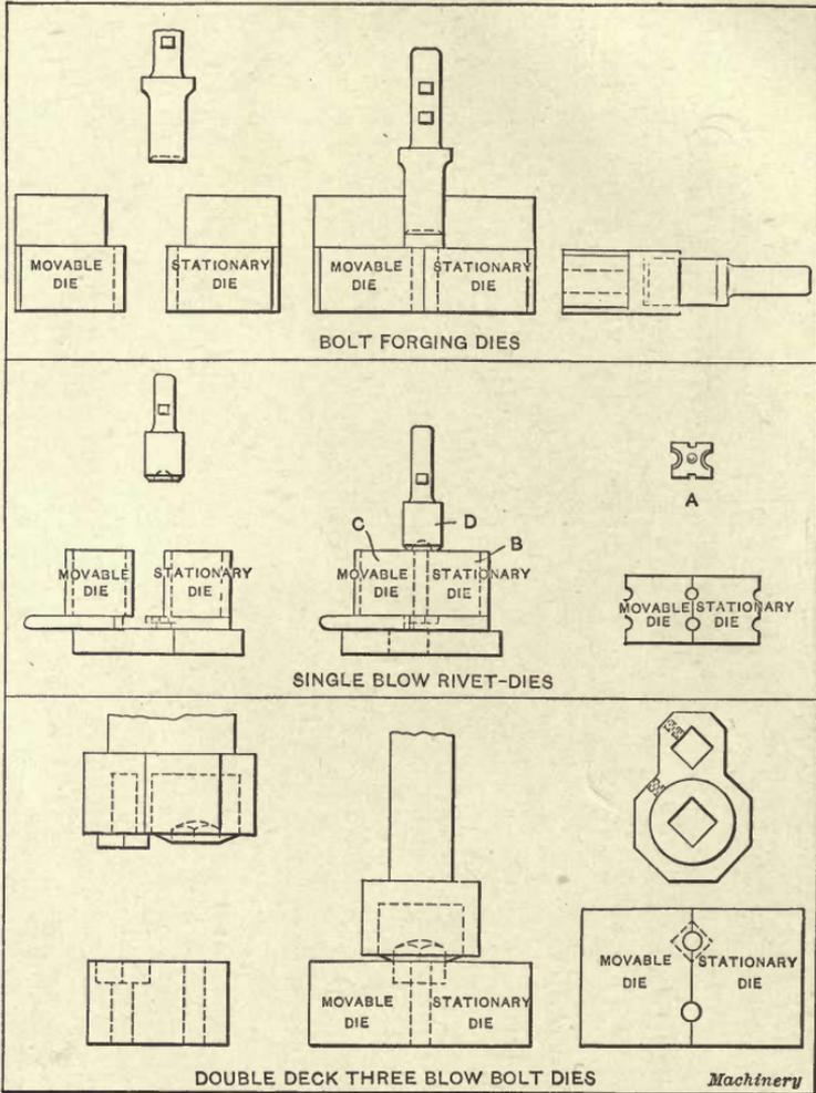
Fig. 3. Plain Type of Bolt Forging Dies of Universal Application.
