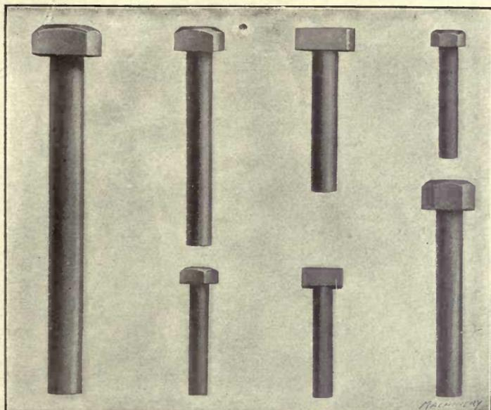
Fig. 23. Some Examples of Work produced in National Hammer Headers
