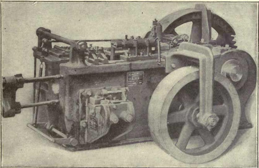
Fig. 2. Ajax Bolt Heading Machine suitable for all Types of Machine Bolts and Upset Forgings
