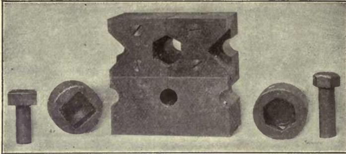
Fig. 12. Combination Square and Hexagon Double-deck Bolt Dies
