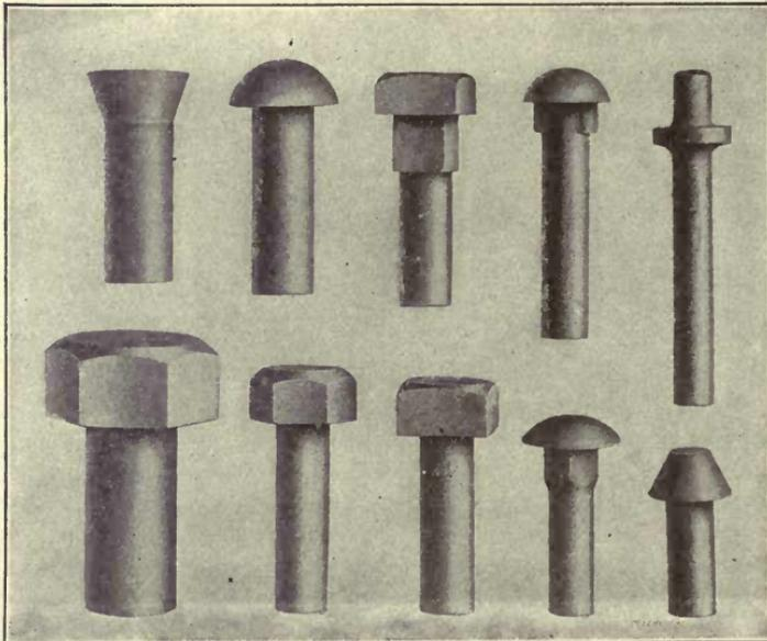
Fig. 13. Some Examples of Work turned out on National Wedge-grip Bolt and Rivet Header
