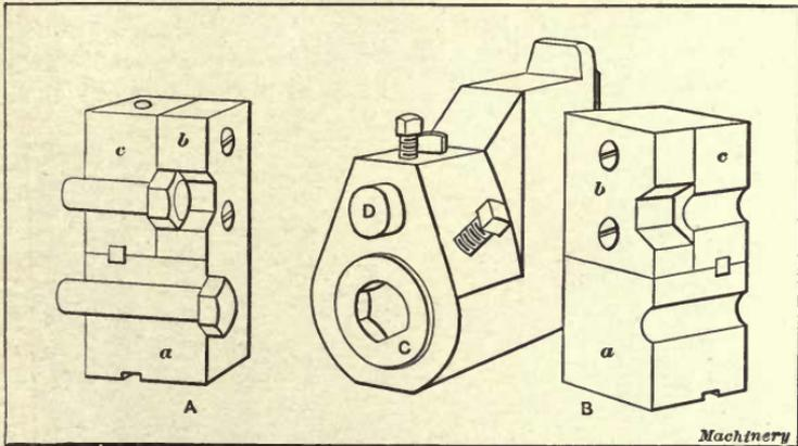
Fig. 11. Type of Double-deck Dies used in producing Bolt Heads without Fins or Burrs in Three Blows
