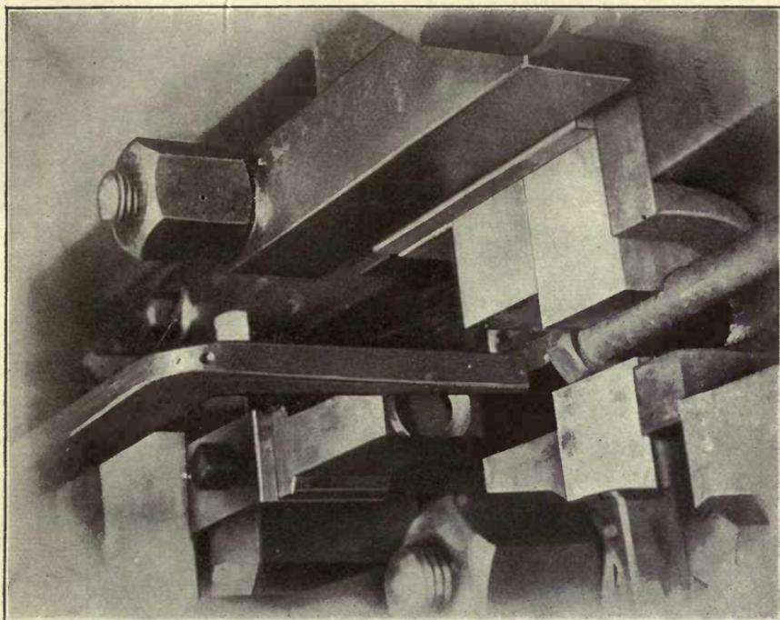
Fig. 7. Second Step in the Production of Bolt Heads
