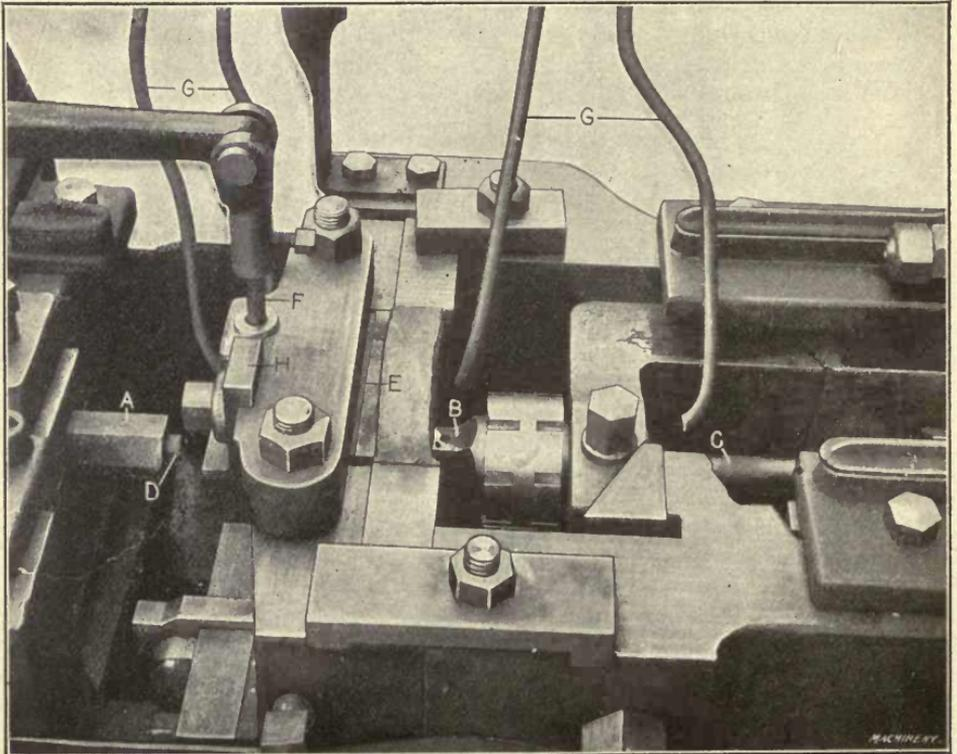
Fig. 35. Detail View of Machine shown in Fig. 34 showing Dies, Punching, Piercing, Crowning Tools, etc.
