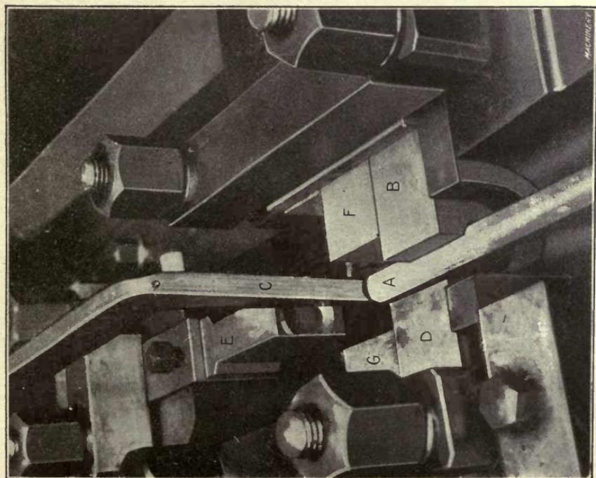
Fig. 6. First Step in the Production of Bolt Heads in Plain Forging
