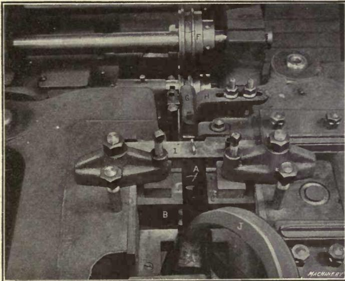
Fig. 23. View looking down into Die Space of Ajax Continuous-motion Bolt and Rivet Header
