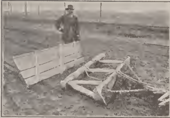
Drag with Platform Removed
