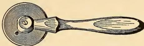
FIG. 32. — Comb-foundation cutter.
