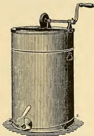
FIG. 121. — Extractor with stationary can.
