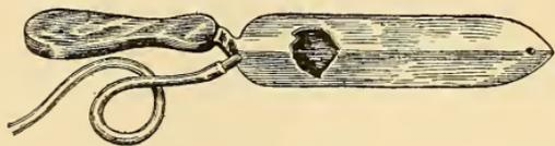
FIG. 117. — Steam-heated uncapping knife.
