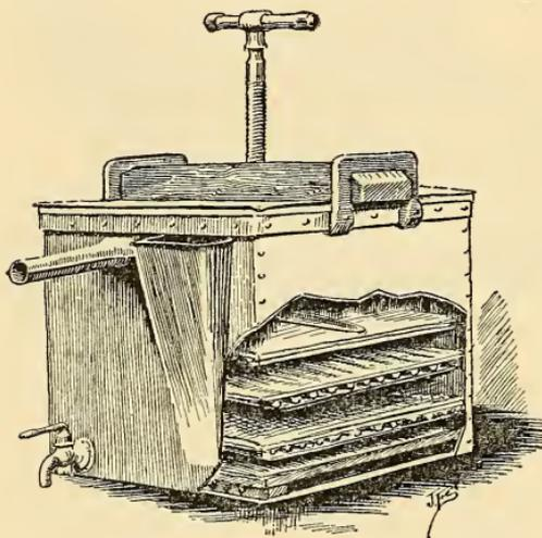
FIG. 140. — Hot water (Hershiser) wax press.
