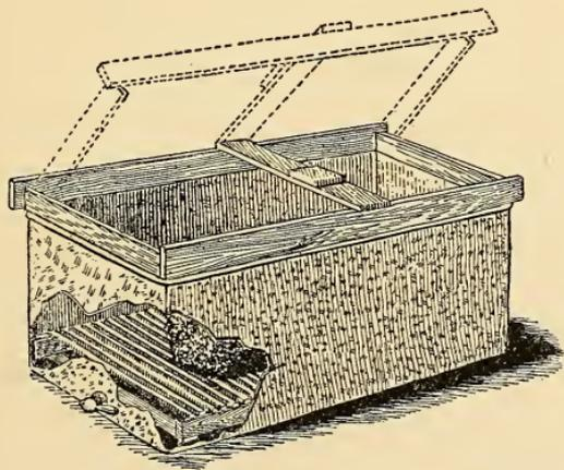
FIG. 120. — Tank to receive cappings.
