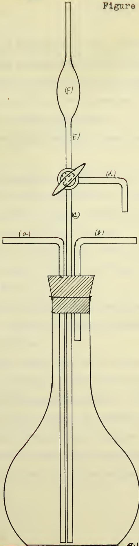
cock it may be run off through tube (d). When it is desired to aerate the solution with purified air, compressed air is blown through a series of wash bottles and attached to tube (a) containing in order, - cotton, sterile water, sulphuric acid, and a weak solution of sodium hydroxide.
