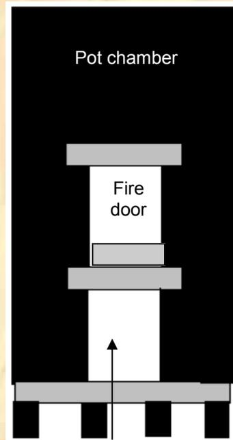
Entry for clearing out post firing debris
