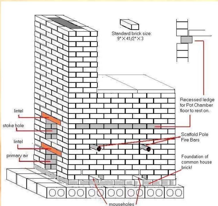
This is a drawing of the brick chimney'd kiln as it evolved before the perforated floor version; useful for brick counting and with some detail notes as well.
