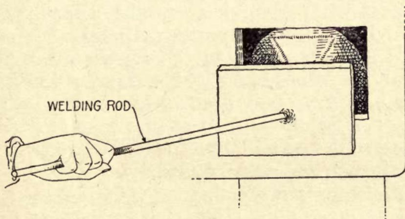
FIG. 25.—Welding rod tacked to jacket.
