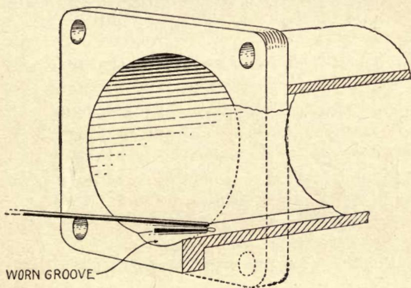
FIG. 26.—Welding scored cylinder—position of flame.
