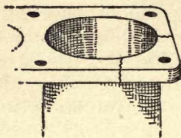
FIG. 19.—Broken cylinder lug.
