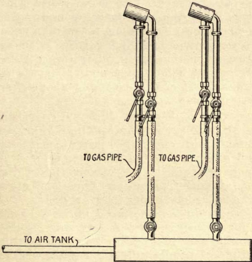
FIG. 7.—Gas preheating torches, with manifold for air.
