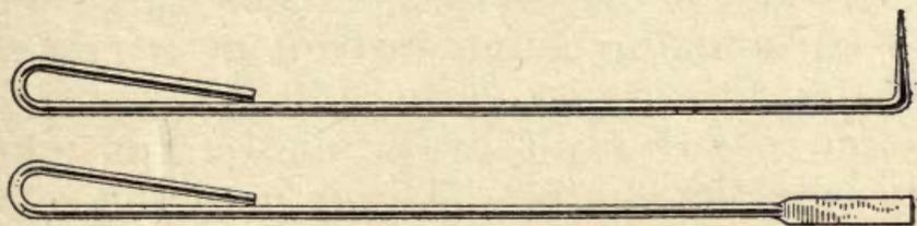
FIG. 30.—Rods for puddling aluminum.
