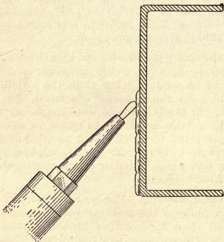
FIG. 49.—Beginning the frame weld—flame directed upwards.
