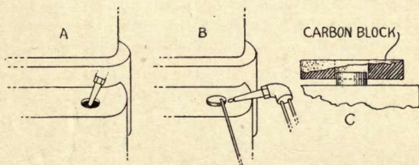
FIG. 29.—Making new boss for valve guides.
