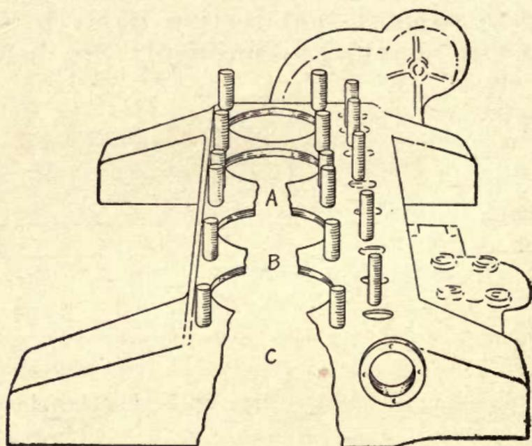
FIG. 40.—Direction of welding—toward unbonded section.
