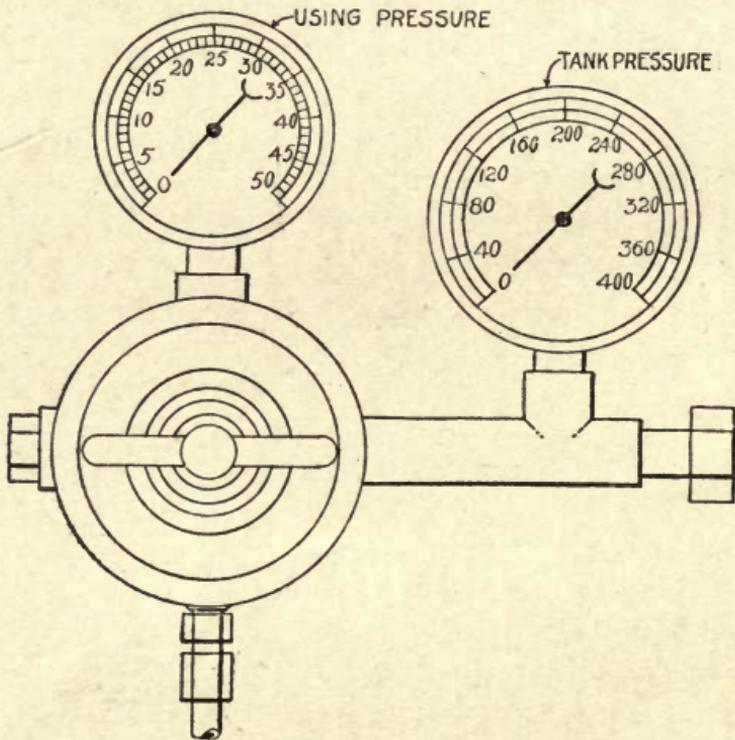
FIG. 5.—Regulators should have two gauges.
