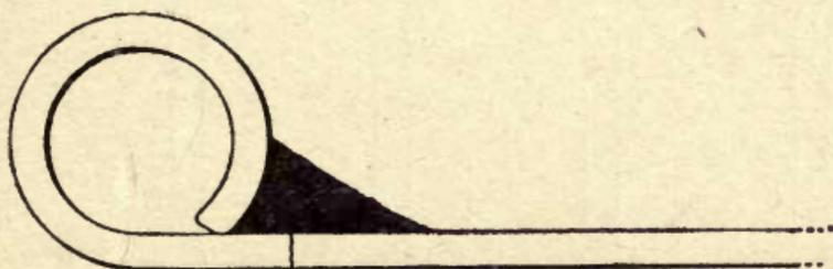
FIG. 60.—A spring weld at this point will usually hold.
