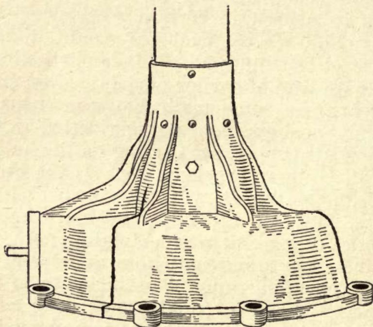
FIG. 62.—Break in malleable rear housing.
