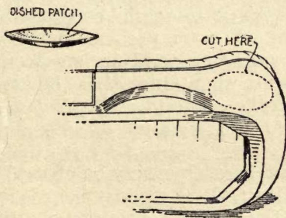
FIG. 43.—Preparation for body welding.
