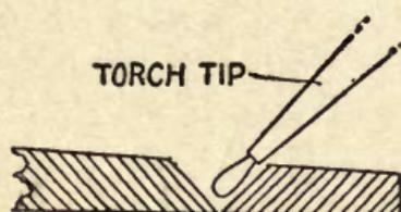
FIG. 16.—Flame directed toward heavier section.
