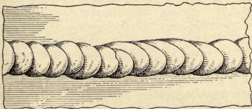
FIG. 31.—Appearance of flux weld.
