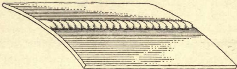
FIG. 46.—Proper appearance of steel weld.
