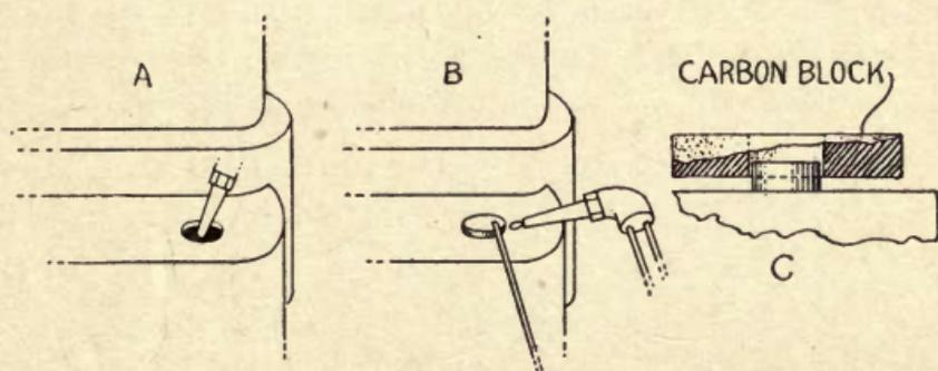
FIG. 29.—Making new boss for valve guides.
