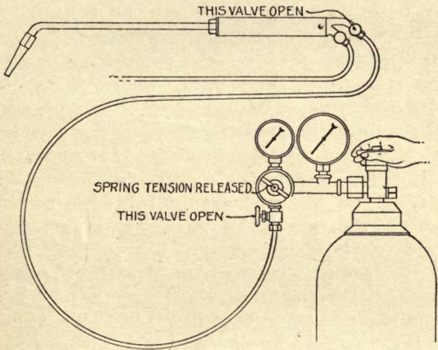
FIG. 9.—Turn on the oxygen carefully.
