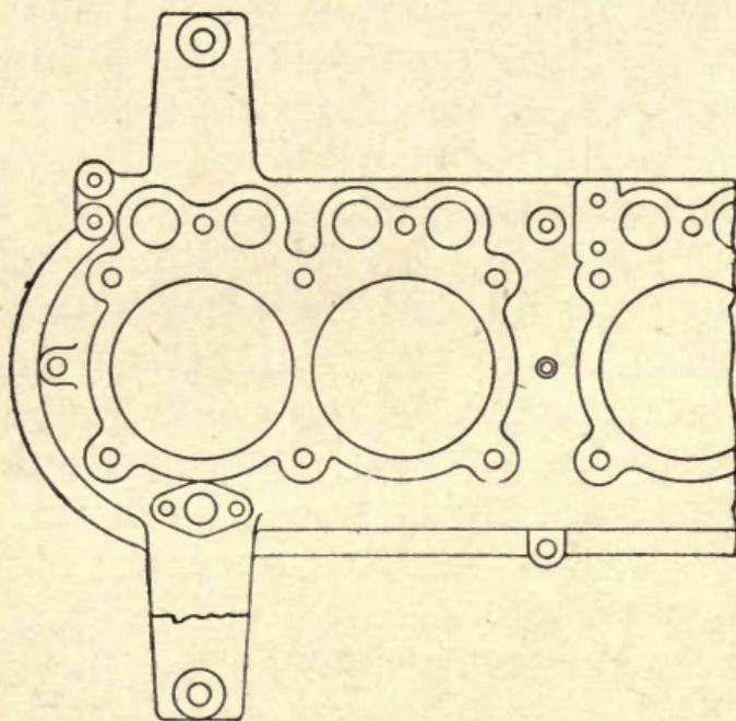
FIG. 33.—Break in arm of case.
