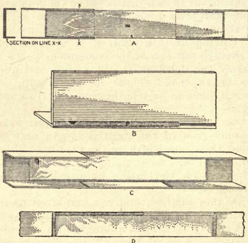
FIG. 52.—Method of lengthening frame.
