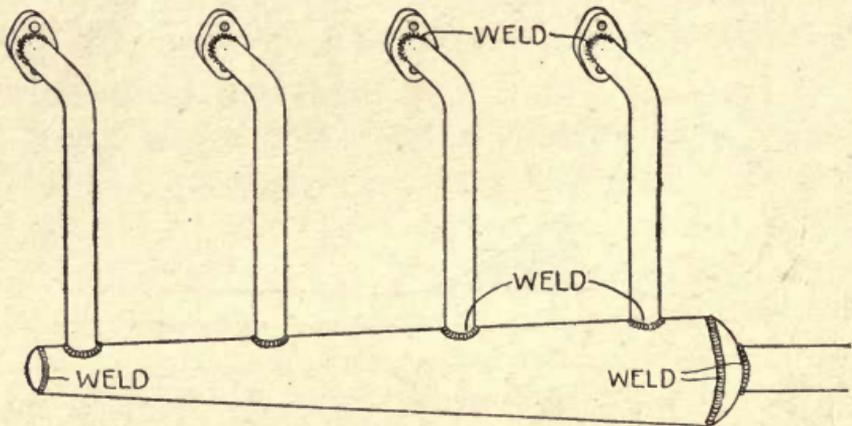
FIG. 61.—Exhaust constructed by welding.
