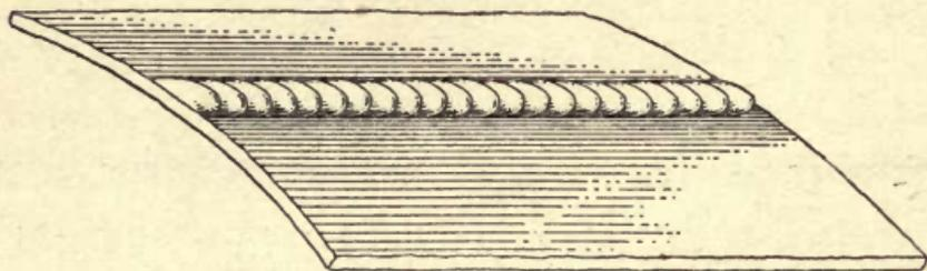
FIG. 46.—Proper appearance of steel weld.
