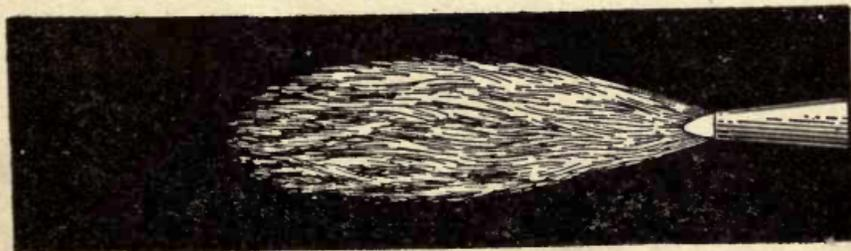
FIG. 13.—Oxidizing flame—ruinous to good welding.
