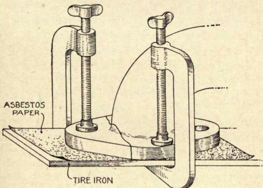
FIG. 32.—Set up of aluminum manifold.
