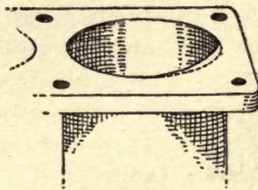
FIG. 20.—Bore warped as shown.
