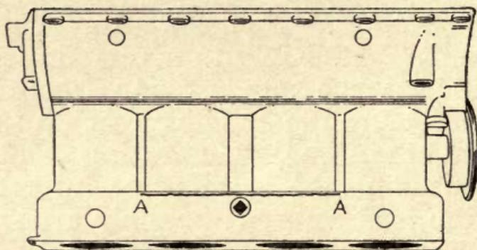
FIG. 23.—Water jacket break in four-cylinder casting.
