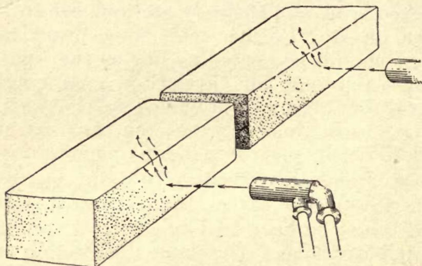
FIG. 38.—Indirect heating with gas torches.
