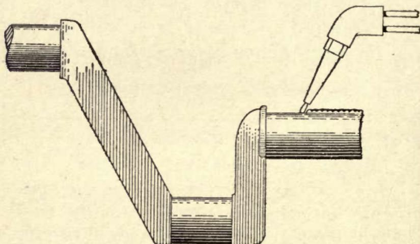
FIG. 54.—Building up journal of crank shaft.
