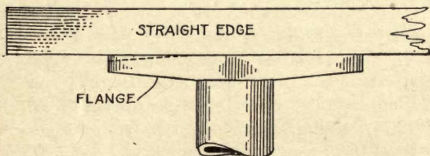
FIG. 18.—Testing for alignment.
