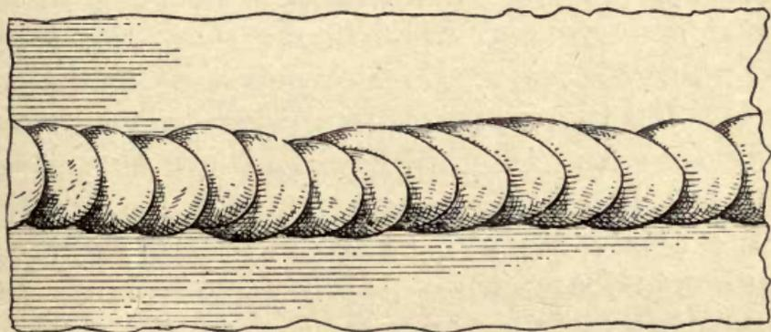
FIG. 31.—Appearance of flux weld.
