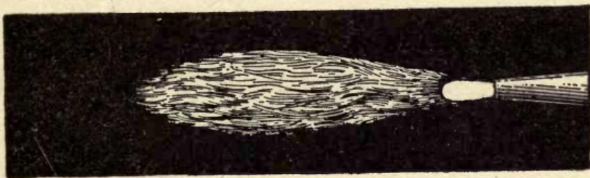
FIG. 12.—Neutral flame—proper proportions of both gases.
