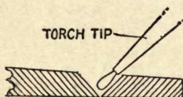
FIG. 16.—Flame directed toward heavier section.
