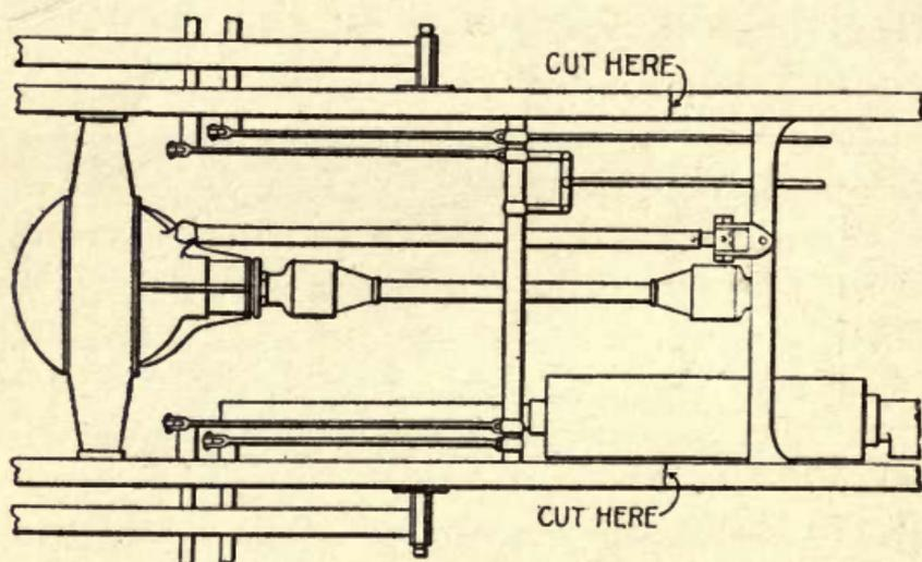
FIG. 51.—Where to cut the frame for lengthening.
