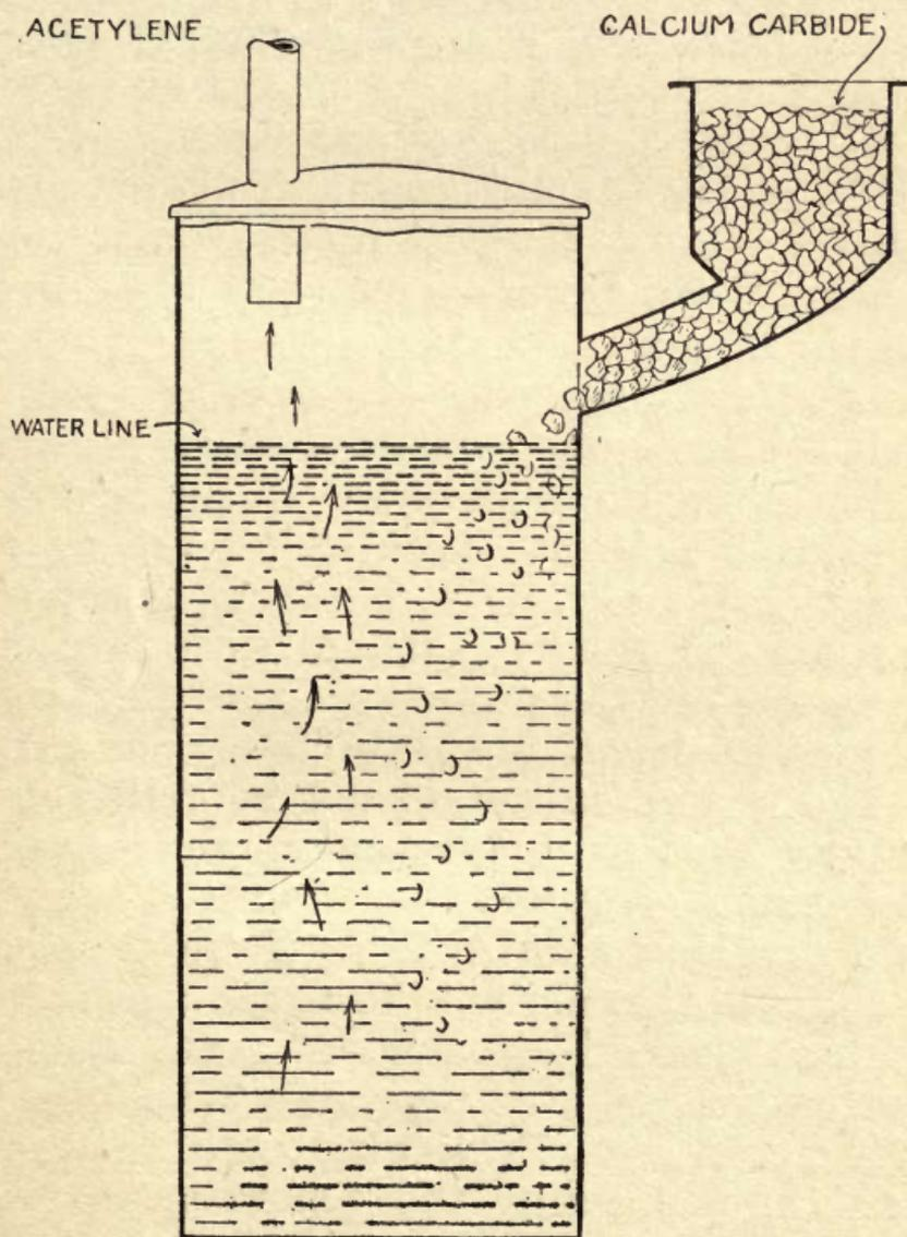
FIG. 2.—Principle of acetylene generation—carbide to water.
