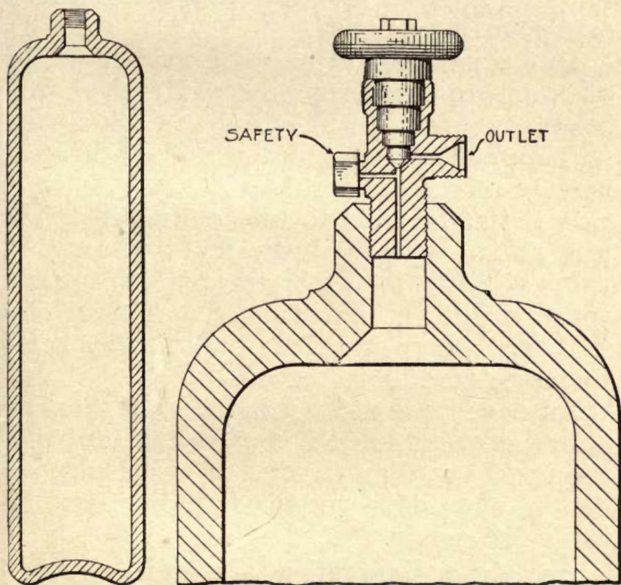
FIG. 1.—Oxygen cylinder and valve.
