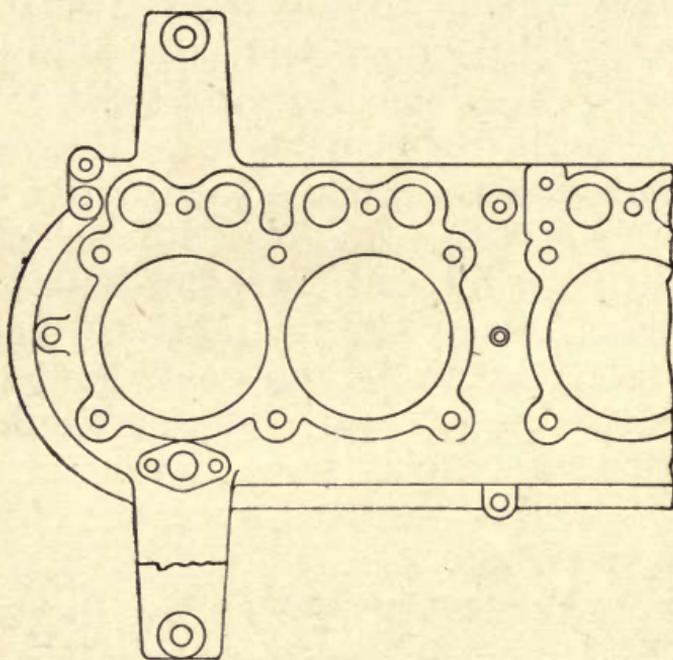
FIG. 33.—Break in arm of case.
