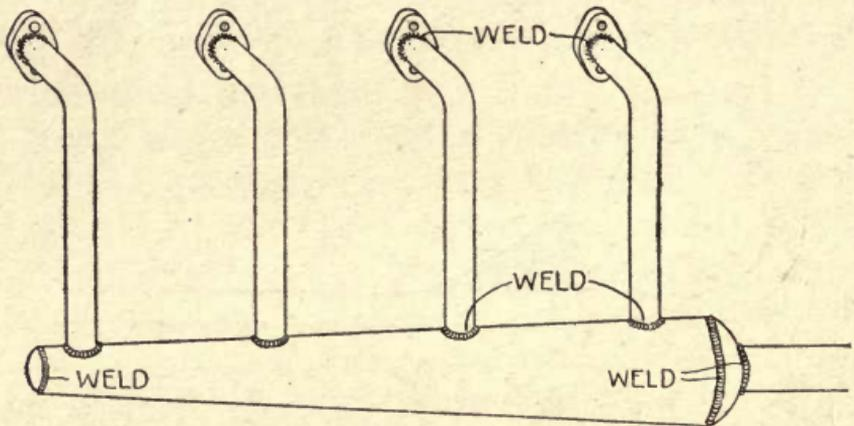
FIG. 61.—Exhaust constructed by welding.
