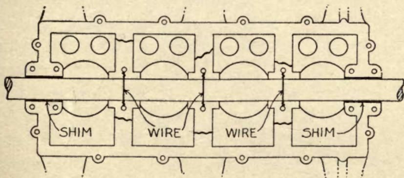
FIG. 39.—Use of shaft to line up broken bearings.
