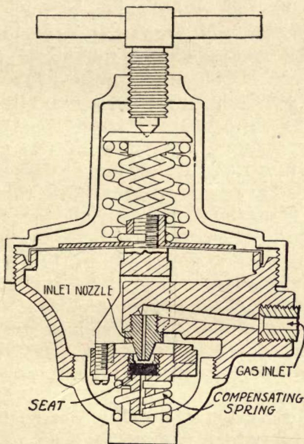
FIG. 4.—Section of diaphragm regulator.
