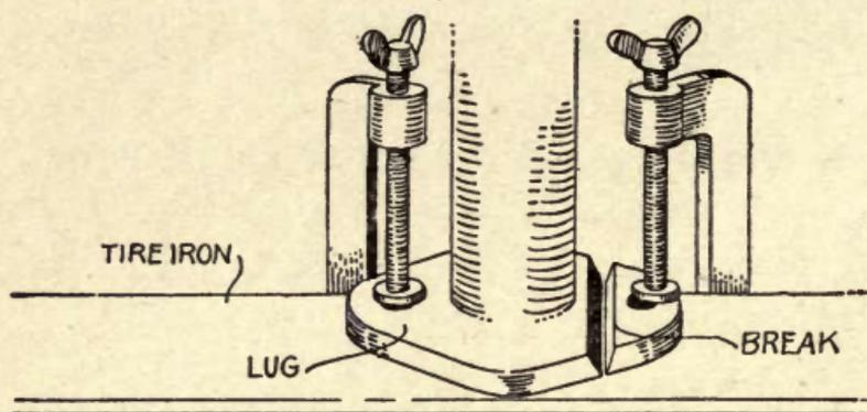
FIG. 15.—Set up of exhaust manifold.
