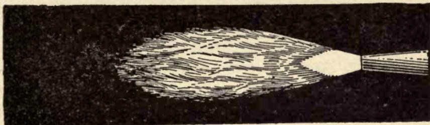
FIG. 11.—Carbonizing flame—not enough oxygen.
