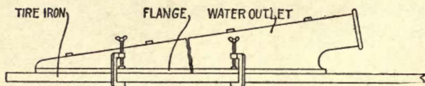
FIG. 21.—Water outlet set up for welding.
