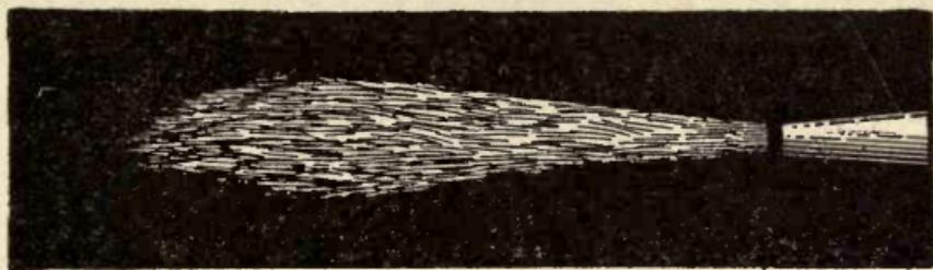
FIG. 10.—Acetylene blowing away from tip.
