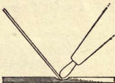
ROD IN CONTACT WHILE PORTION IS MELTED OFF.
