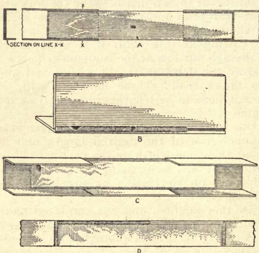
FIG. 52.—Method of lengthening frame.
