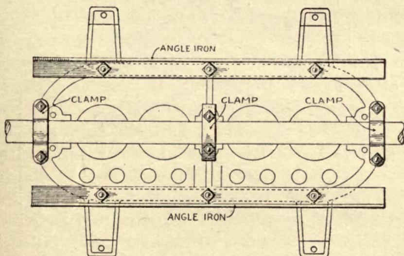
FIG. 35.—Wrong method of setting up case.
