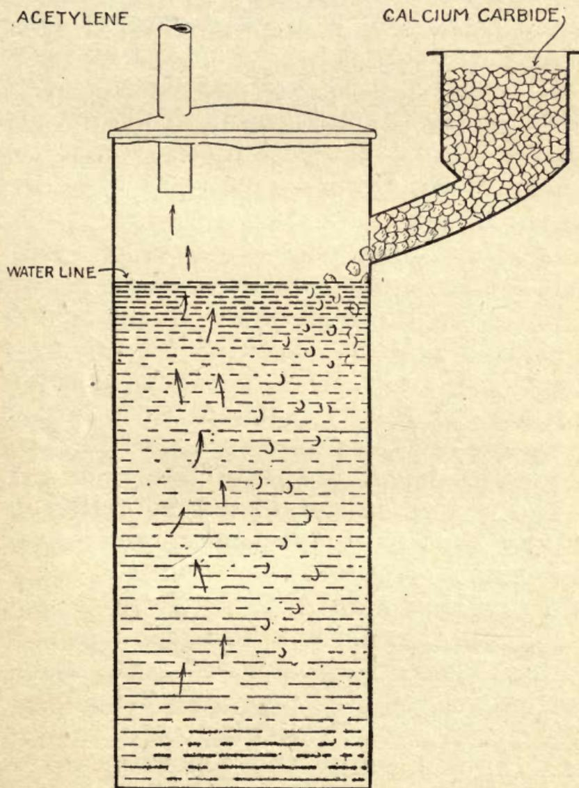
FIG. 2.—Principle of acetylene generation—carbide to water.
