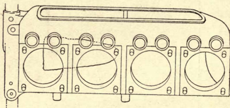
FIG. 27.—Cast iron crank case with steel patch.
