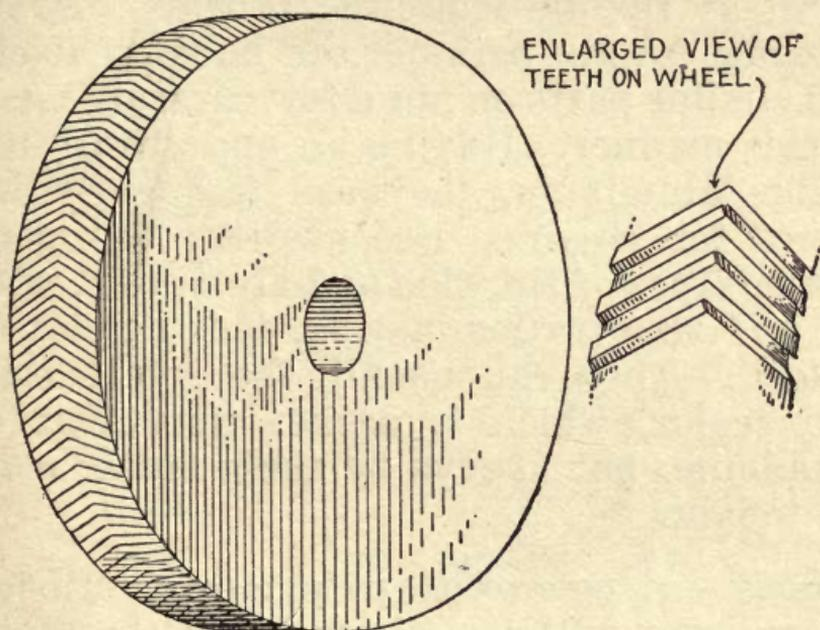
FIG. 42.—Finishing wheel for aluminum.
