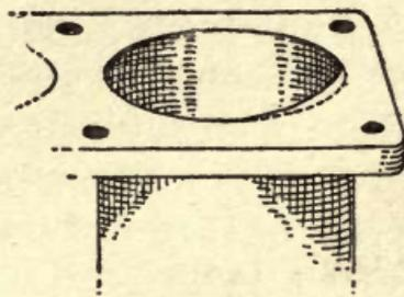
FIG. 20.—Bore warped as shown.
