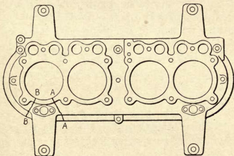
FIG. 34.—Arm broken into body of case.
