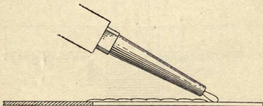
FIG. 56.—Position of torch for sheet metal welding.
