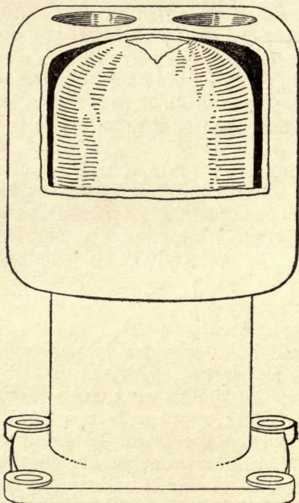
FIG. 24.—Break in compression head.
