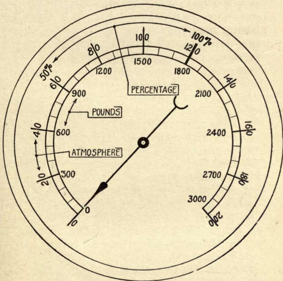
FIG. 6.—High pressure oxygen gauge dial.
