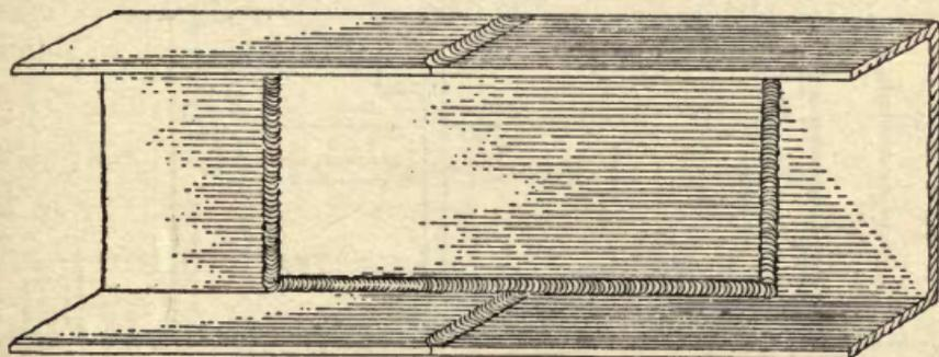
FIG. 50.—Reinforcing inside of frame with welded plate.
