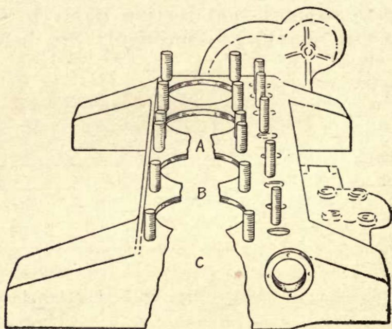
FIG. 40.—Direction of welding—toward unbonded section.
