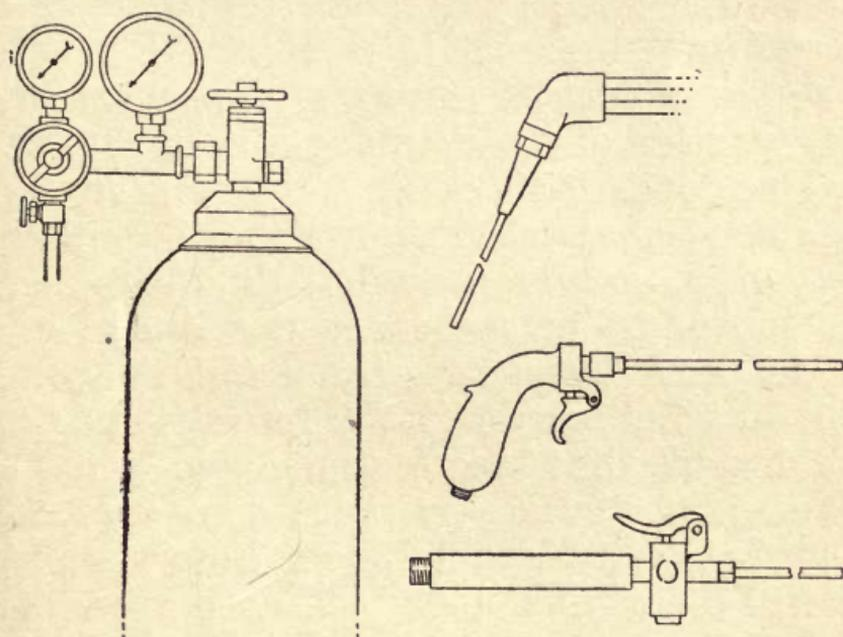
FIG. 65.—Oxygen carbon burning apparatus, with different types of burners.
