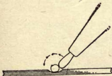
FLAME TOUCHES EACH PART OF METAL IN MELTING NEW MATERIAL WITH OLD.
