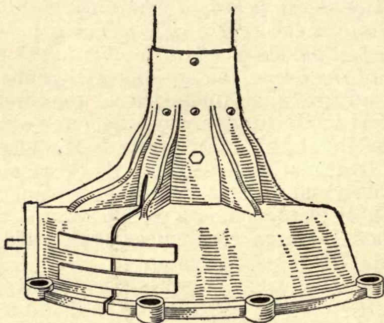
FIG. 63.—Housing reinforced with wrought iron straps.
