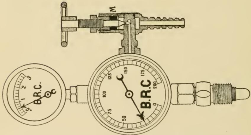
These gases, to be used in the blow-pipe, must therefore be brought to a lower pressure; this result is attained by the use of regulating valves mounted on the tanks. In the actual work these regulating valves are used in conjunction with
