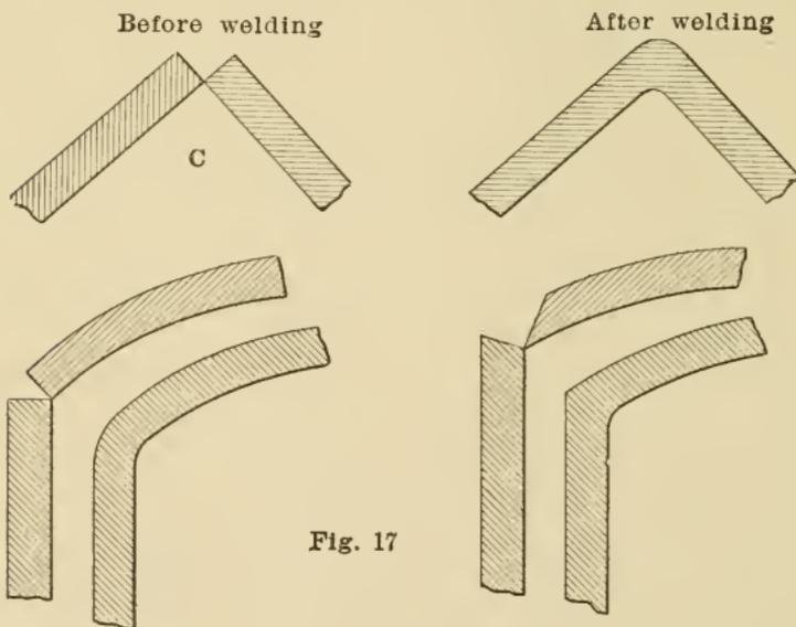
In general, in preparing plates to be assembled by oxacetylene welding care should be taken not to imitate shapes previously requiring bolting or riveting.
