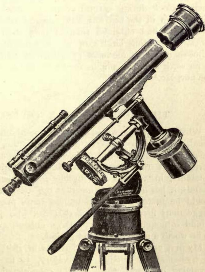
**Fig. 317.—3-inch Portable Equatorial Telescope.**
