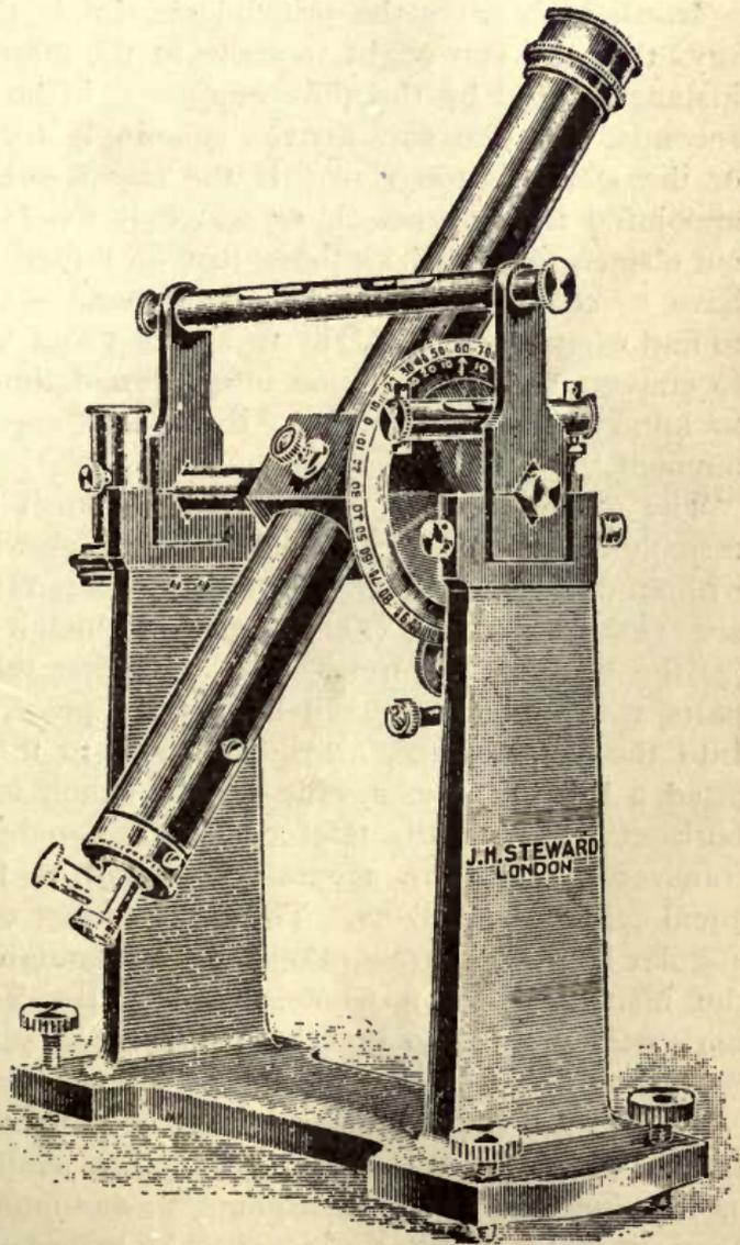
Fig. 349.—The Transit Instrument for obtaining the time.
