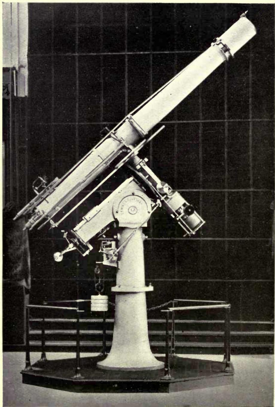
Equatorial Telescope, with Object-glass of 10 inches aperture (*Cooke*).
