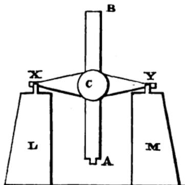
may be explained by help of fig. 7. An ordinary telescope, *AB*, is fixed to an axis at right angles to the telescope. The shape of the axis and the method of attachment of the telescope thereto, are specially designed so as to secure as much rigidity as possible. At the extremities of the axis are pivots,
