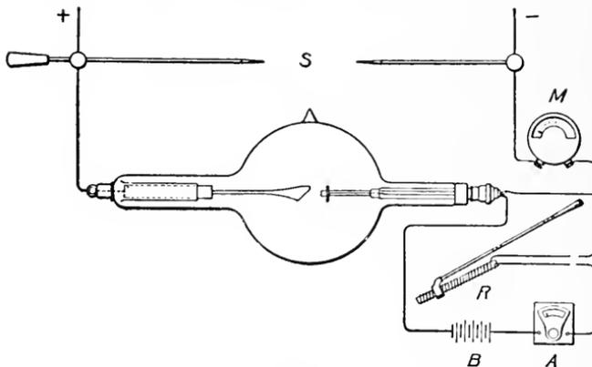
FIG. 128A.—DIAGRAM SHOWING WIRING CIRCUIT OF COOLIDGE TUBE.
