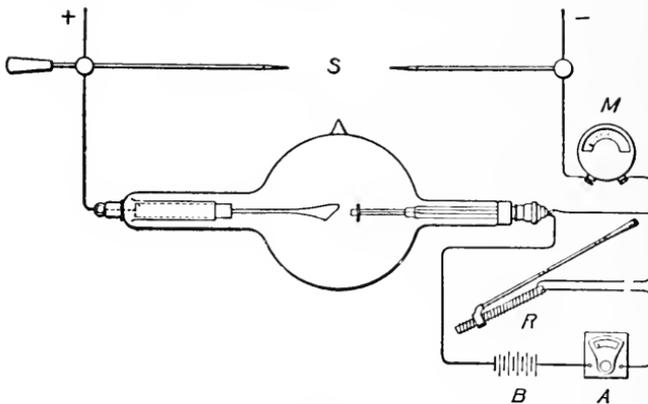
FIG. 128A.—DIAGRAM SHOWING WIRING CIRCUIT OF COOLIDGE TUBE.
