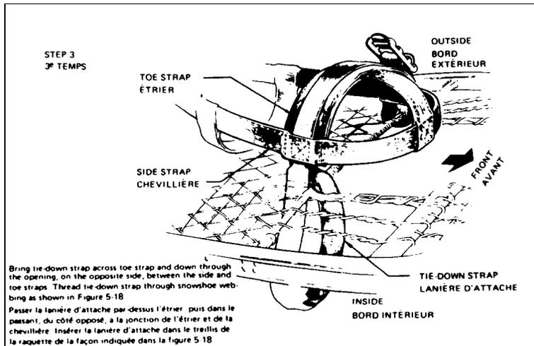
Figure 5-20 Attaching Harness to Snowshoe Step 3
