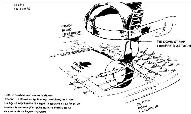
Figure 5-18 Attaching Harness to Snowshoe Step 1
