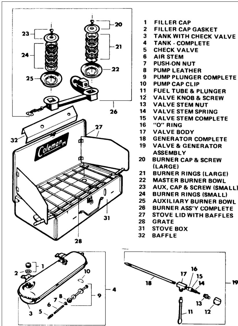
Figure 2-8C Stove Coleman Model 431 Two Burner
