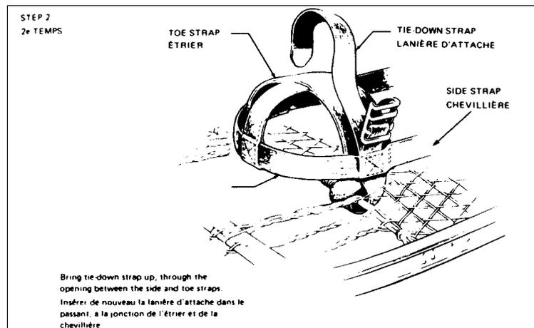
Figure 5-19 Attaching Harness to Snowshoe Step 2
