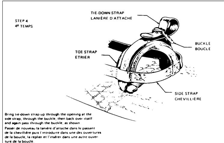
Figure 5-21 Attaching Harness to Snowshoe Step 4
