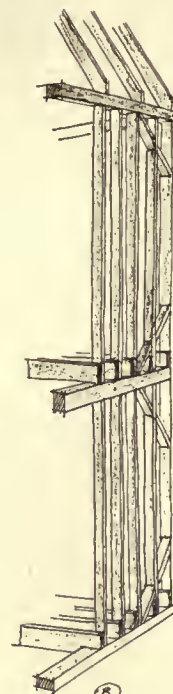
BRACED FRAME AS DEVELOPED FROM NEW ENGLAND COLONIAL
