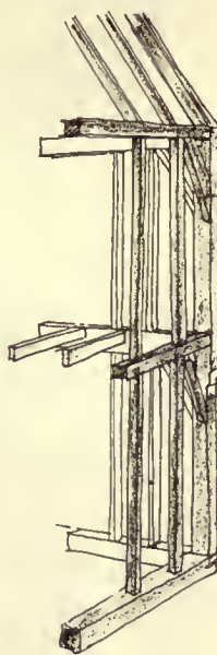
TYPE OF FRAMING FOR COLONIAL OF FIRST PERIOD
