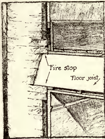
Fire stopping of furred off space in brick wall Fig 1.
