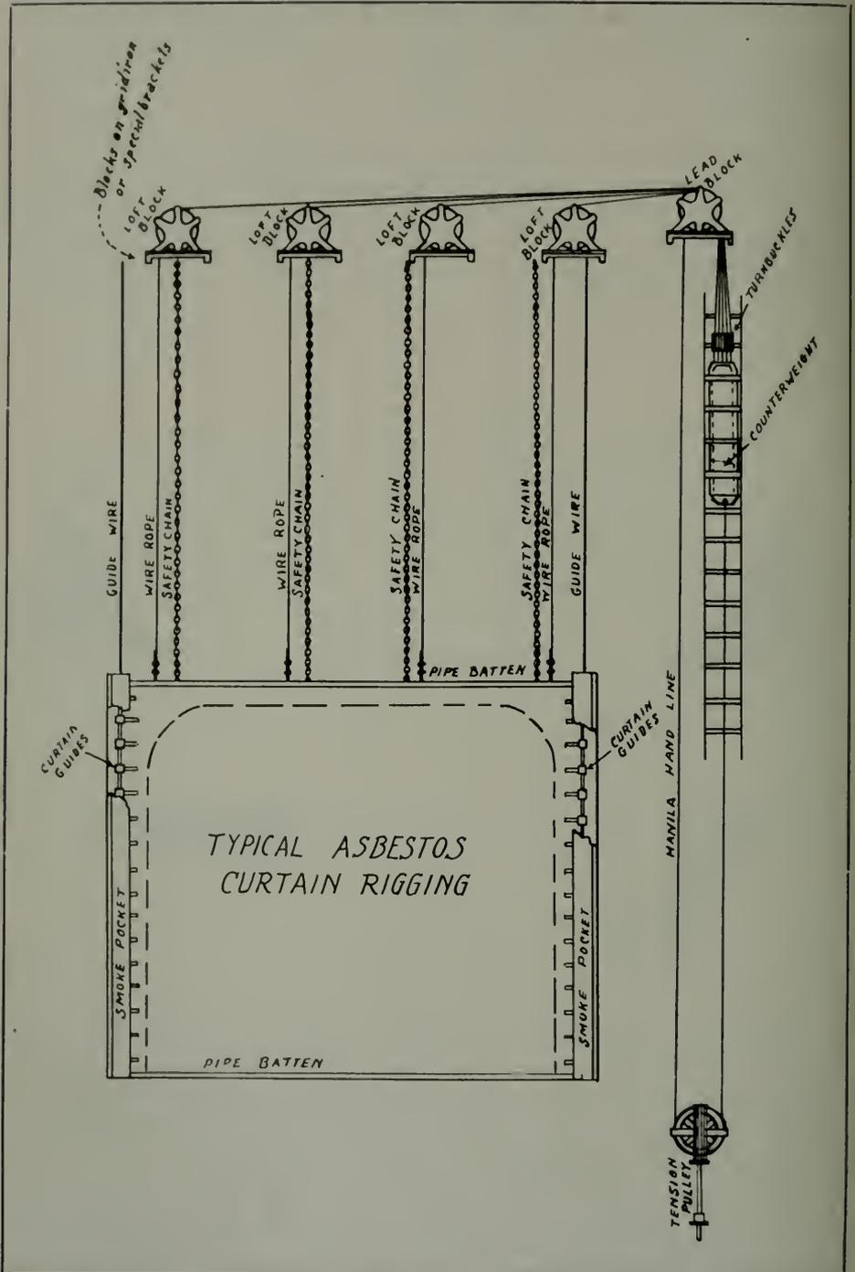
FIG. 4 TYPICAL RIGGING FOR AN ASBESTOS CURTAIN
