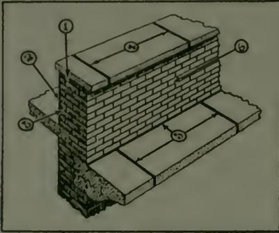
1. Water-proof Cut-Off of Dehydratine No. 6 on top of Parapet Wall under Coping.
